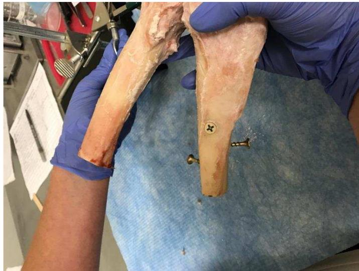
9. Drill fixture holes in femur. (NOTE: it is typically easier to drill the holes when the femur is cleaned of all soft tissue, as described in Step 5).
