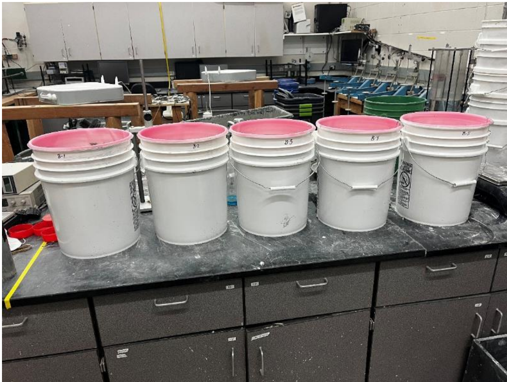
Photo 19. Desiccation buckets after initial placement and during subsequent drying
