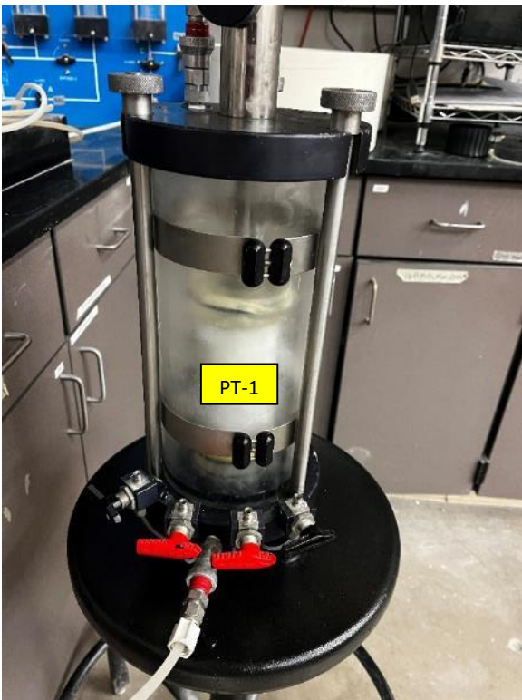
Photo 26. PT-1 as cell is filled with water
