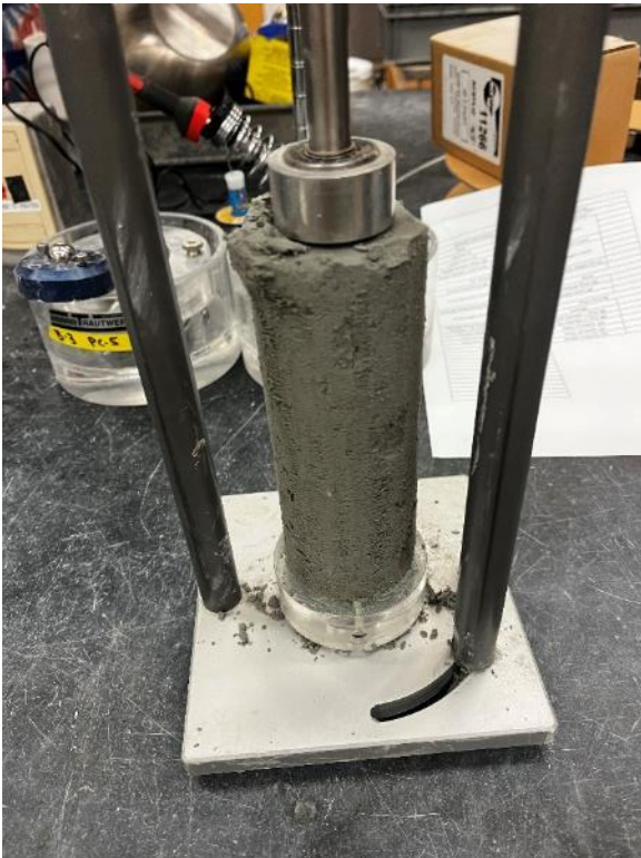
Photo 58. PT-5 sample trimming for triaxial testing
