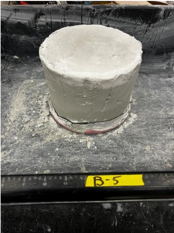
Photo 73. B-5 after removal from bucket and liner
