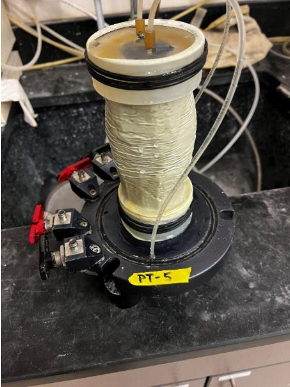
Photo 60. PT-5 post shear testing
