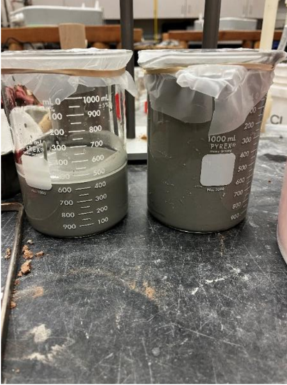
Photo 9. Zero effective stress void ratio test start
