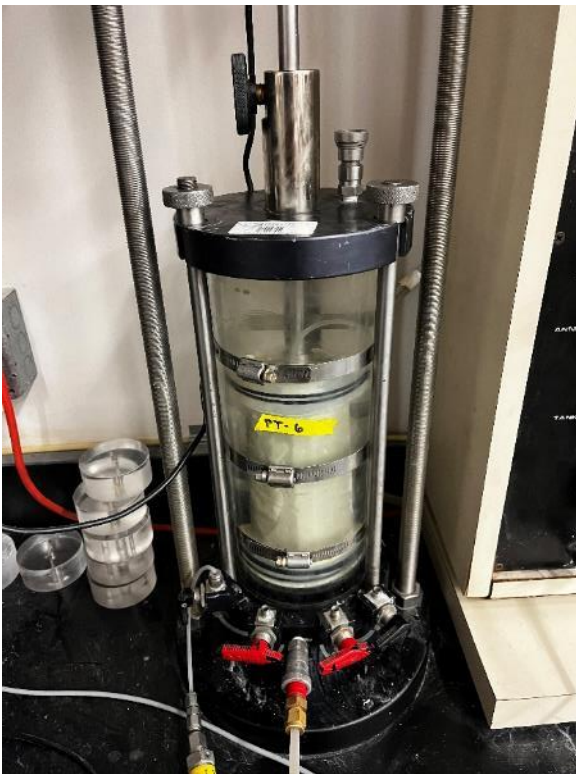
Photo 62. PT-6 during shear testing
