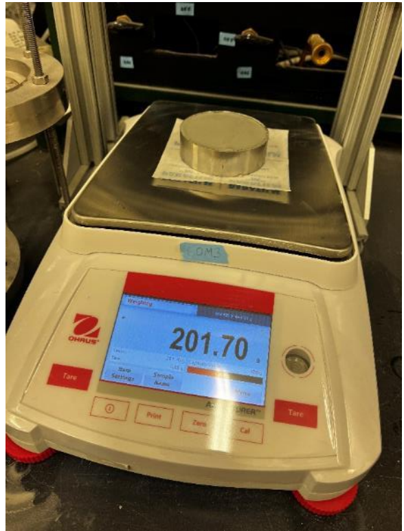
Photo 12. Shrinkage limit test sample
