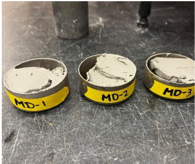
Photo 23. Moisture samples processed from B-1
