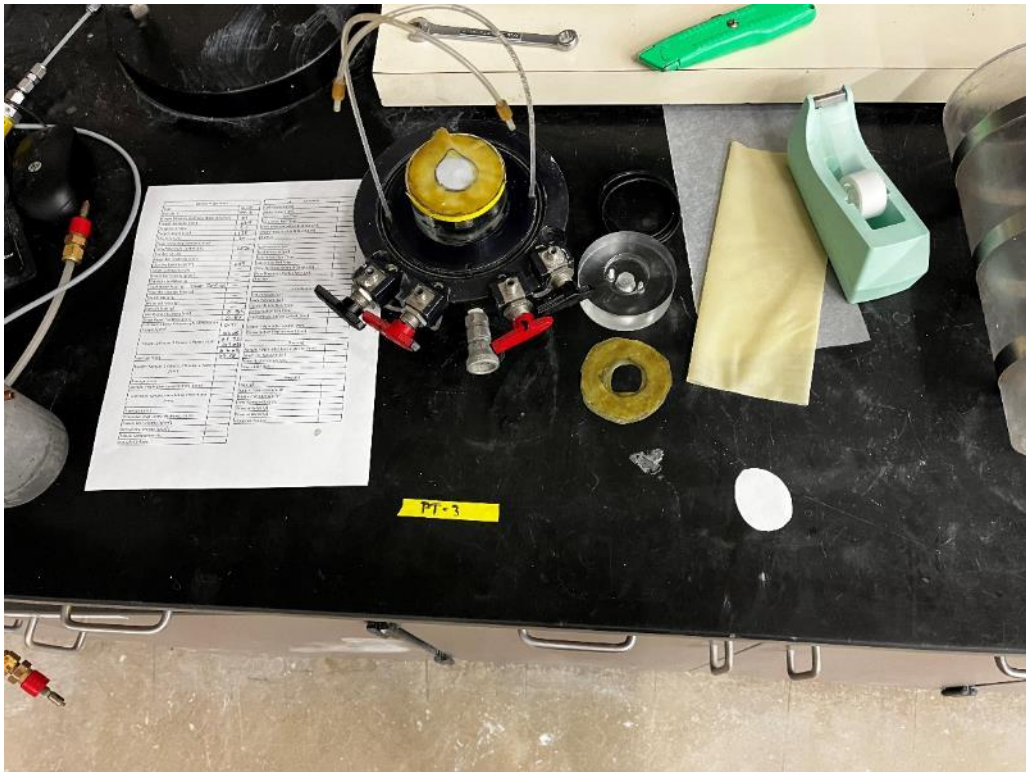
Photo 80. Typical triaxial sample set up and equipment for each desiccation bucket
