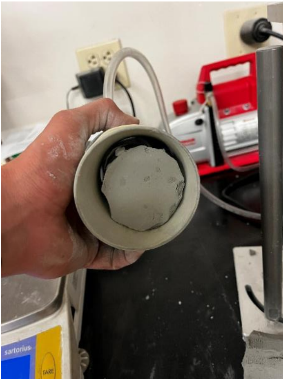
Photo 38. PT-3 oversized mold to apply membrane
