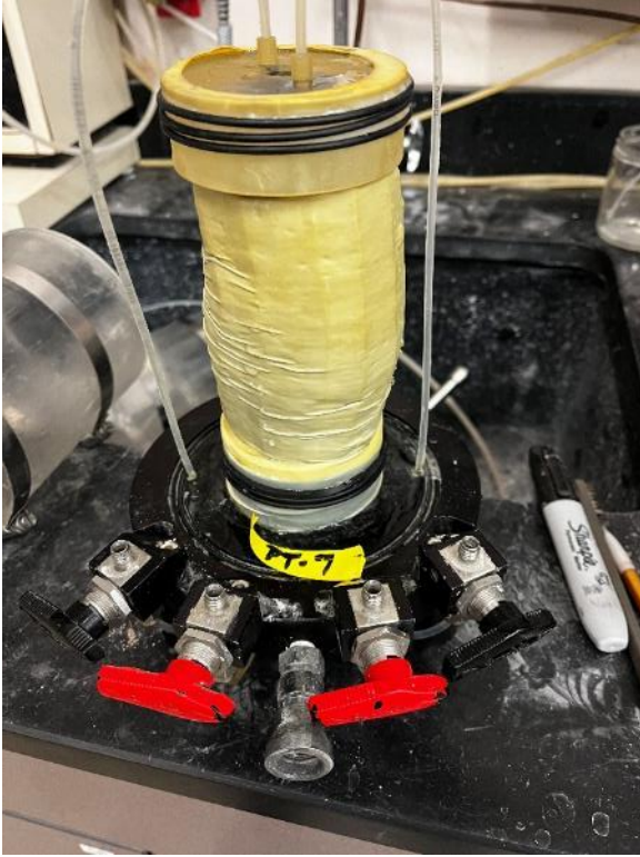
Photo 71. PT-7 post shear testing
