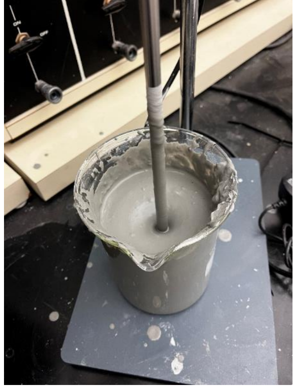
Photo 6. Mixing for mini vane shear
