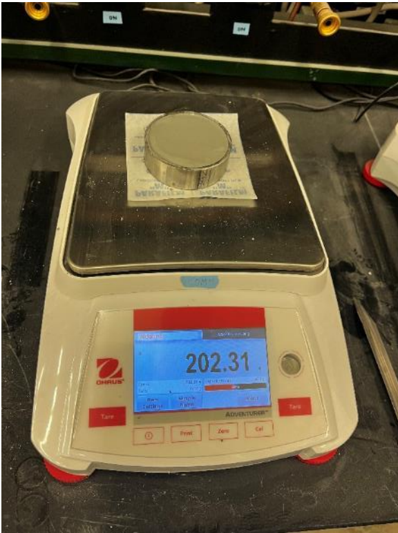
Photo 11. Shrinkage limit test sample
