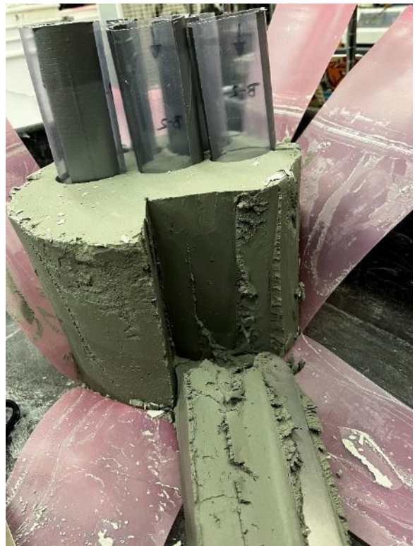
Photo 31. B-2 outer edge removed to access samples for moisture density testing
