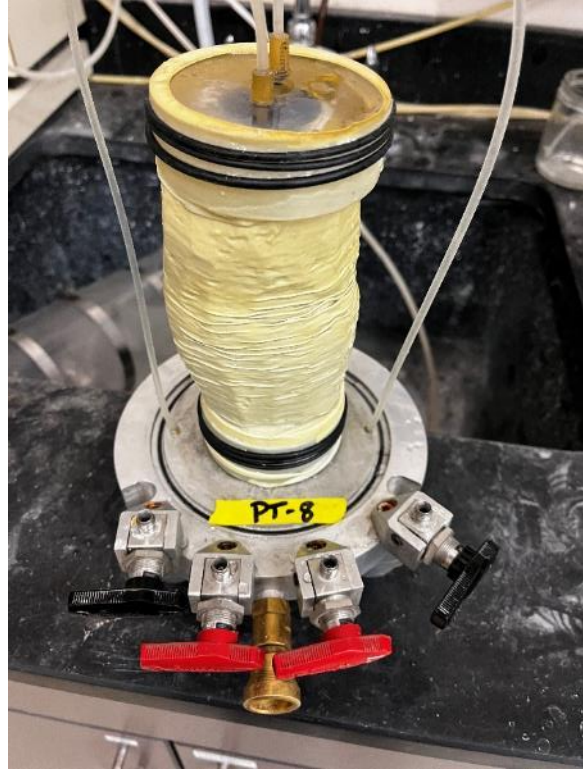
Photo 72. PT-8 post shear testing
