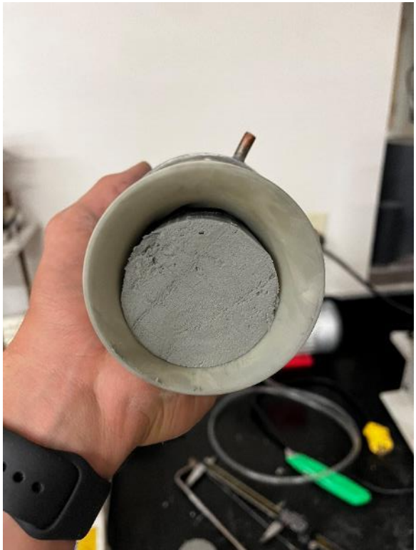
Photo 43. PT-4 suspended in membrane
