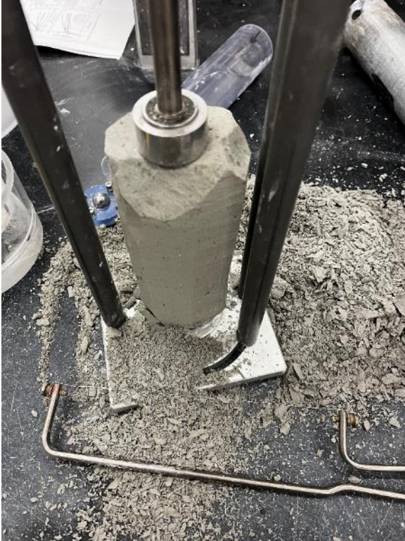
Photo 68. PT-7 during sample trimming
