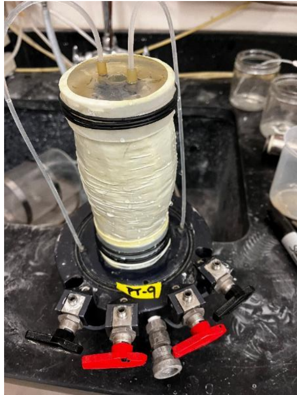
Photo 76. PT-9 post shear testing
