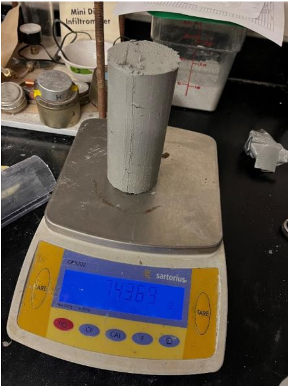
Photo 42. Weight of PT-4 prior to testing
