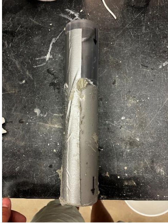
Photo 21. B-1 triaxial compression sample
