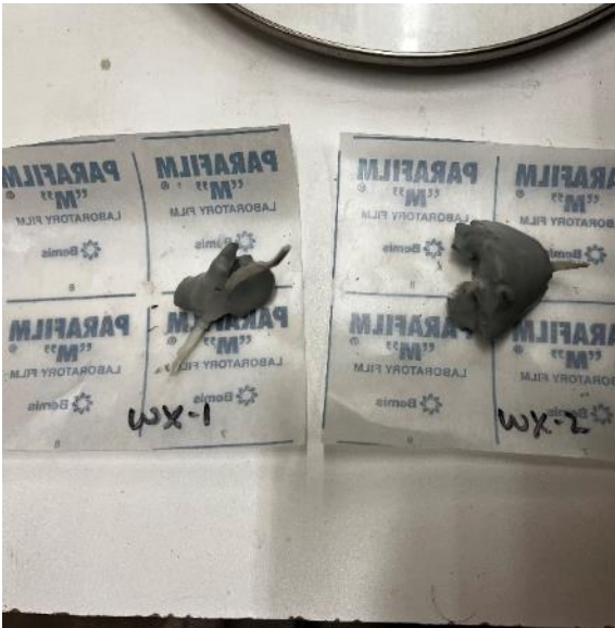
Photo 22. Density samples processed from B-1
