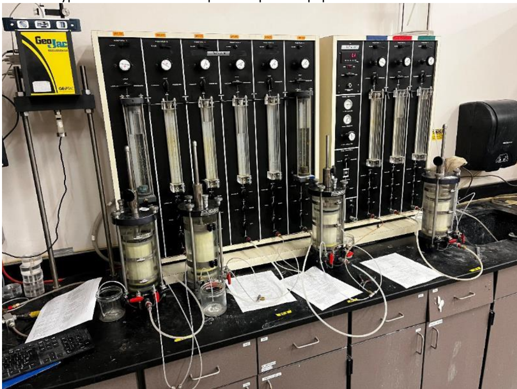
Photo 83. Triaxial equipment, cells, samples, pressure panels, and GeoJac for triaxial testing
