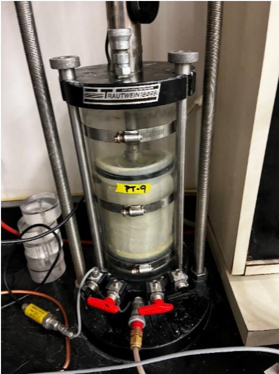
Photo 75. PT-9 post shear testing
