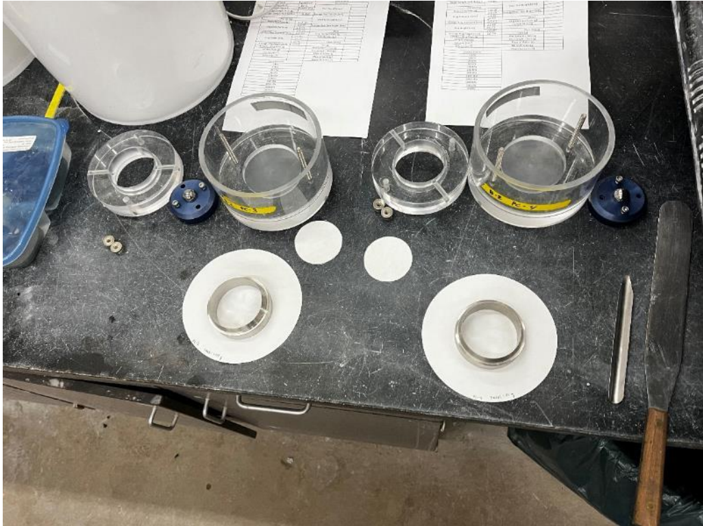
Photo 82. Typical consolidation sample set up and equipment for each desiccation bucket
