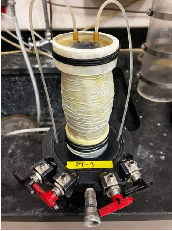
Photo 48. PT-3 post shear testing
