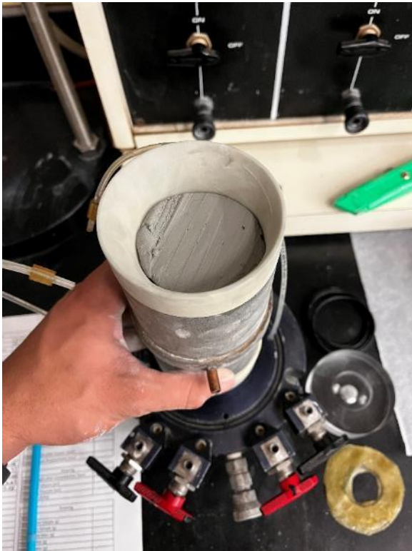
Photo 39. PT-3 placement on end platens
