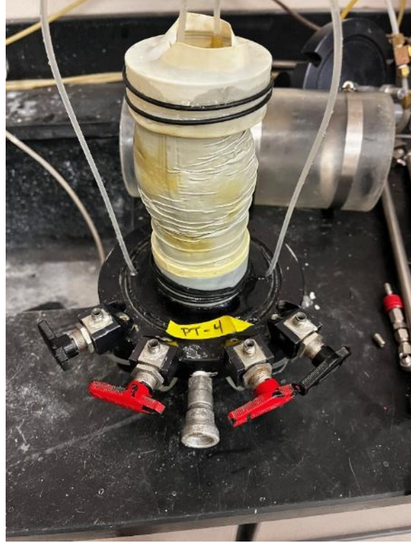
Photo 49. PT-4 post shear testing
