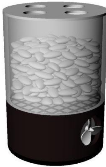
Figure 3.1. A 55-gallon drum equipped with a fan and mesh screening across the lower quarter to elevate tubers and facilitate air circulation. The fan controls were passed through a hole drilled in the drum and sealed with duct tape.
