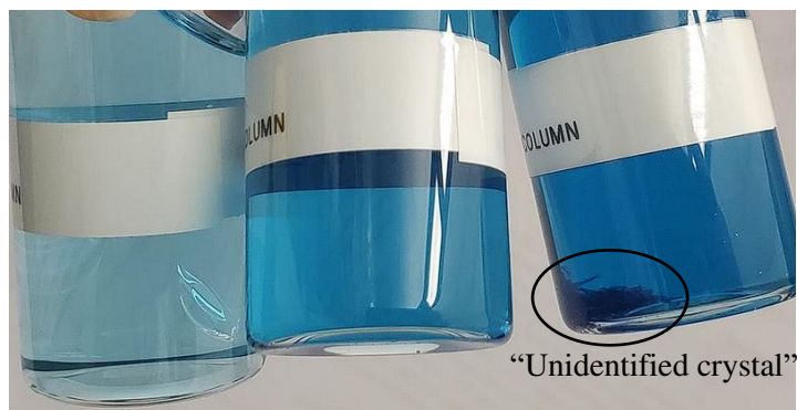
Figure 4.20. Fractions (20 mL) collected from performing the Friedländer synthesis under continuous flow conditions. On the fraction on the right, you can see “unidentified crystal” that had recrystallized out of the fraction after it sat at room temperature for about 24 hours.
