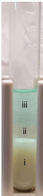
Figure 2.2. Layering of the different components used to synthesize the CuBDTri nanosheets. The labels i, ii, and iii correspond to \text{H}_2\text{BDTri} dissolved in a 2:1 mixture of water/DMF, a solvent spacer comprised of a 1:1 mixture of water/DMF, and then \text{CuCl}_2 \cdot \text{H}_2\text{O} dissolved in a 1:2 mixture of water/DMF, respectively.
