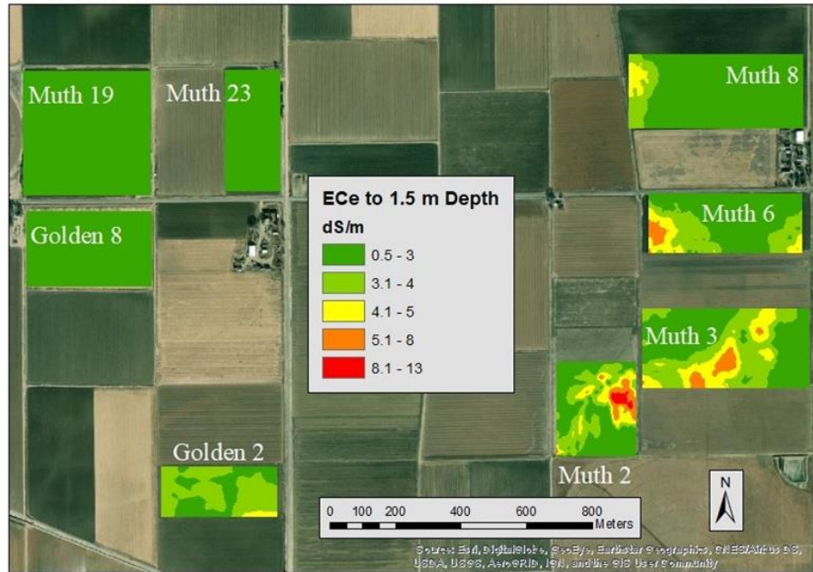
Figure 11: Map of the 2019 EC_e survey derived from the ME-38 in dS\ m^{-1} . Muth 2, Muth 3, Muth 6, Muth 8 and Golden 2 were used in the multiple linear regression model.
