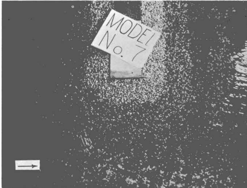
Fig. 31 - Photograph of the abutment for a discharge of 0.94 cfs showing the separation on the upstream (left) shoulder
