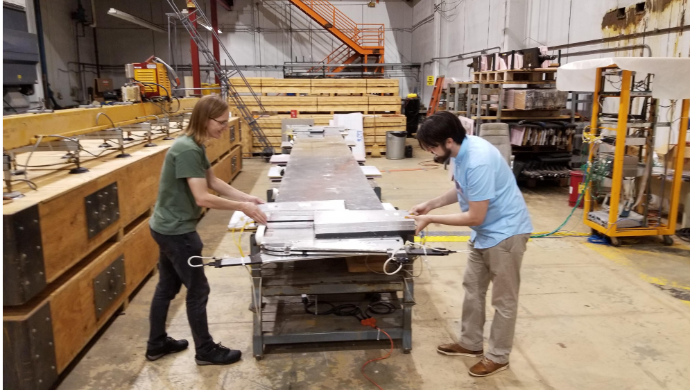
Figure 2.18: University of Houston postdoctoral researcher Antoni Aduszkiewicz and (at the time) CSU graduate student Chris Hilgenberg align the hodoscopes on the MINOS modules at the Wideband test stand. Photo credit: Robert Wilson.
