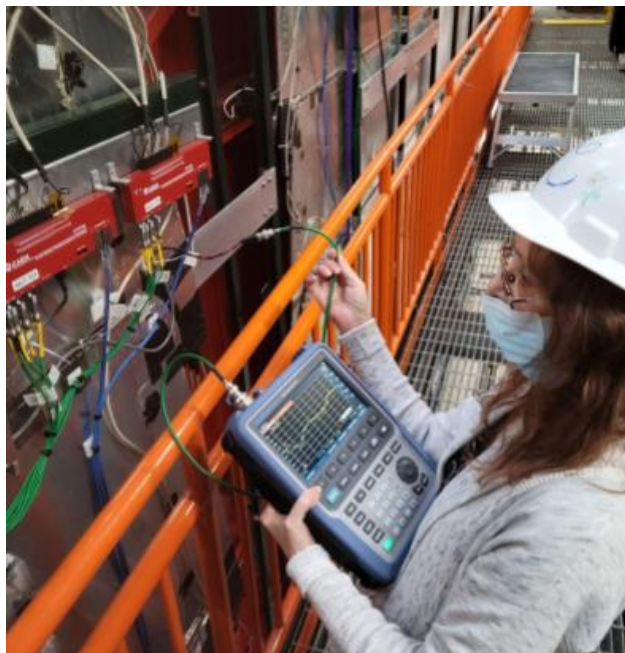
Figure 3.2: Fermilab Engineer Linda Bagby demonstrates use of a spectrum analyzer to look for which frequencies may be more pronounced on an input FEB power cable on the Side CRT.
