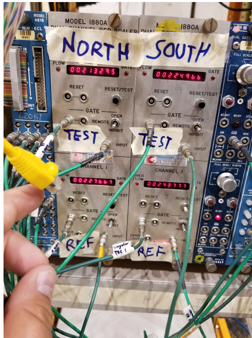
Figure 2.20: The counters used at Wideband to count signals seen by the hodoscopes compared to those seen by the test modules.
