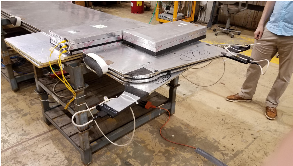
Figure 2.19: A closer look at the south end of the Wideband test stand to better show the module ends and placement of hodoscopes. Photo credit: Robert Wilson.
