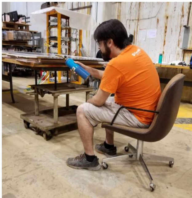
Figure 2.36: Chris Hilgenberg uses a blowtorch in the final stage of preparing the cut modules to be mirrored with Mylar and then sealed with electrical tape.
