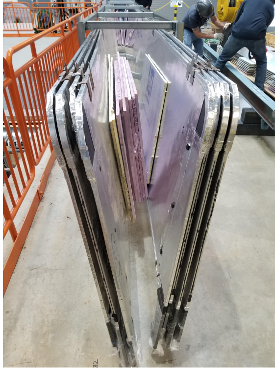
Figure 2.41: Fermilab technician Kelly Hardin had a rig created to be able to transfer multiple MINOS modules from the loading dock to the top of the ICARUS detector.
