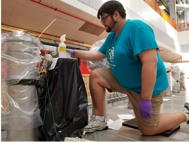
Figure 1.2: Checking some of the >53,000 TPC wire signals during commissioning.
