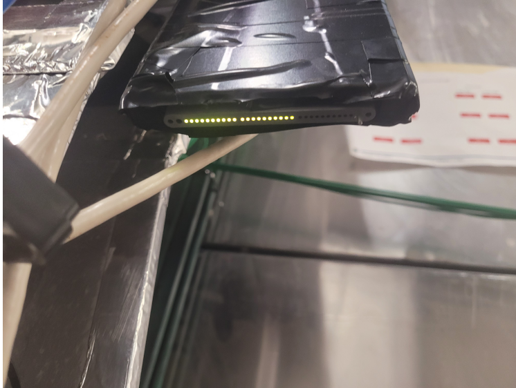
Figure 2.8: A MINOS snout with light illuminating the other end to make the active channels identifiable.
