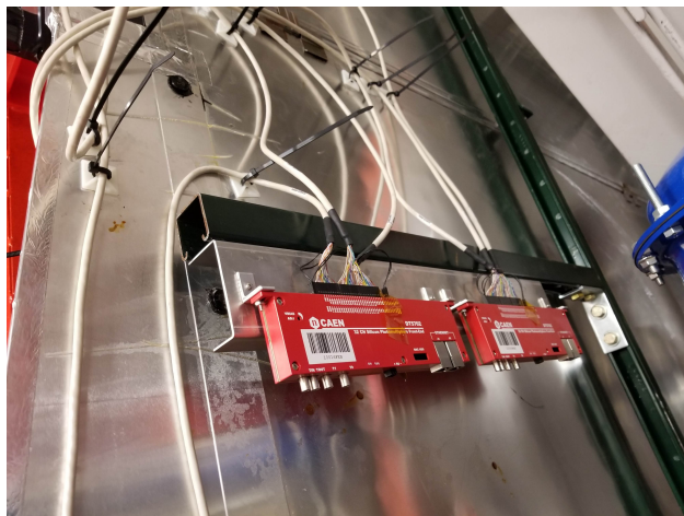
Figure 2.43: Front-End Boards mounted on a finger which extends from the main support post.
