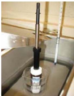
Figure 2.4: Extraction with SPME
