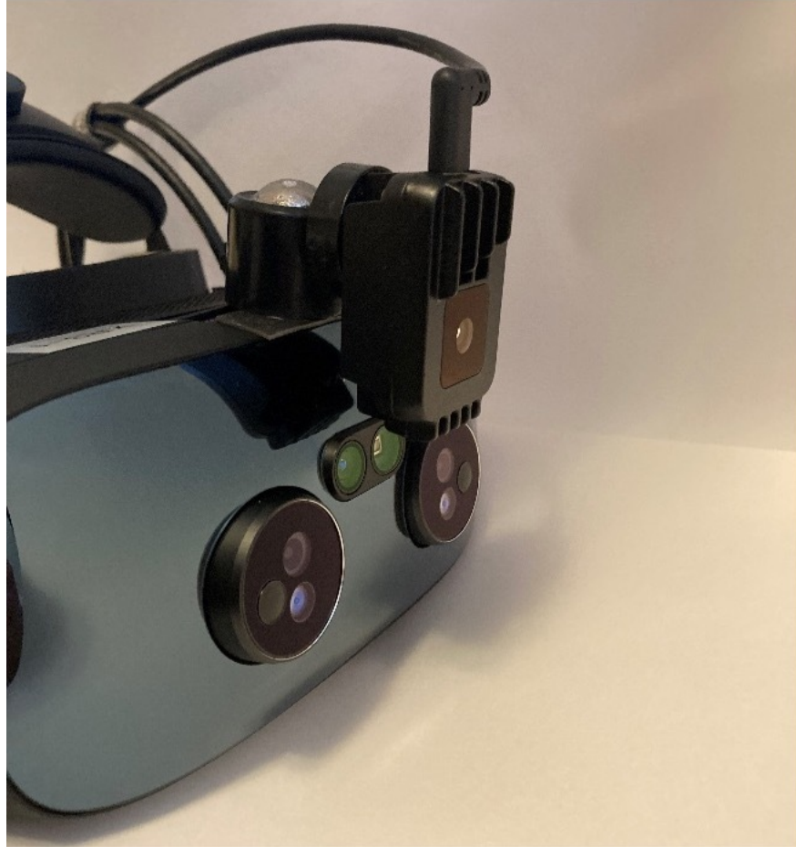
Figure 6.2: OAK-1 camera mounted on XR-3.
