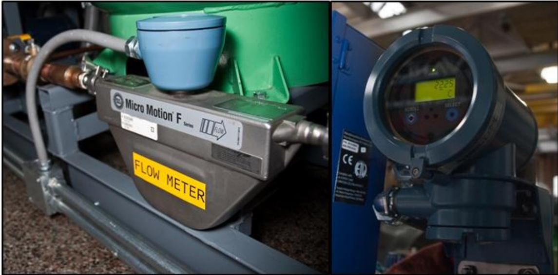
Figure 5-10: Micro Motion coriolis flow meter sensor (left) and transmitter (right).
