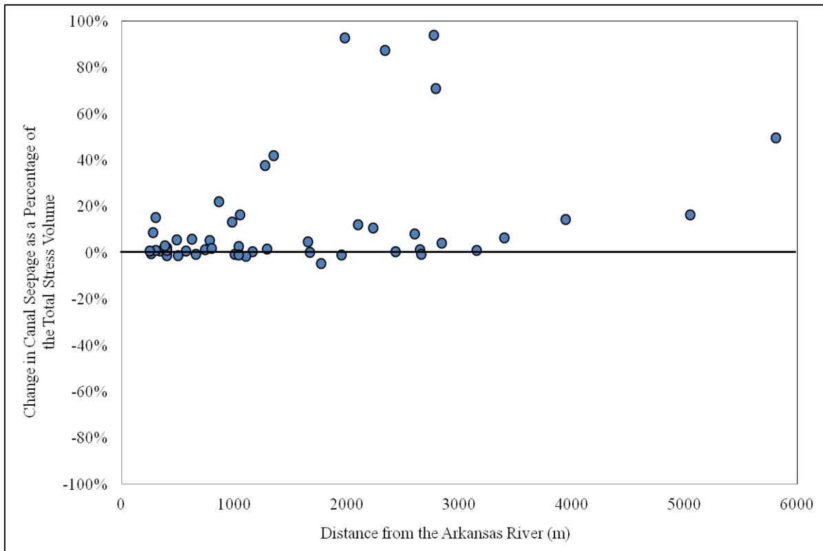
Figure 4.18. Change in canal interception predicted by the MODFLOW-UZF model as a percentage of the stress volume by water addition versus distance to the Arkansas River.
