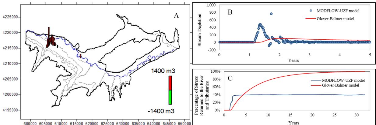
Figure 4.27. (A) Bar plot of stream depletion within the LARV for Field 7, (B) the amount of stream depletion occurring throughout the 32-year simulation period, as predicted by the Glover-Balmer solution and MODFLOW-UZF model, and (C) the cumulative depletion expressed as a percentage of the total stress volume.
