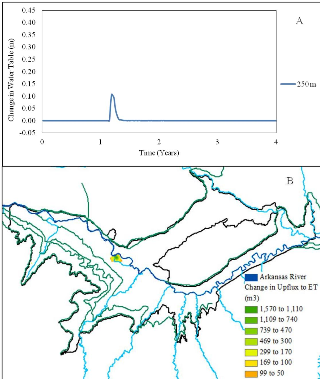
Figure 4.13. (A) The water table elevation change for grid cells in a straight-line path between the stressed cell and Arkansas River, and (B) the total change in upflux to ET for each grid cell for the 32-year simulation period.
