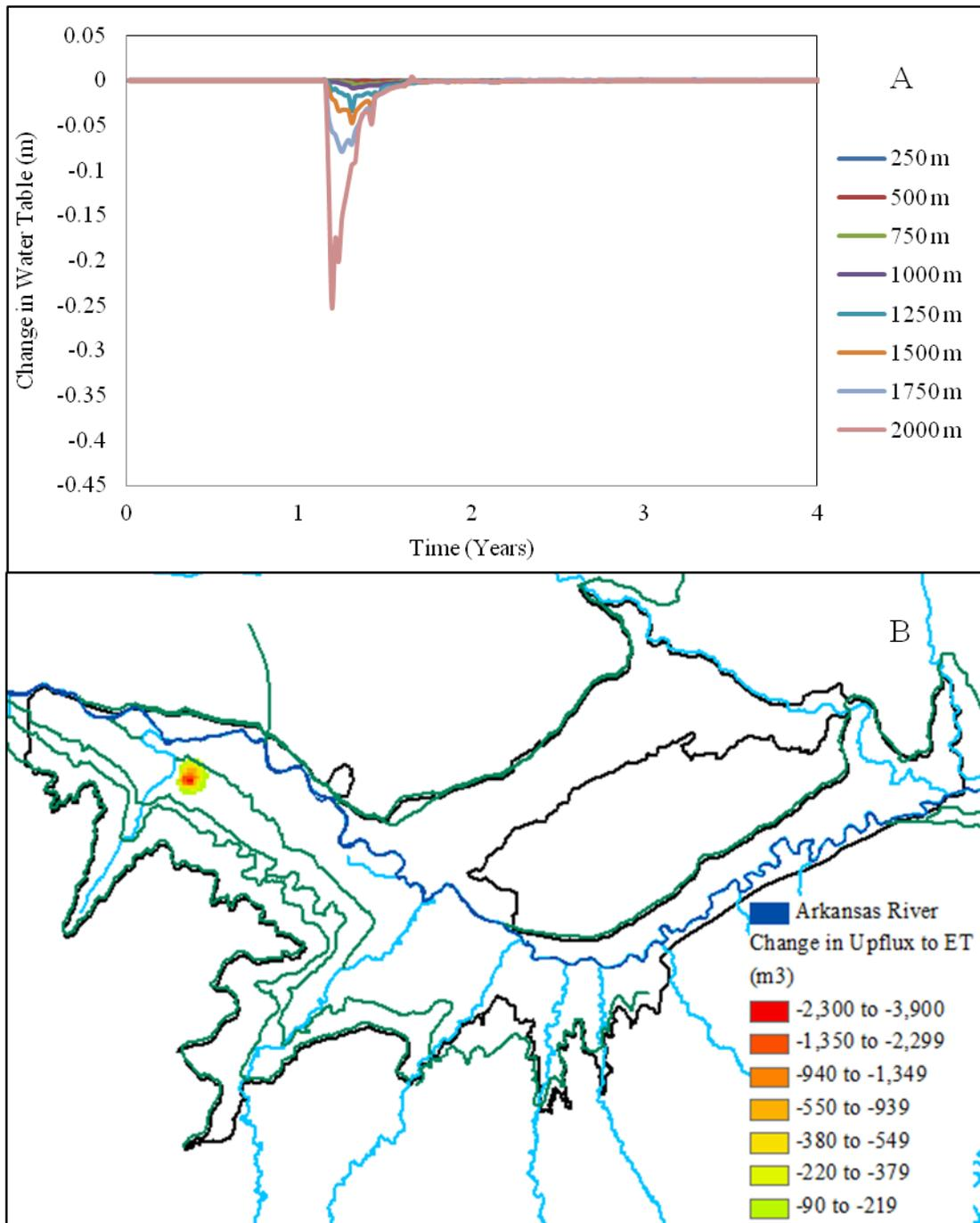
4.28. (A) The water table elevation change for grid cells in the shortest straight-line path between the stressed cell and Arkansas River, and (B) the total change in upflux to ET for each grid cell in the 32-year simulation period.
