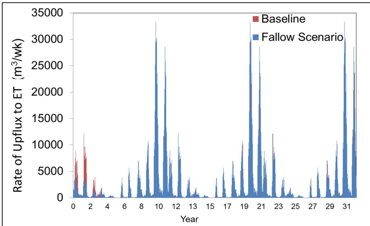
Figure 4.3. Predicted contribution to ET by upflux from the saturated zone for the baseline and fallowing MODFLOW-UZF scenarios.
