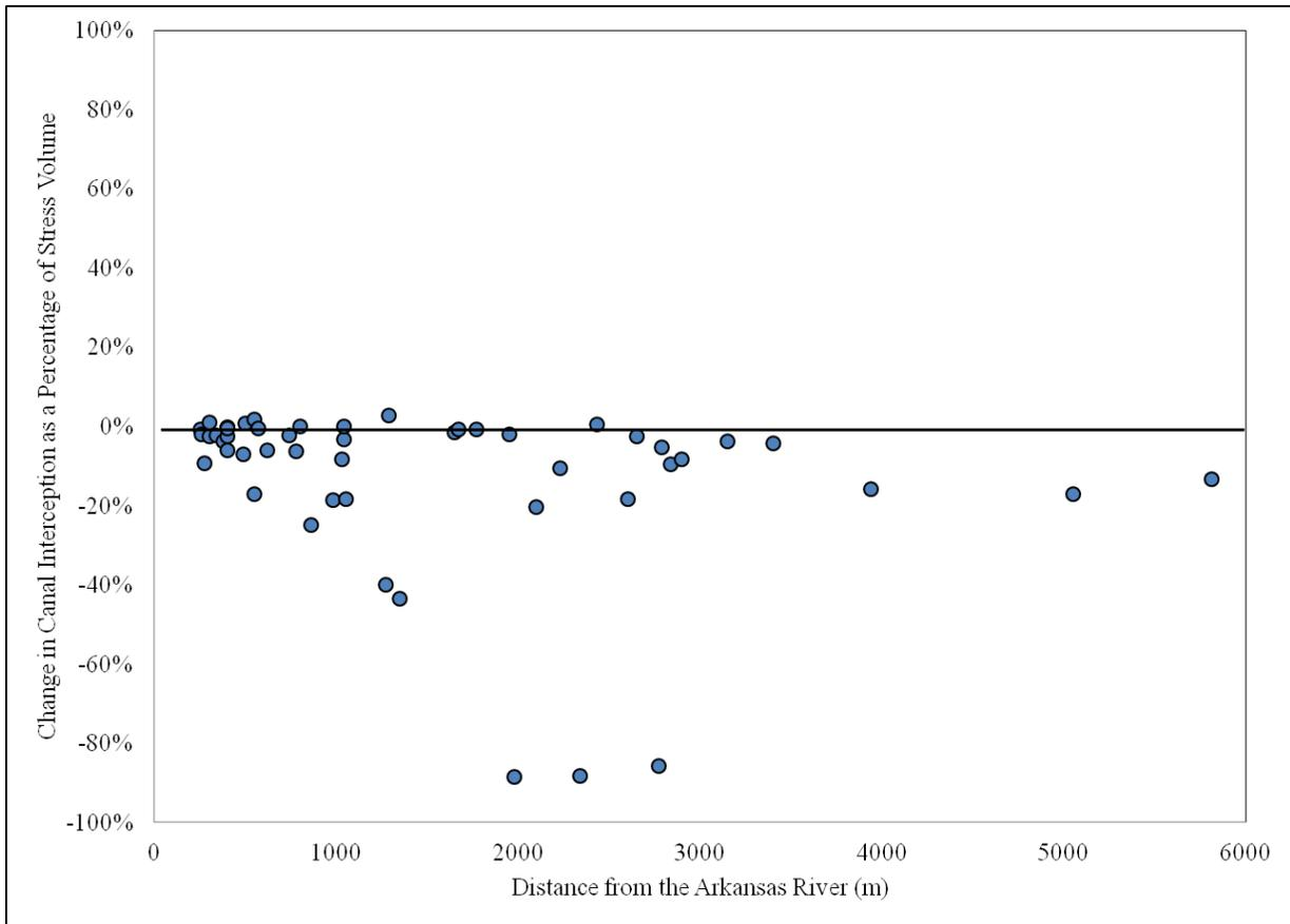
Figure 4.30. Change in canal interaction predicted by the MODFLOW-UZF model as a percentage of stress volume by water extraction versus distance to the Arkansas River.
