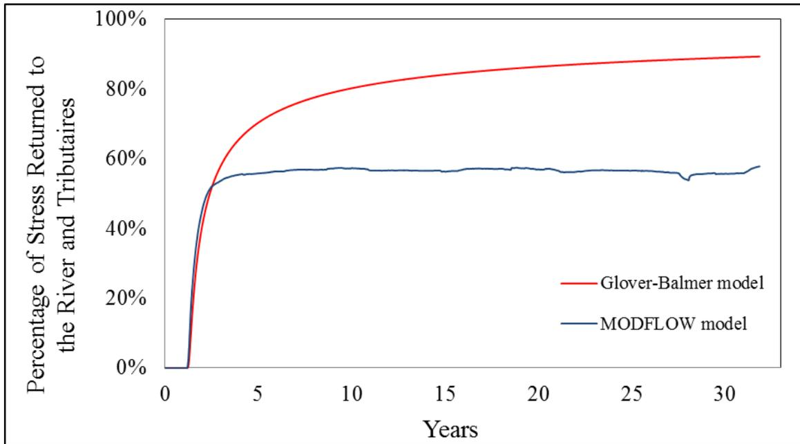
Figure 3.3. An example of URFs developed from the Glover-Balmer model and the MODFLOW-UZF model for a particular scenario.
