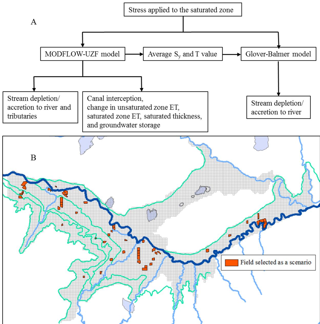
Figure 3.2. (A) Flow chart of the general structure of extraction/addition scenarios used for the evaluation of the Glover-Balmer solution by comparison to a calibrated MODFLOW-UZF numerical model, and (B) the fields selected as comparison scenarios within the LARV.
