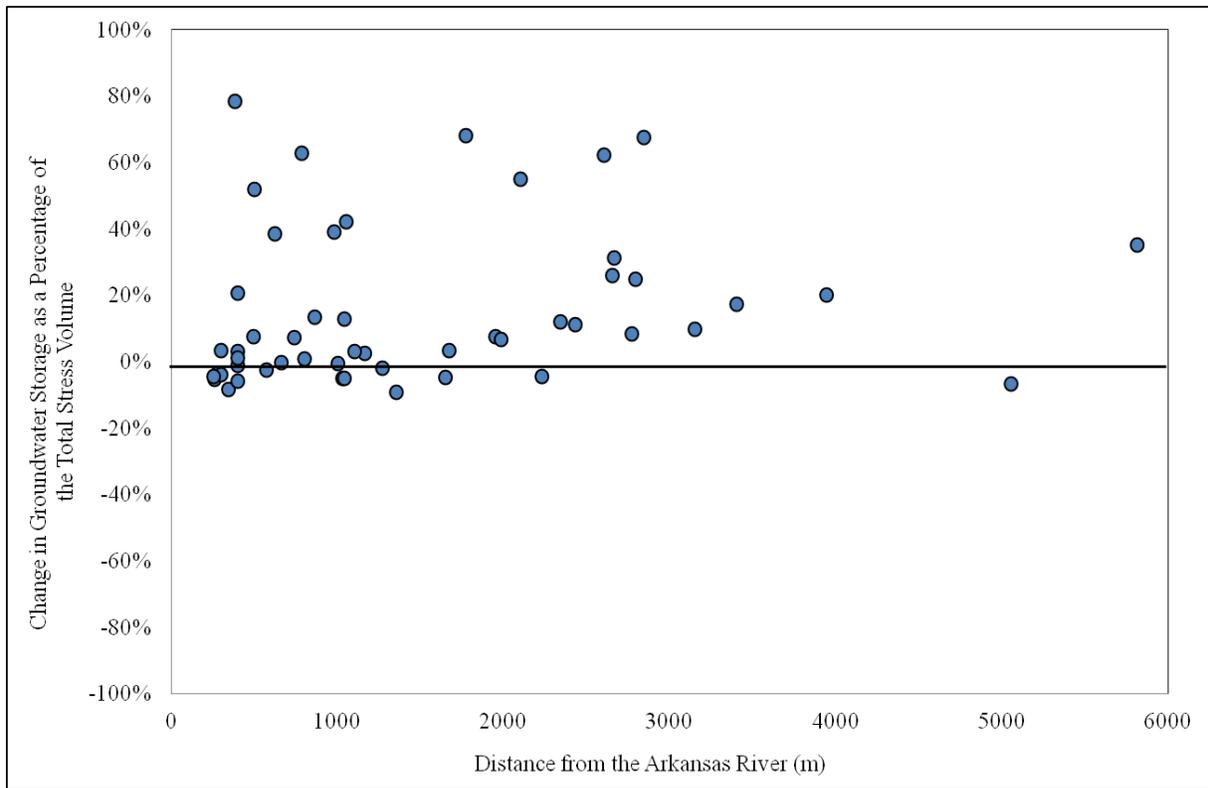
Figure 4.19. Change in groundwater storage predicted by the MODFLOW-UZF model as a percentage of stress volume by water addition versus distance to the Arkansas River.
