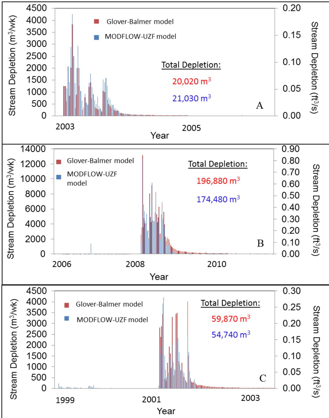
Figure 4.10. Weekly stream depletion estimates from the MODFLOW-UZF model and the Glover-Balmer solution for the case of following Field 4 within (A) a relatively dry hydrologic year (2003), (B) an average year (2008), and (C) a relatively wet year (1999).
