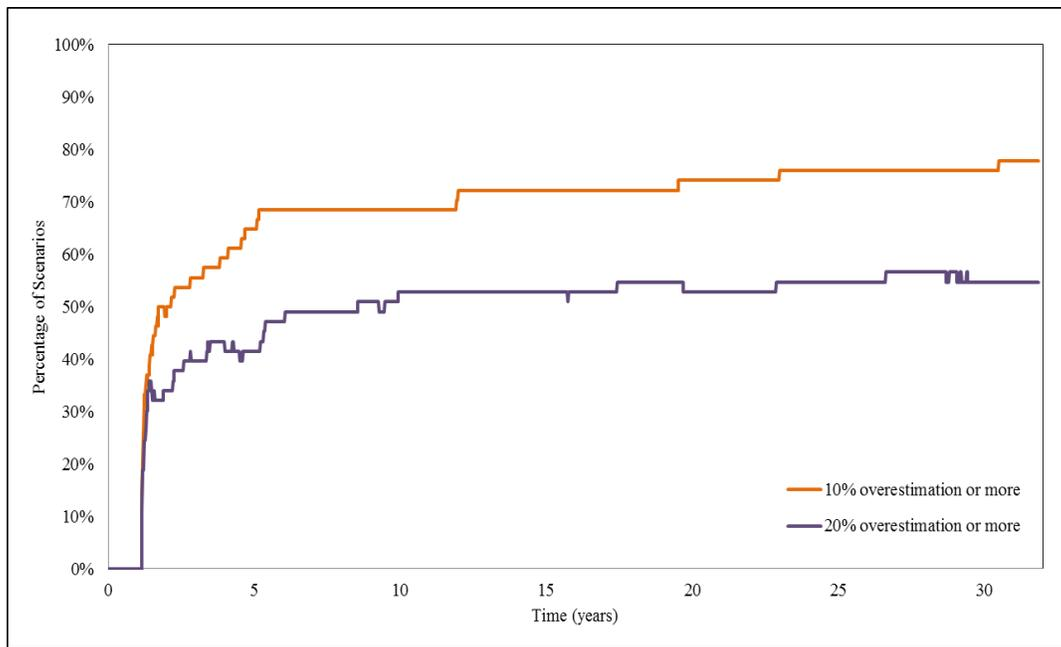
Figure 4.33. Percentage of scenarios in which the Glover-Balmer model overestimates stream depletion in comparison to predictions by the calibrated MODFLOW-UZF model by at least 10% or 20% for water extraction scenarios.
