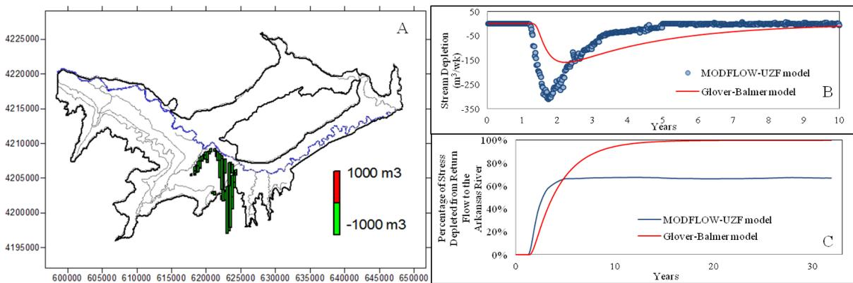
Figure 4.15. (A) Bar plot of stream accretion (negative depletion) as predicted by the MODFLOW-UZF model for Field 6, (B) the time period in which stream accretion occurs within the 32-year simulation period, as predicted by the Glover-Balmer solution and MODFLOW-UZF model, and (C) the cumulative stream accretion expressed as a percentage of the total stress volume.
