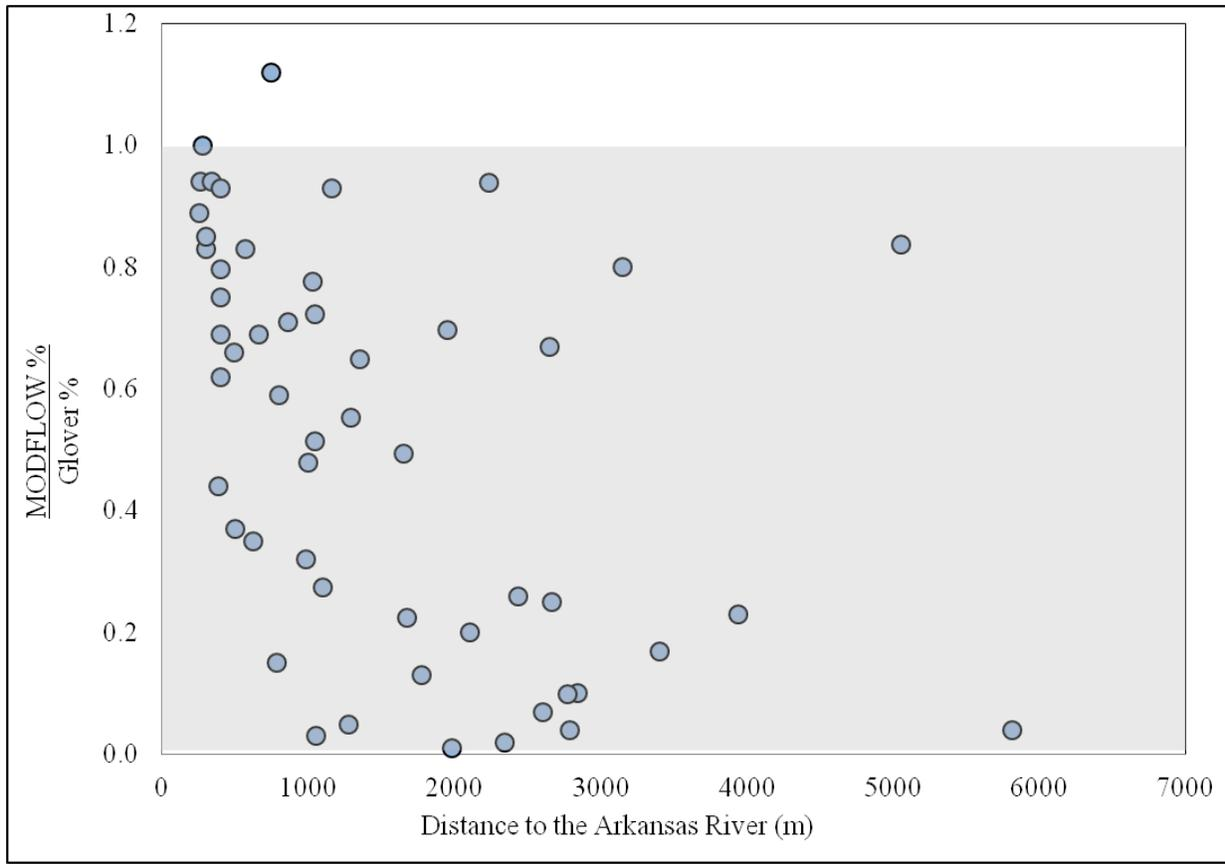
Figure 4.20. The ratio of the cumulative volume of stream accretion as a percentage of the stress volume predicted by the MODFLOW-UZF model divided by the cumulative volume of accretion as a percentage of the stress volume predicted by the Glover-Balmer method at the end of the 32-year simulation for 52 scenarios of water addition to the saturated zone versus distance from the Arkansas River.
