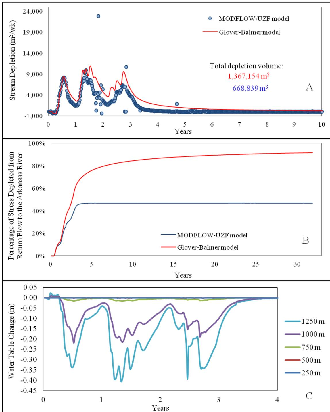
Figure 4.2. (A) The amount of stream depletion occurring at each timestep throughout the 32-year simulation period, as predicted by the Glover-Balmer solution and MODFLOW-UZF model, (B) the cumulative depletion expressed as a percentage of the total fallowed volume, and (C) the change in water table elevation for each cell in a straight-line path from the Arkansas River to the fallowed field.
