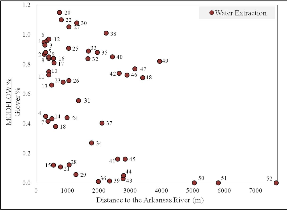
Figure A.2. The ratio of the cumulative volume of stream depletion as a percentage of the stress volume predicted by the MODFLOW-UZF model divided by the cumulative volume of depletion as a percentage of the stress volume predicted by the Glover-Balmer method at the end of the 32-year simulation for 52 scenarios of water extraction from the saturated zone versus distance from the Arkansas River, with data labels of exact distances for reference in the following detailed tables.
