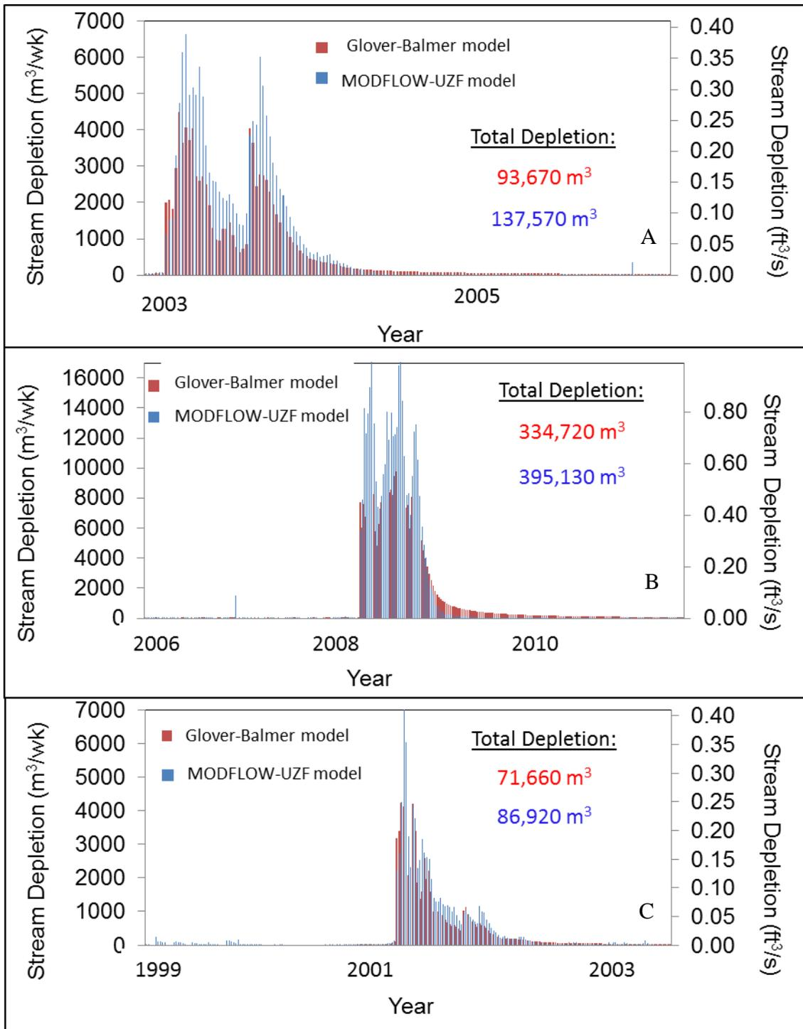
Figure 4.8. Weekly stream depletion estimates from the MODFLOW-UZF model and the Glover-Balmer solution for the case of following Field 3 within (A) a relatively dry hydrologic year (2003), (B) an average year (2008), and (C) a relatively wet year (1999).
