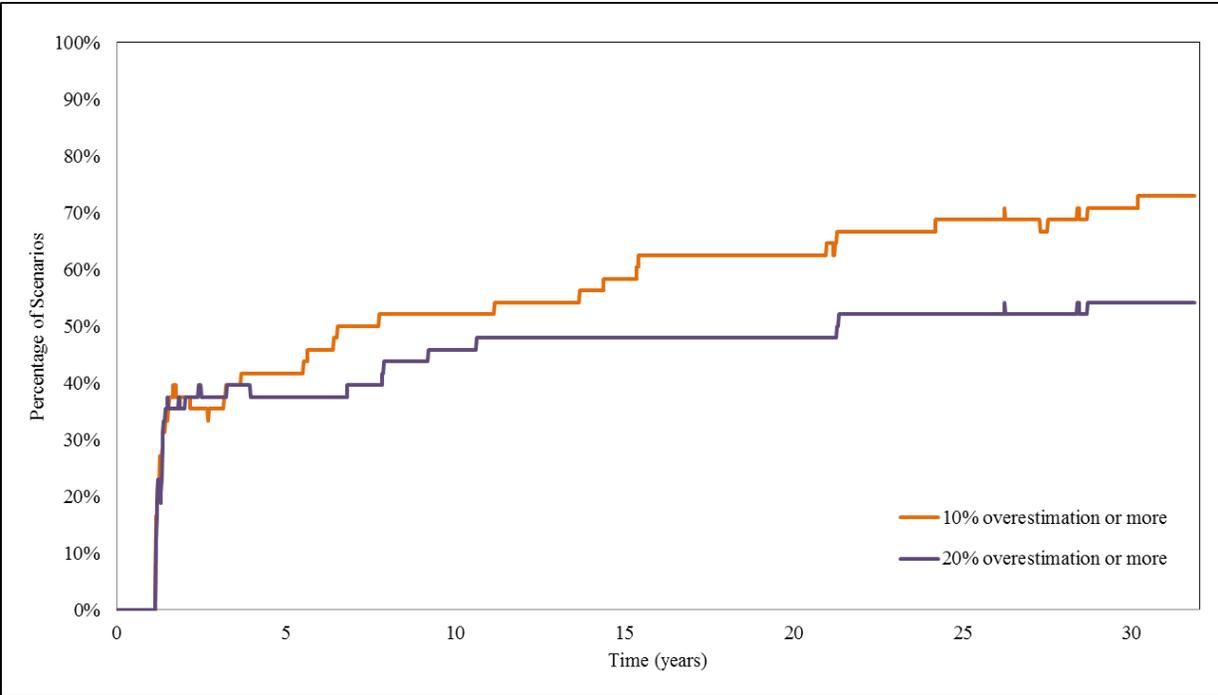
Figure 4.21. Percentage of scenarios in which the Glover-Balmer solution overestimates stream accretion in comparison to predictions by the calibrated MODFLOW-UZF model by at least 10% or 20% for water addition scenarios.
