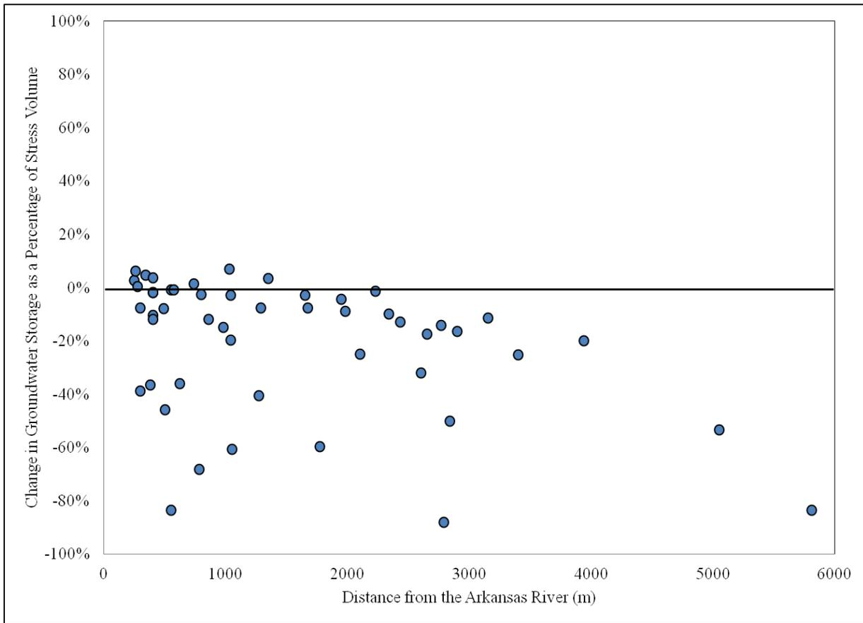
Figure 4.31. Change in groundwater storage predicted by the MODFLOW-UZF model as a percentage of the stress volume versus distance to the Arkansas River.
