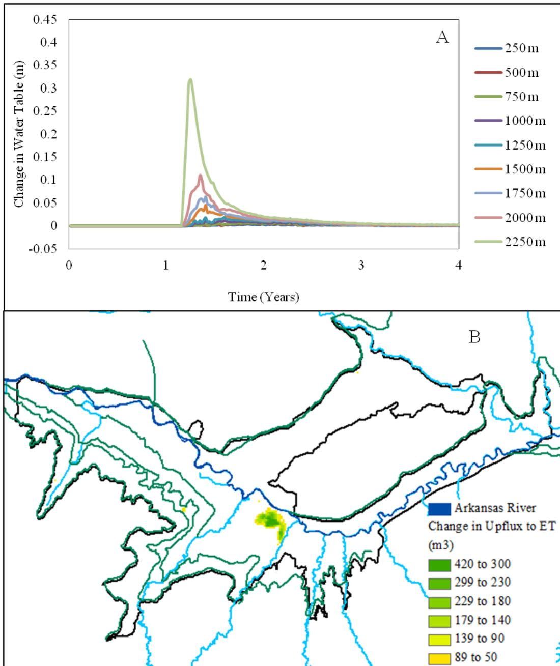
Figure 4.16. (A) The water table elevation change for grid cells in a straight-line path between the stressed cell and Arkansas River, and (B) the total change in upflux to ET for each grid cell in the 32-year simulation period.
