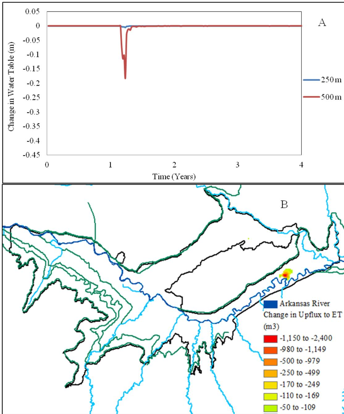
Figure 4.25. (A) The water table elevation change for MODFLOW-UZF model grid cells in the shortest straight-line path between the stressed cell and Arkansas River, and (B) the total change in upflux to ET for each grid cell for the 32-year simulation period.
