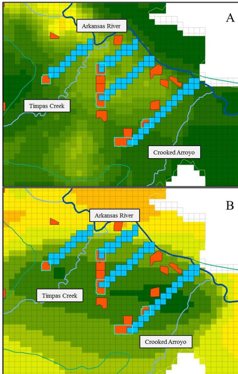
Figure 3.1. Examples of the selection of model cells in a straight-line (blue cells) for several example fields (shown in orange), with minimum distance from the Arkansas River for time- and depth-averaged (A)  $T$  values, and (B)  $S_y$  values.
