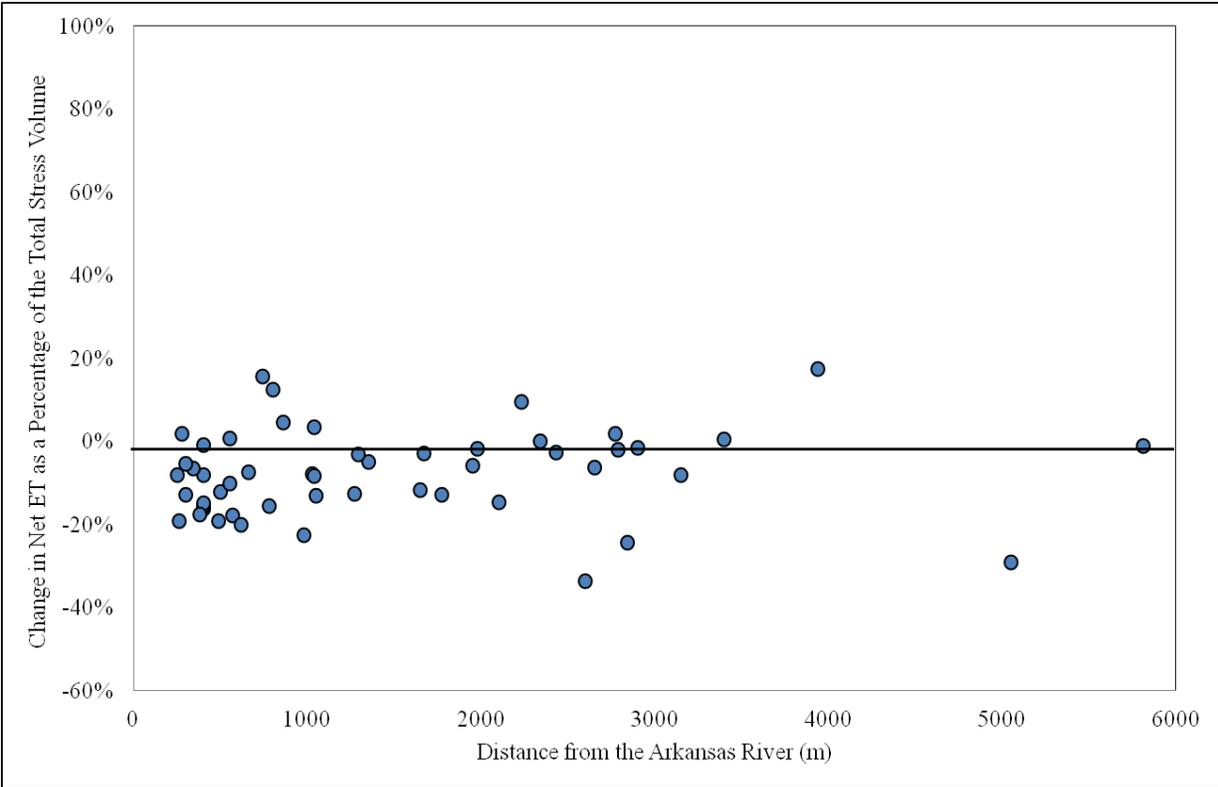
Figure 4.29. Change in groundwater storage predicted by the MODFLOW-UZF model as a percentage of the stress volume by water extraction versus distance from the Arkansas River.
