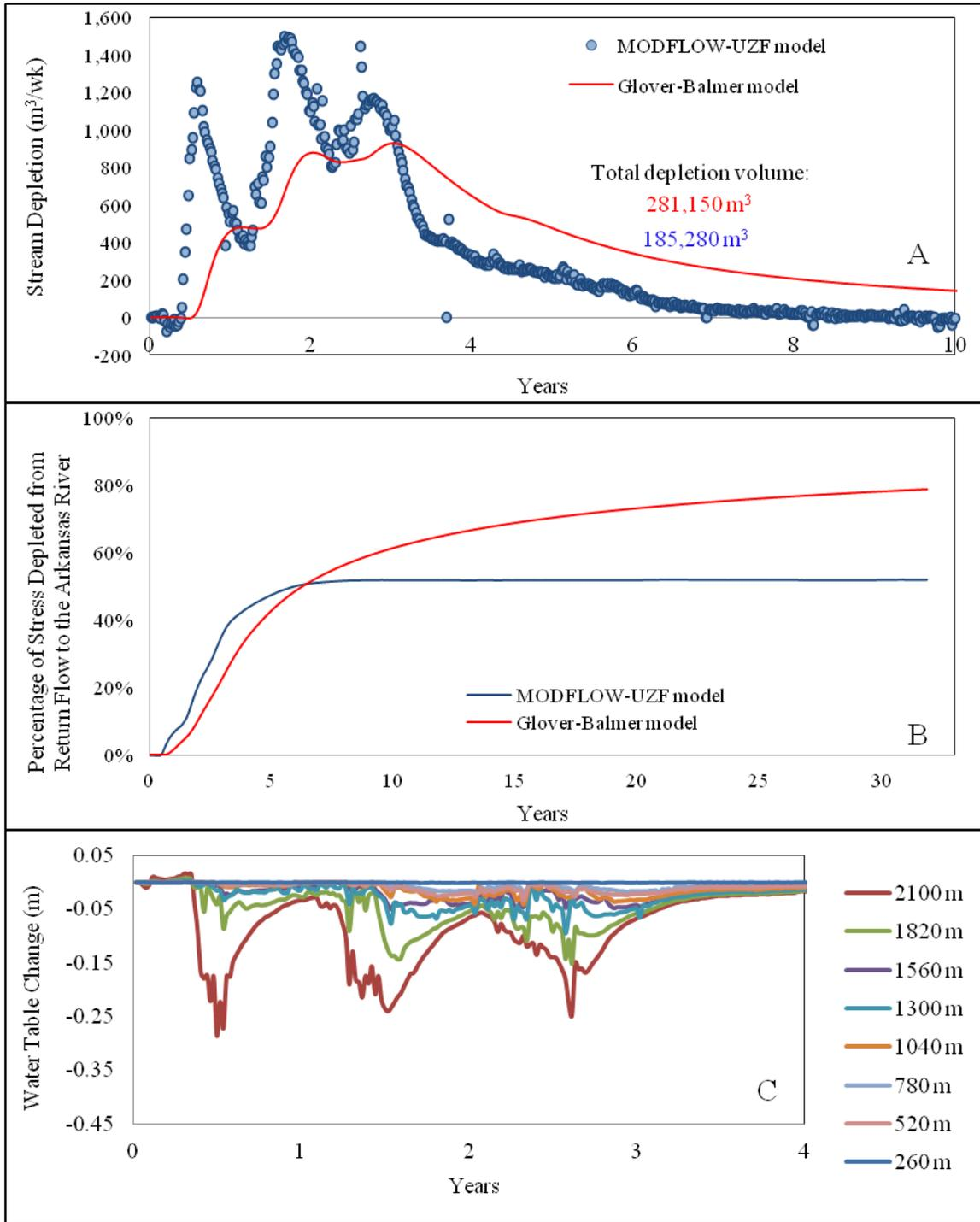
Figure 4.5. (A) The amount of stream depletion occurring at each timestep throughout the 32-year simulation period, as predicted by the Glover-Balmer solution and MODFLOW-UZF model, (B) the cumulative depletion expressed as a percentage of the total fallowed volume, and (C) the change in water table elevation for each cell in a straight-line path from the Arkansas River to the fallowed field.
