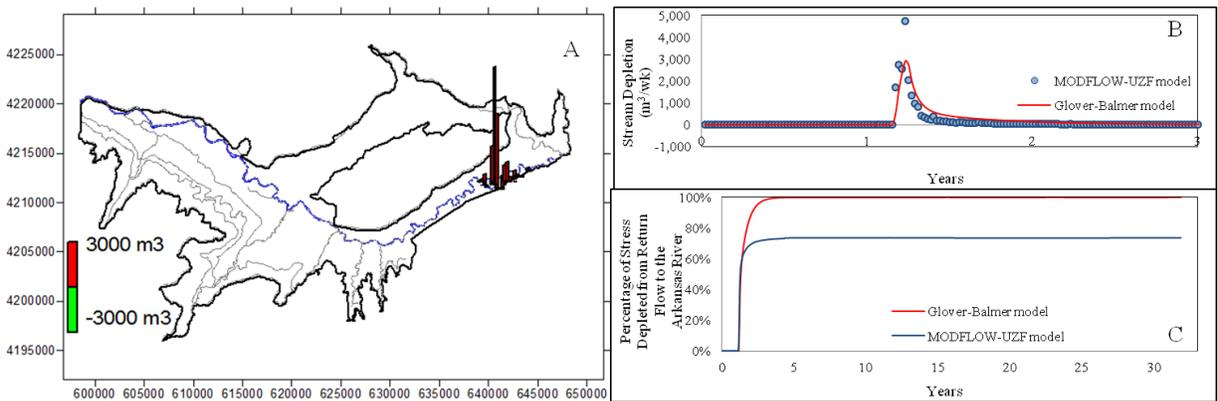
Figure 4.24. (A) Bar plot of stream depletion within the LARV for Field 7, (B) the amount of stream depletion occurring throughout the 32-year simulation period, as predicted by the Glover-Balmer solution and MODFLOW-UZF model, and (C) the cumulative depletion expressed as a percentage of the total stress volume.
