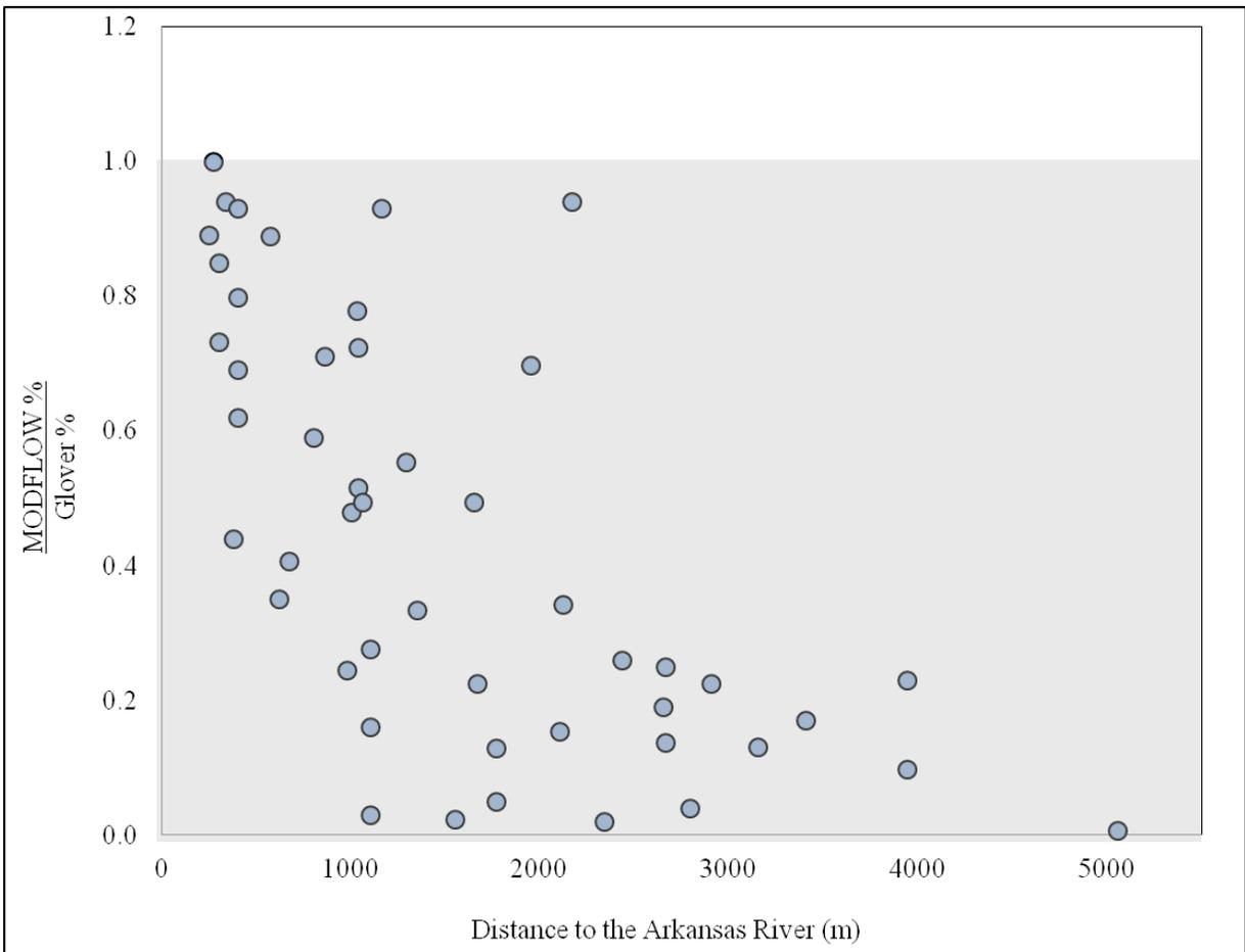
Figure 4.22. The ratio of the cumulative volume of stream accretion as a percentage of the stress volume predicted by the MODFLOW-UZF model divided by the cumulative volume of accretion as a percentage of the stress volume predicted by the Glover-Balmer method at the end of the 32-year simulation for 49 scenarios of water addition to the ground surface versus distance from the Arkansas River.
