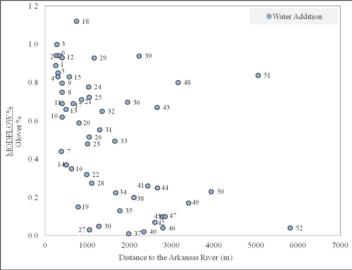
Figure A.1. The ratio of the cumulative volume of stream accretion as a percentage of the stress volume predicted by the MODFLOW-UZF model divided by the cumulative volume of accretion as a percentage of the stress volume predicted by the Glover-Balmer method at the end of the 32-year simulation for 52 scenarios of water addition to the saturated zone versus distance from the Arkansas River, with data labels of exact distances for reference in the following detailed tables.
