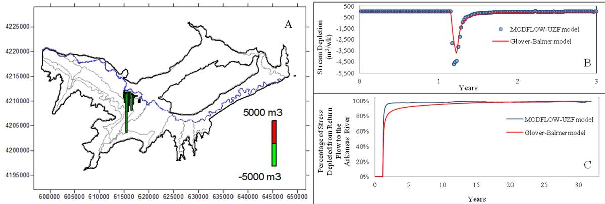
Figure 4.12. (A) Bar plot of stream accretion (negative depletion) as predicted by the MODFLOW-UZF model for Field 5, (B) the time period in which stream accretion occurs within the 32-year simulation period, as predicted by the Glover-Balmer solution and MODFLOW-UZF model, and (C) the cumulative accretion expressed as a percentage of the total stress volume.
