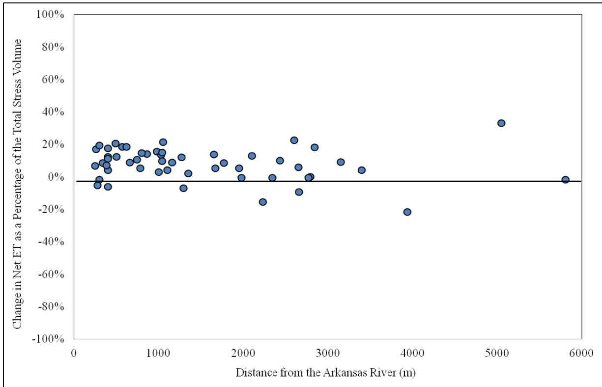
Figure 4.17. The change in net ET predicted by the MODFLOW-UZF mode as a percentage of stress volume by water addition versus distance to the Arkansas River.
