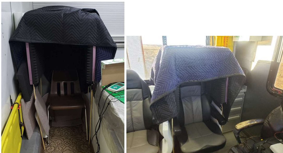
Figure 1a and 1b. Portable booth setup in trailers provided by the company at the (1a) quiet fleet site and (1b) conventional fleet site. This booth was built by researchers to reduce ambient noise for pure-tone audiometry hearing tests. A small rug, carpet tiles, and acoustic panels were used to further reduce noise.
