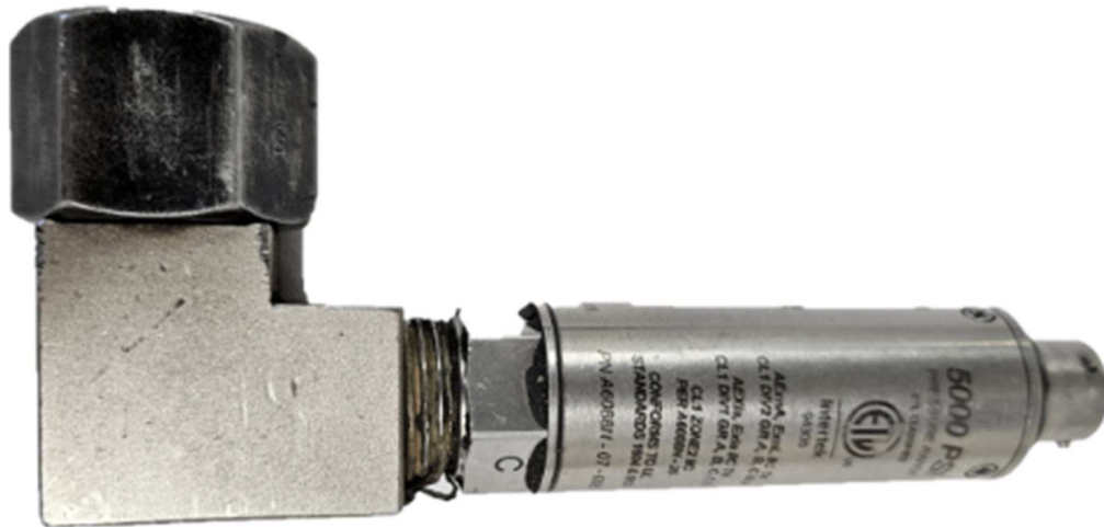
Figure 12: Example of a pressure transducer, which was used to measure the pressure in each cylinder of the operating KVSr 412.
