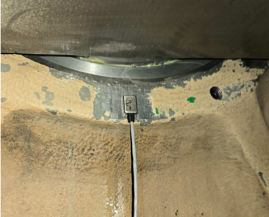
Figure 69: Dynamic strain sensor installed at Location #1 on the #3 main bearing.
