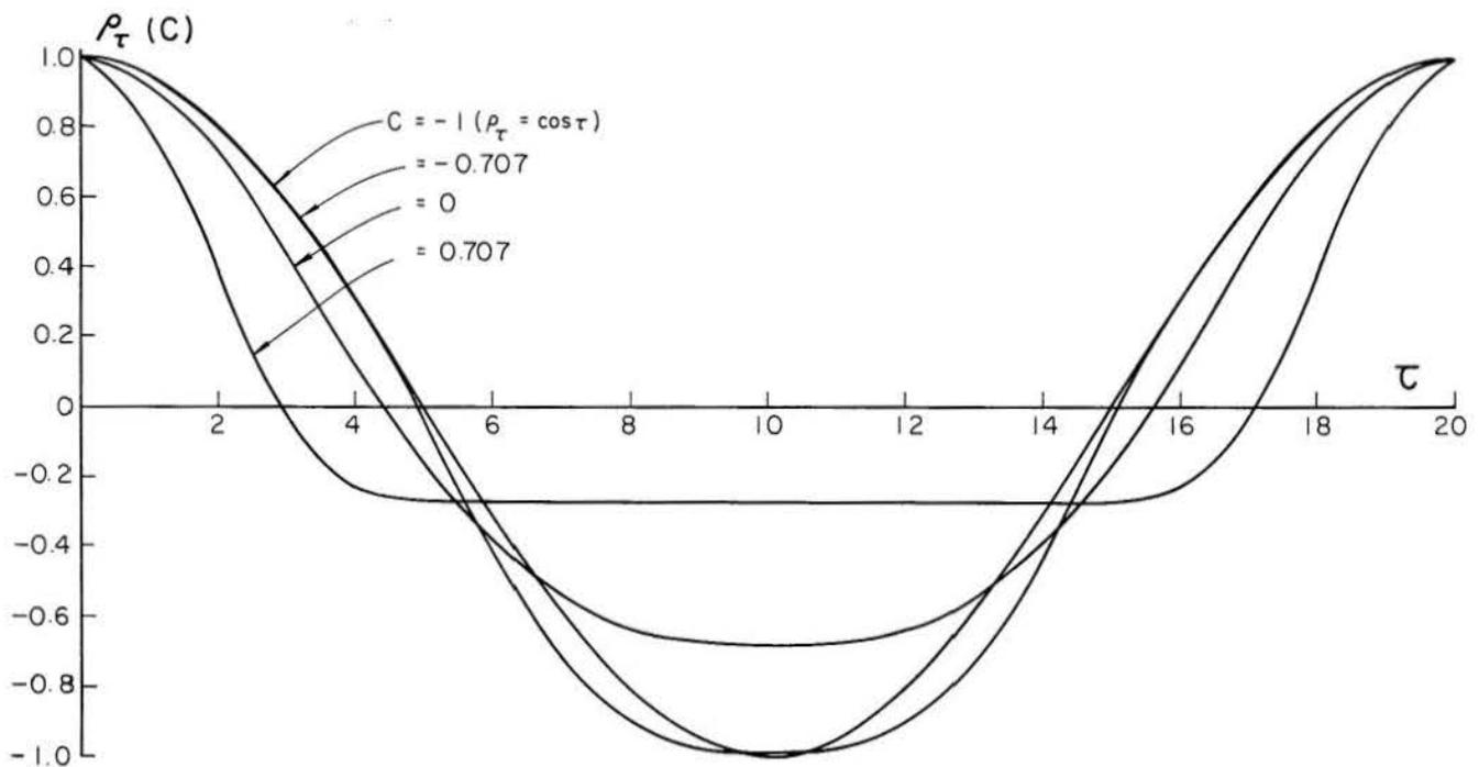
Fig. 6. Autocorrelation coefficients of a sinusoidal series  $x_t = A \sin \omega t$ , (with both the amplitude  $A$  and angular frequency  $\omega$  being unities) truncated at four constant values:  $c = -1$ ;  $c = -0.707$ ;  $c = 0$ ; and  $c = 0.707$
