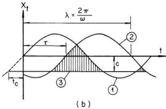
Fig. 1. Schematic diagram for the lagged cross product of a sinusoidal series: (1) sine series; (2) shifted series for  $\tau$ ; (3) level of truncation
