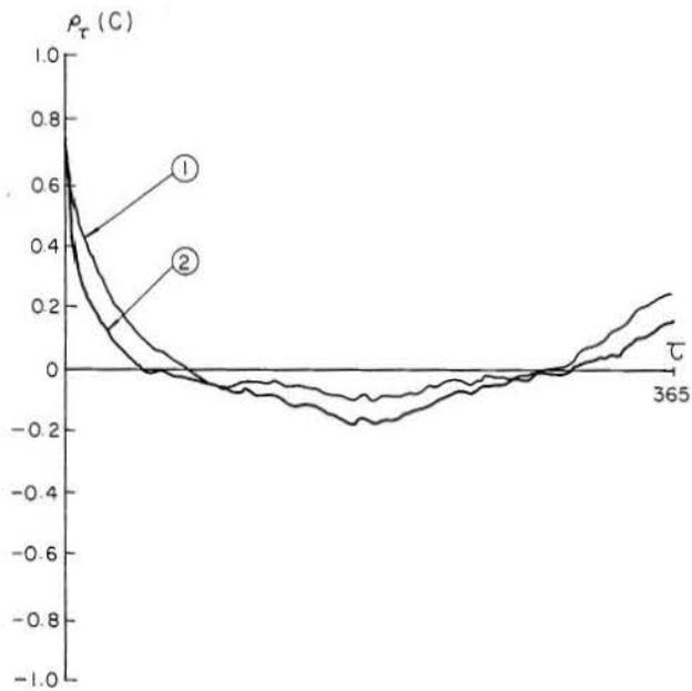
Fig. 9. Correlogram of truncated and untruncated series of daily flows of the Batten Kill River at Battenville, N. Y.: (1) correlogram of untruncated series; and (2) correlogram of truncated series; with  $c = \bar{x}$
