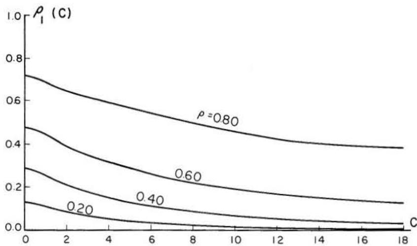
Fig. 5. First autocorrelation coefficient as a function of the level of truncation  $c$  for lognormal process of the first order Markov linear model of eqs. (17) and (18), for four values of  $\rho_1 = \rho$ :  $0.20, 0.40, 0.60$  and  $0.80$
