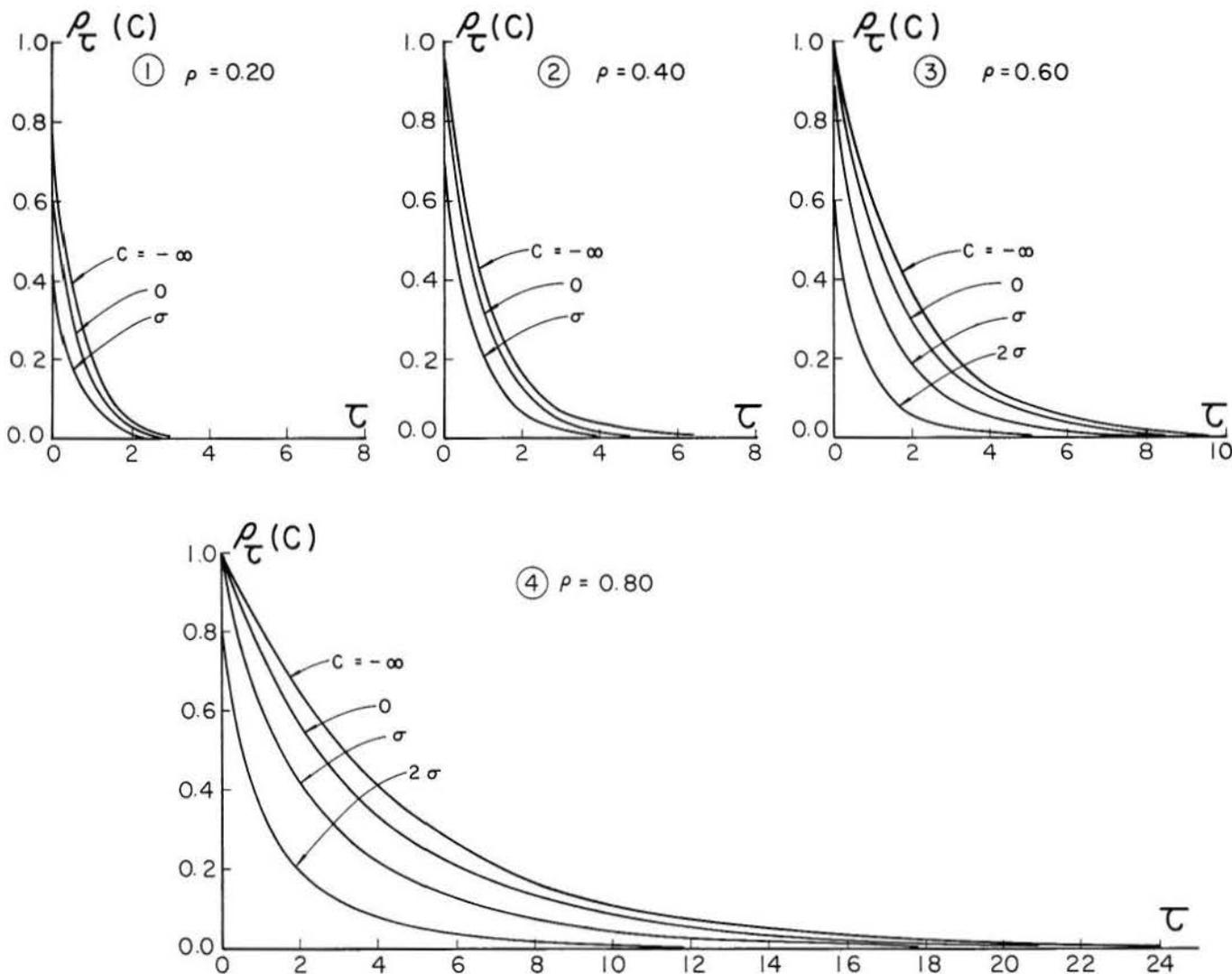
Fig. 2. Correlograms of the truncated normal process of the first order Markov linear model for: (1)  $\rho = 0.20$ ; (2)  $\rho = 0.40$ ; (3)  $\rho = 0.60$ ; and (4)  $\rho = 0.80$ . The truncation constants  $c$  are either  $-\infty$ ,  $0$  and  $\sigma$ ; or  $-\infty$ ,  $0$ ,  $\sigma$  and  $2\sigma$
