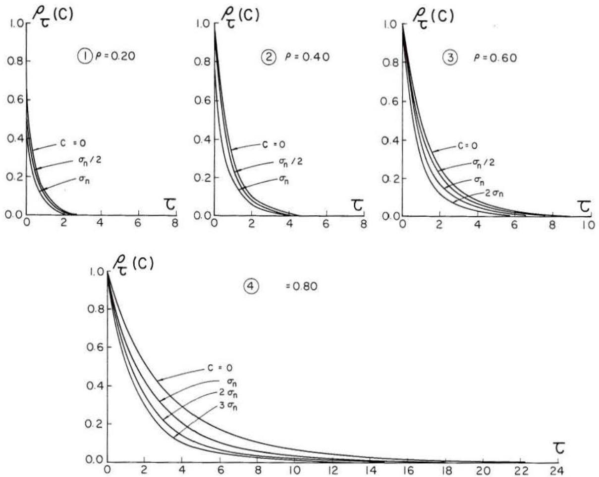
Fig. 4. Correlograms of the truncated lognormal process of the first order Markov linear model for: (1)  $\rho = 0.20$ ; (2)  $\rho = 0.40$ ; (3)  $\rho = 0.60$  and (4)  $\rho = 0.80$ . The truncation constants  $c$  are either  $0, \sigma_n/2, \sigma_n$  (first two graphs), or  $0, \sigma_n/2, \sigma_n, 2\sigma_n$  (third graph), or  $0, \sigma_n, 2\sigma_n, 3\sigma_n$  (fourth graph)
