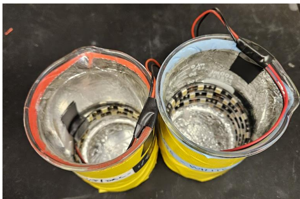
Figure A3.1. Photographs of 400 mL white LED light beakers used for AkCS (left) and polymerizations (right).
