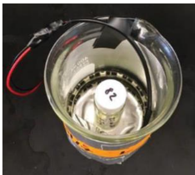
Figure A2.1. 400 mL white light LED beaker photoreactor for polymerizations.
