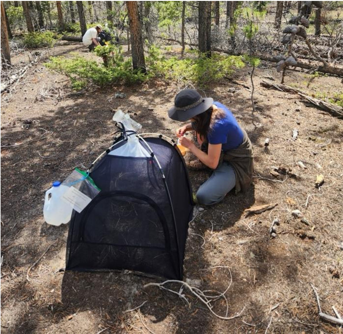
Figure 1. Photo of a BugDorm Soil Insect Emergence Trap (Model BT2013) deployed on the forest floor.
