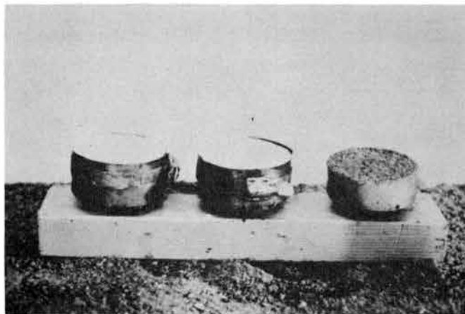
(b) Capping Sample with Plaster of Paris
