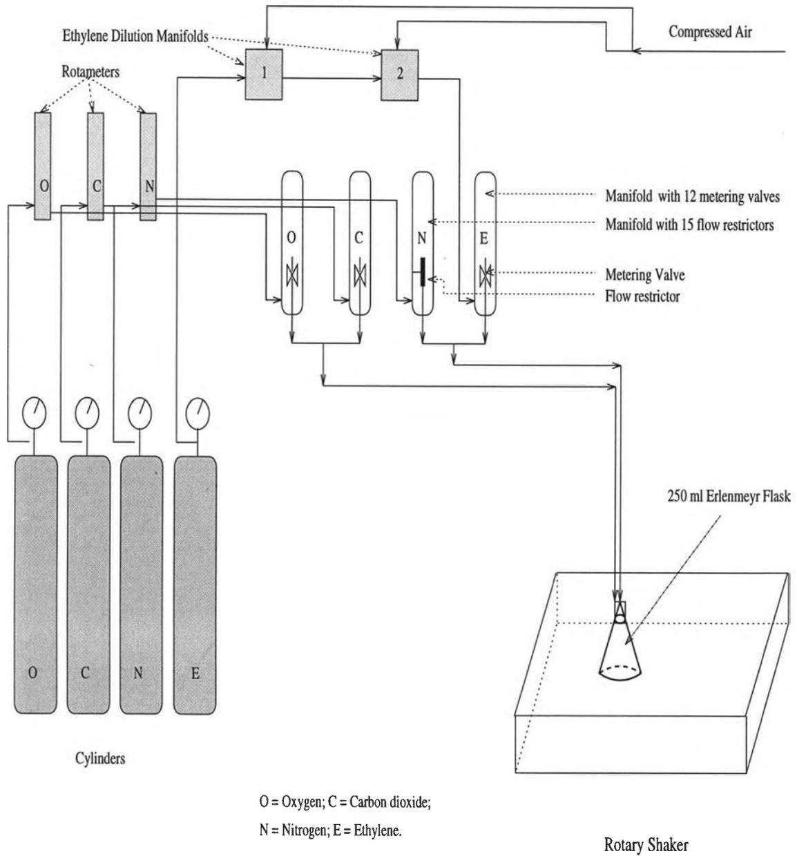
Figure 2.1: Schematic diagram of the gas mixing apparatus.
