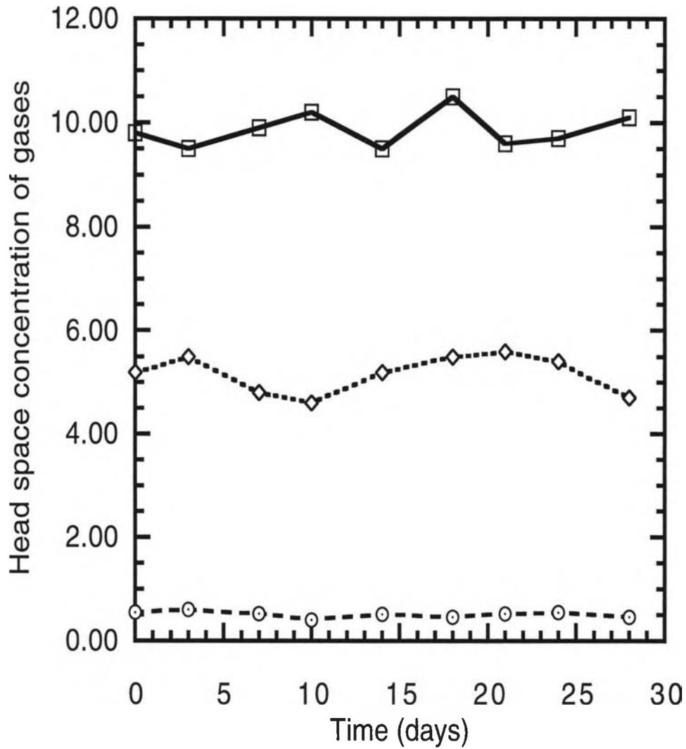
Figure 2.2: Typical concentrations of oxygen, carbon dioxide and ethylene as measured through the out-flow filter unit; the gas apparatus was pre-adjusted to 10% (v/v)  $O_2$ , 0.5% (v/v)  $CO_2$  and 5 ppm ethylene.  $\square$  = oxygen;  $\diamond$  = carbon dioxide;  $\odot$  = ethylene.
