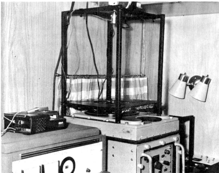
FIGURE 2. View of radar equipment inside trailer. Unit on left houses transmitter, modulator, receiver, and power supplies. Unit in center is PPI indicator with digital display unit for documenting certain data within the field of the time lapse camera. Unit on right is second PPI indicator used for routine viewing and still photographs.
