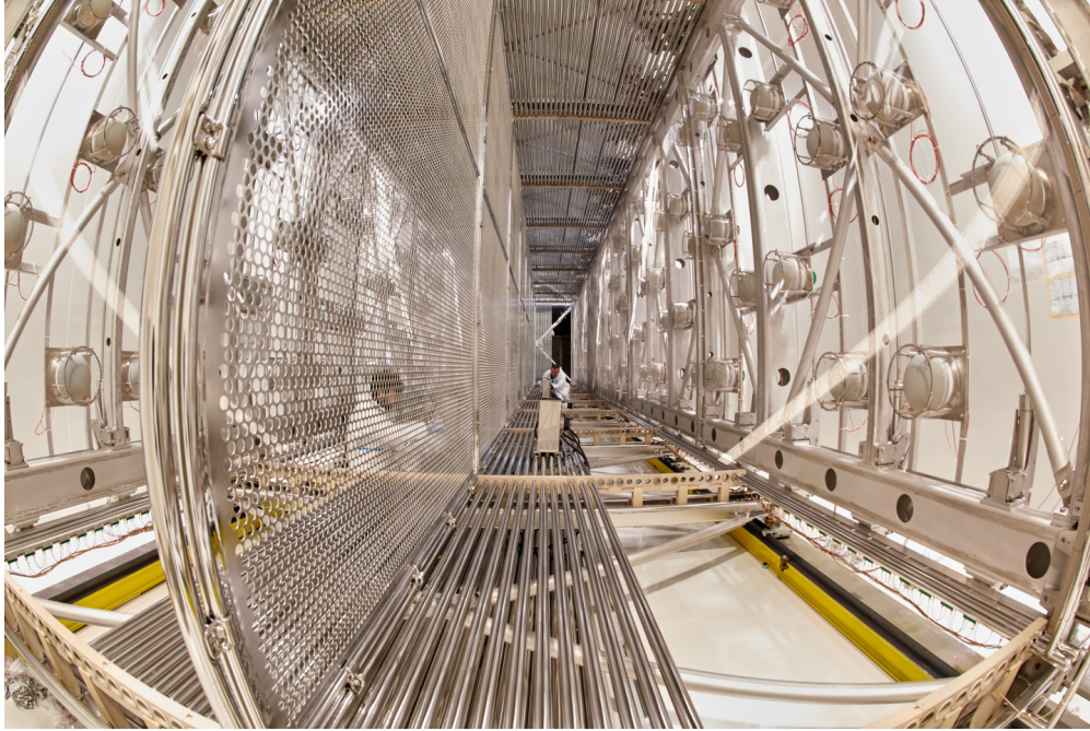
Figure 2.1: Photograph of the inside of one of ICARUS’s cryogenic modules. The vertical metal sheet separating the two time projection chambers is the cathode plane. The longitudinal bars across the top and bottom of the TPC are the field cage. Arrays of photomultiplier tubes are shown at the anode plane of both TPCs. Light flares from the wire planes are also visible at both anode planes. Image is from [5].
