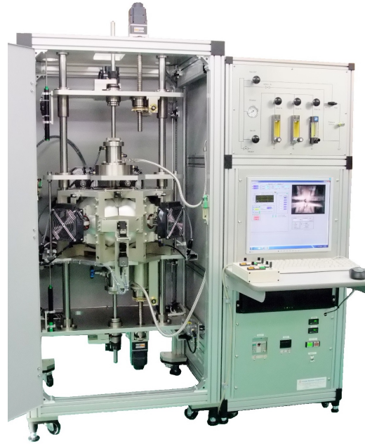
Figure 2.6: Optical float zone furnace (MODEL FZ-T-4000-H-VII-VPO-PC, Crystal Systems Corp.) used for large single-crystal growth of rare-earth silicates.
