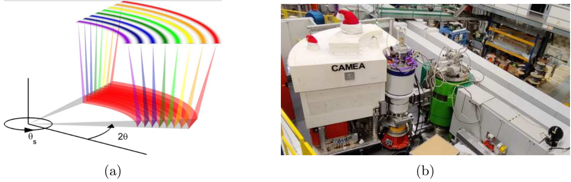
Figure 4.11: (a) Schematic representation of CAMEA's multi-analyzer array, which enables simultaneous detection of eight final energy channels, each covering an azimuthal range of 60^\circ in the horizontal plane. The analyzer-detector bank can be rotated to different 2\theta angles, while the sample angle \theta_s can also be adjusted for alignment and optimized momentum-space coverage. (b) Photograph of the CAMEA spectrometer at the Swiss Spallation Neutron Source (SINQ), showing the experimental setup.
