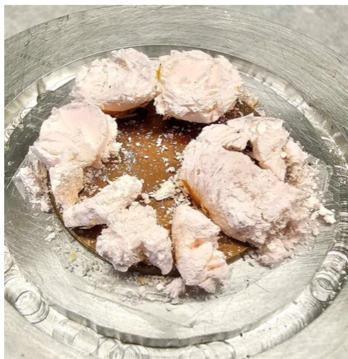
Figure 4.3: Degradation of \text{ErCl}_3 Crystals Upon Air Exposure—Image showing \text{ErCl}_3 single crystals after exposure to ambient air, resulting in significant hydration and decomposition into a fine, white powder. This transformation occurs due to the hygroscopic nature of \text{ErCl}_3 , which rapidly absorbs moisture and forms \text{ErCl}_3 \cdot 6\text{H}_2\text{O} , leading to structural collapse and deliquescence.
