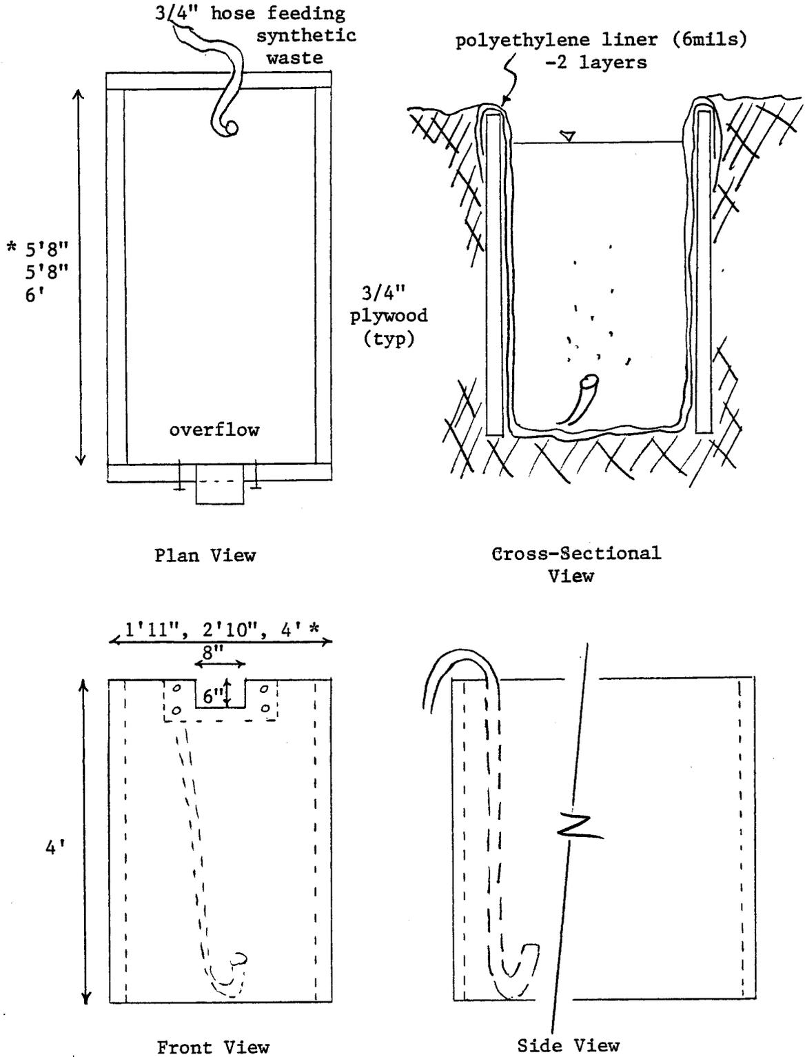
Figure 3-3. Typical Model Pond Construction
