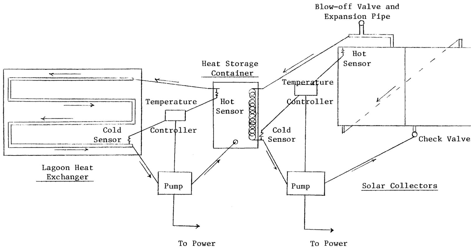
Figure 3-5. Schematic of Equipment Apparatus; System 2.
