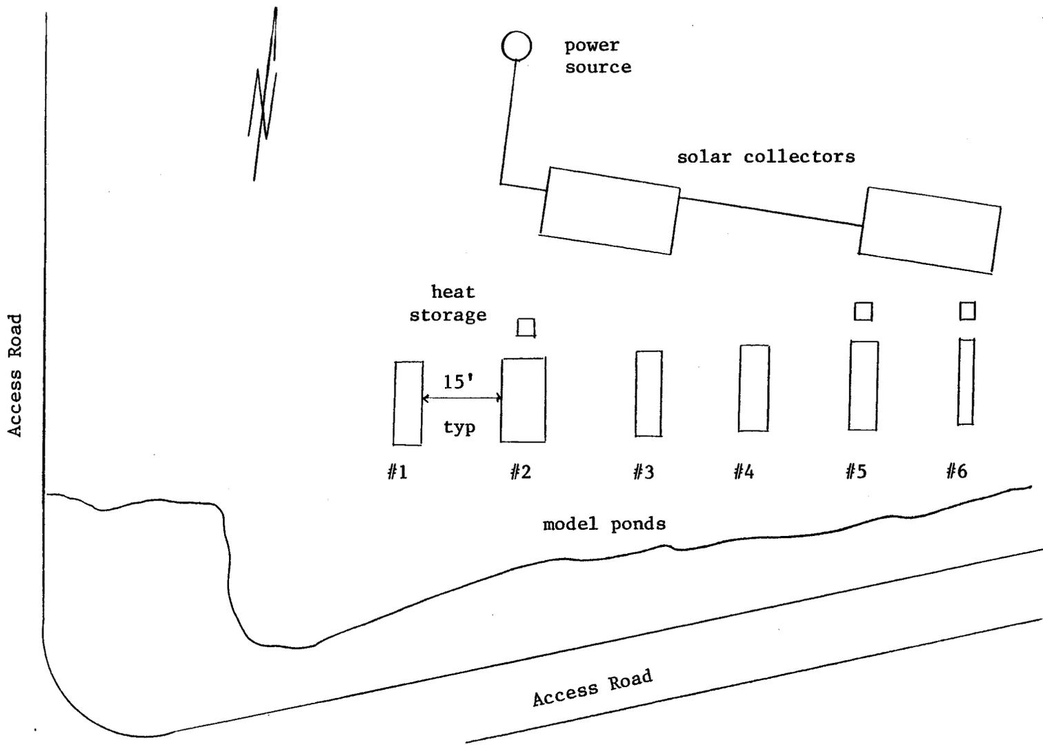
Figure 3-1. Schematic Of Site Layout.
