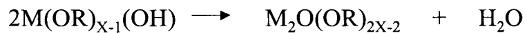
Figure 1.5. Solution chemistry for the sol-gel process using 2-methoxyethanol as reactant and solvent with titanium (IV) butoxide.
