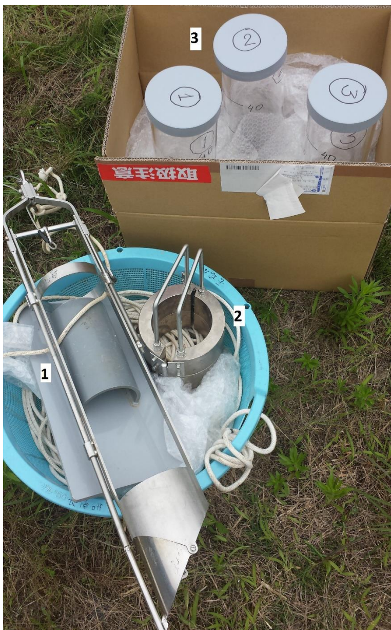
Figure 5. Sediment core sampling device(1), weight(2), and three sample containers(3).
