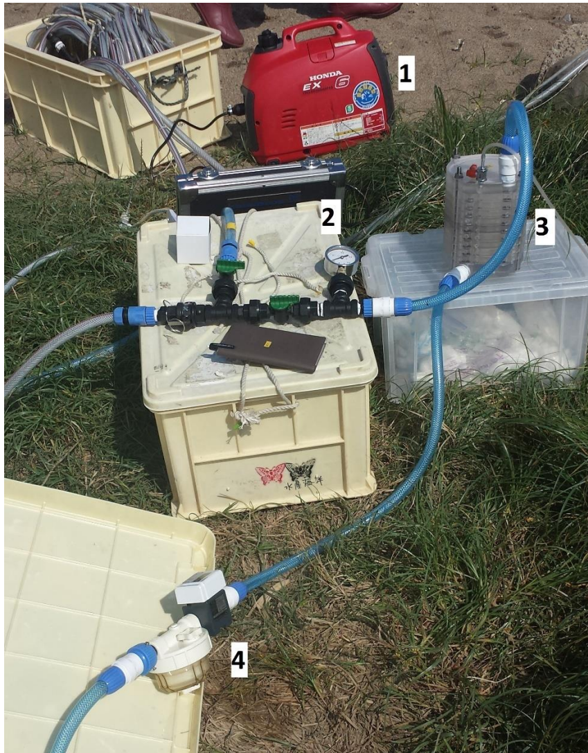
Figure 2. In-situ filtration system showing generator (1), pressure gauge (2), filter stack (3), sorbent cartridge (4).
