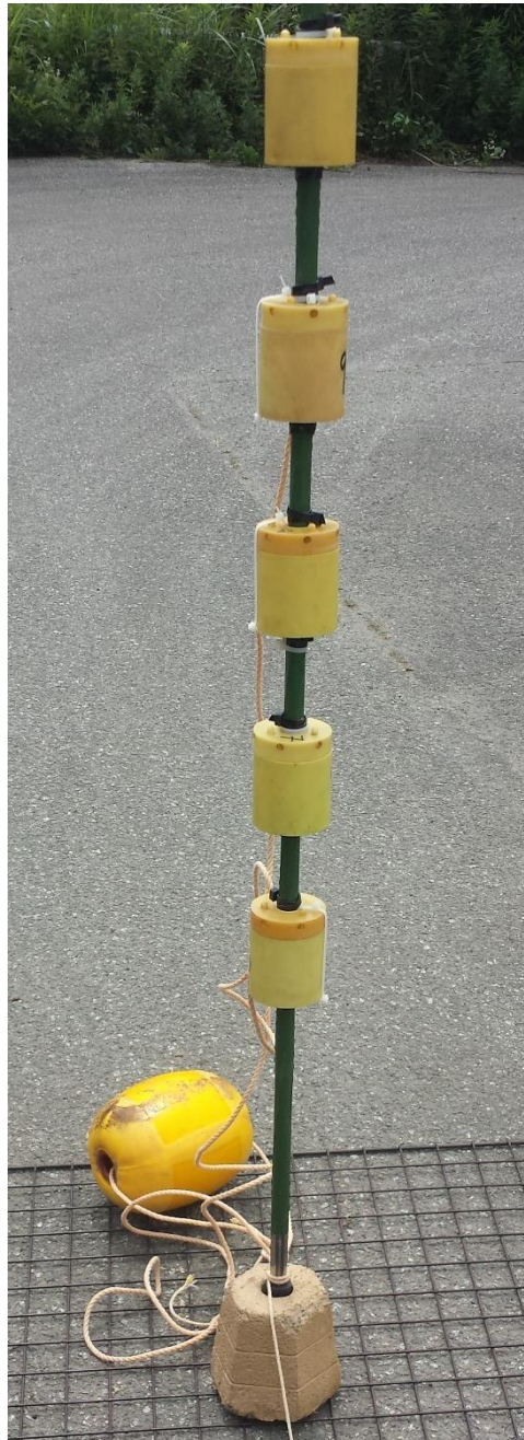
Figure 4. Sediment traps deployed to Inkyozaka and Funasawa 1 ponds.
