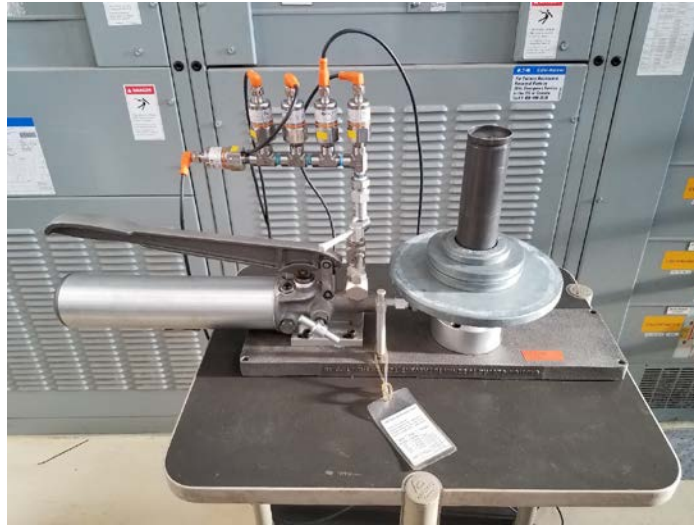
Figure E-1 Calibration of pressure transmitters using a deadweight tester
