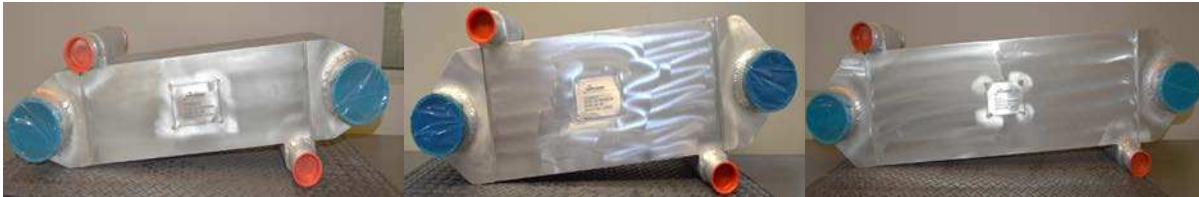
Figure 3-6 Prototype recuperator, economizer, and suction line heat exchanger (Left to Right)
