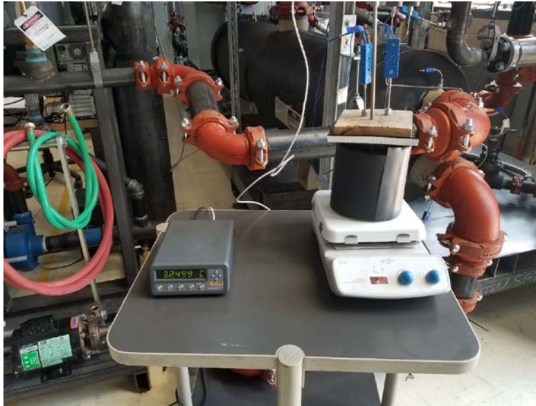
Figure E-2 Calibration of thermocouples using a platinum resistance thermometer
