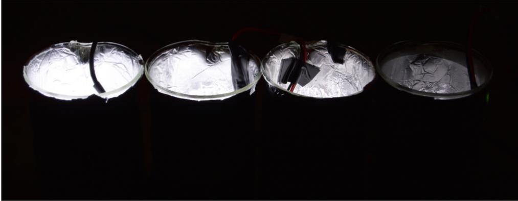
**Figure 4.6.** Picture of the relative light intensities used in this study, controlled by an LED dimmer. From left to right: 100%, 50%, 25%, 5% relative light intensity.
