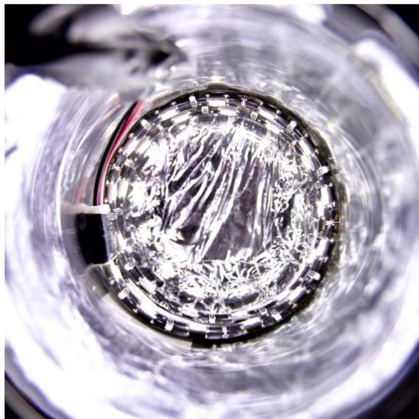
**Figure 4.5.** A picture of the photoreactor used for O-ATRP, constructed from a 400mL beaker lined with 45 cm of white LEDs.
