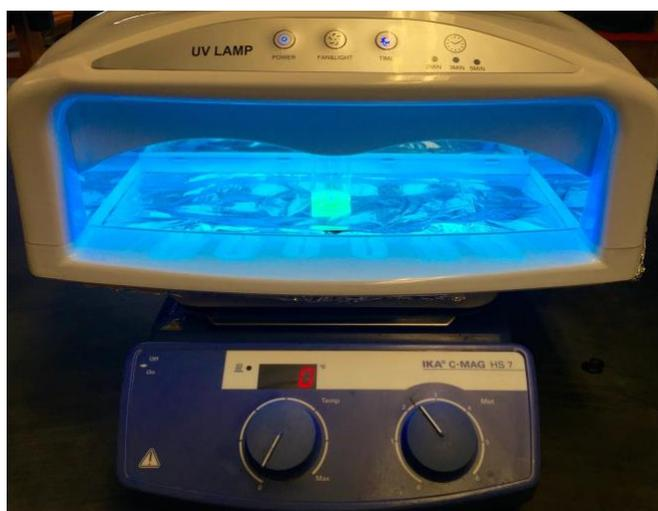
**Figure 3.9.** Photograph of the reaction setup for O-ATRP using UV irradiation.
