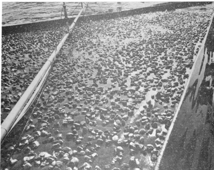
Fig. 14 - The surface detention is shown draining from the gravel surface after the cessation of rainfall.
