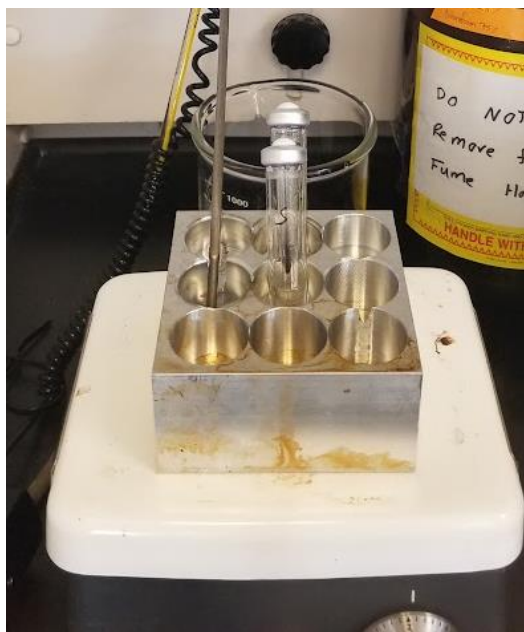
Figure 6.3. Picture of the 180 °C treatment setup, showing the two sample vials immersed in hot silicone oil, with a thermometer constantly monitoring the temperature.
