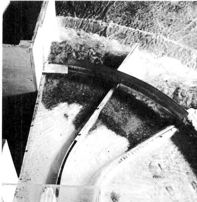
Fig. 19. Recommended structure Sluicing at Q \approx 15 c.m.s.
