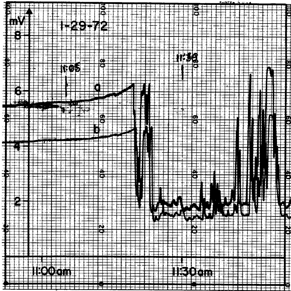
Fig. 3. Sample section of pyranometer chart output (a) incoming radiation (b) reflected radiation Cumulus clouds occurred after 11:19 a.m.
