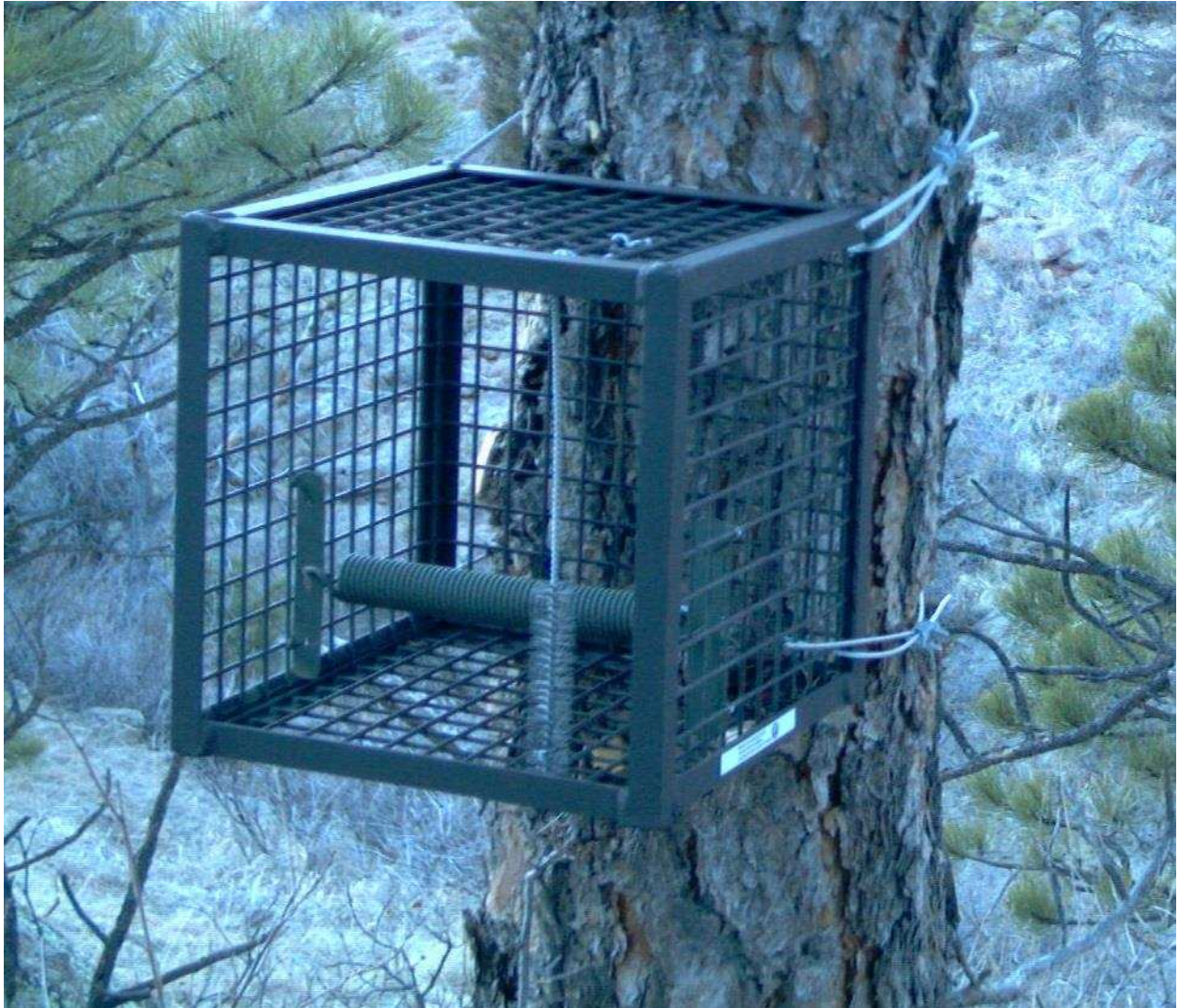
Figure 4. One of the metal-mesh-cube hair-snaring devices tested on the Front Range, Colorado (2012). A spring and a barrel cleaning brush were attached to snag hair. Bait was wired in the back and replenished approximately once per week. No hair samples were obtained via this device.
