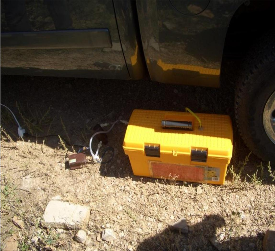
**Figure 4.** Homemade anesthetic box. A plastic toolbox was modified by drilling holes, inserting plastic tubing attached to a hollow cylinder for cotton balls infused with inhalant anesthetic, which was circulated by a small air pump attached to the alternate side of the cylinder. Power was provided through the cigarette lighter attachment of the vehicle. The box could accommodate the entire wire trap so rodent handling prior to anesthetization was minimized.
