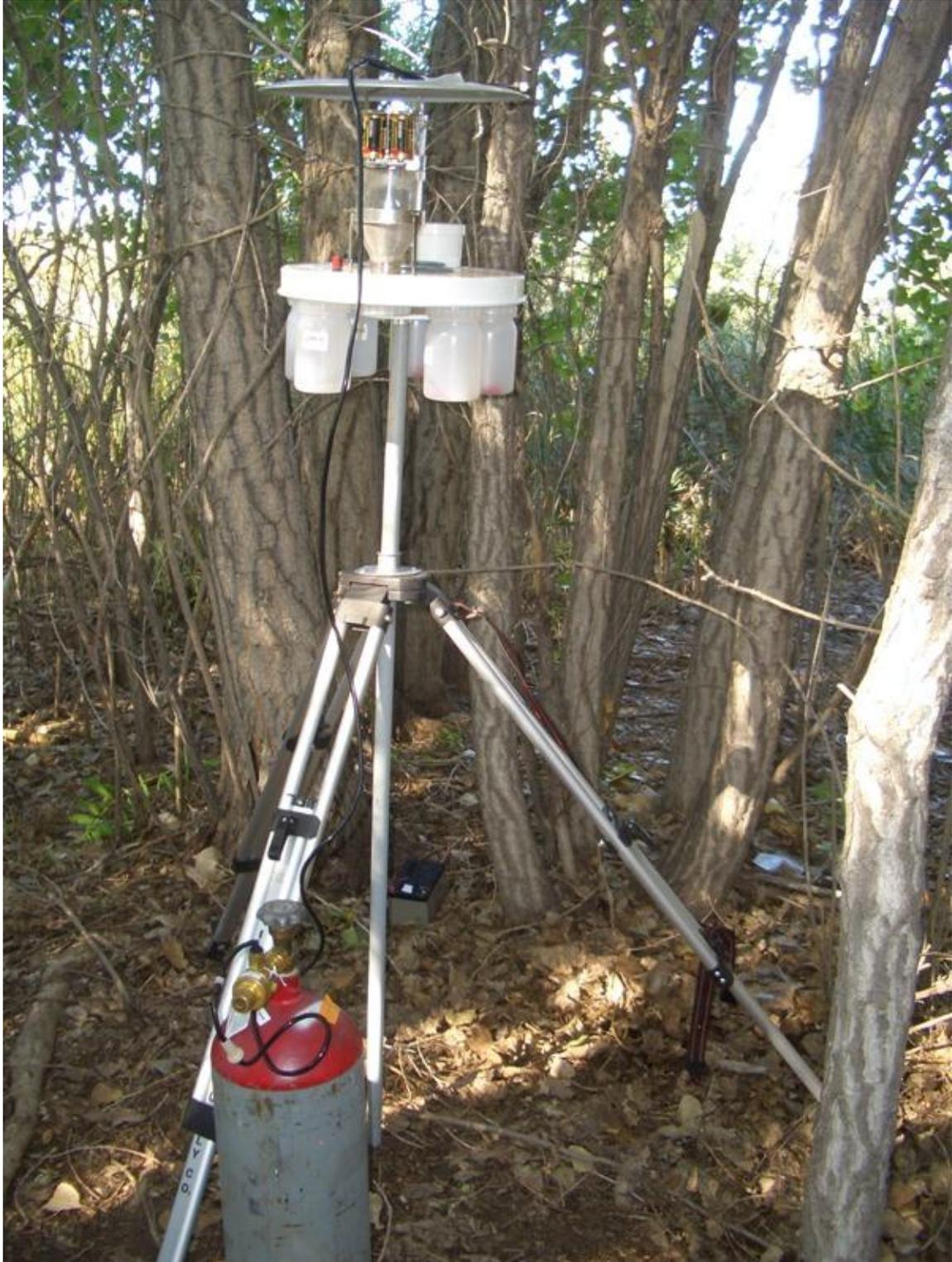
**Figure 11.** Rotator bottle trap assembled. Compressed air bottle contains carbon dioxide.
