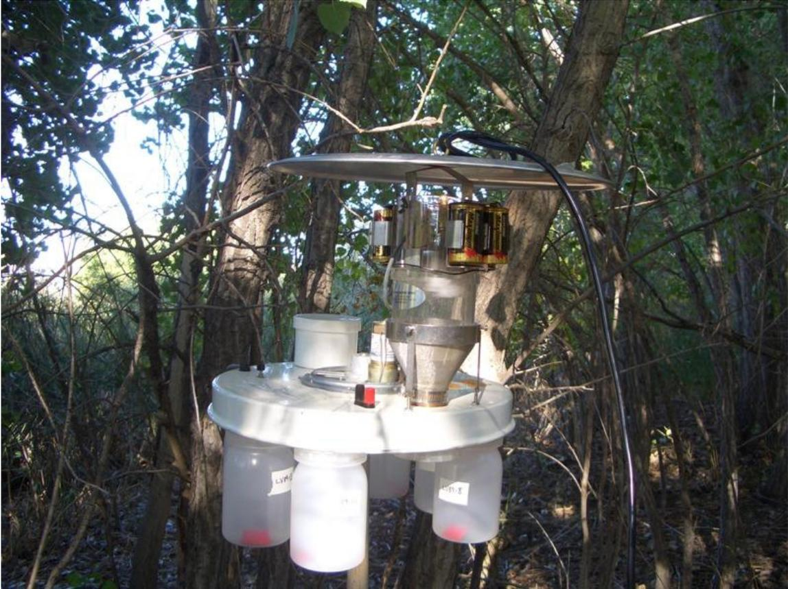
**Figure 13.** Close-up of bottle rotator with light attached to the top.
