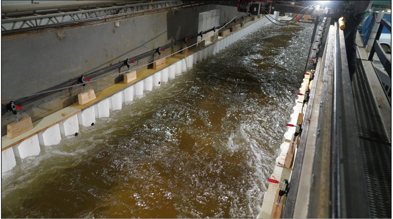
Fig. C3. System A tangent wall configuration
