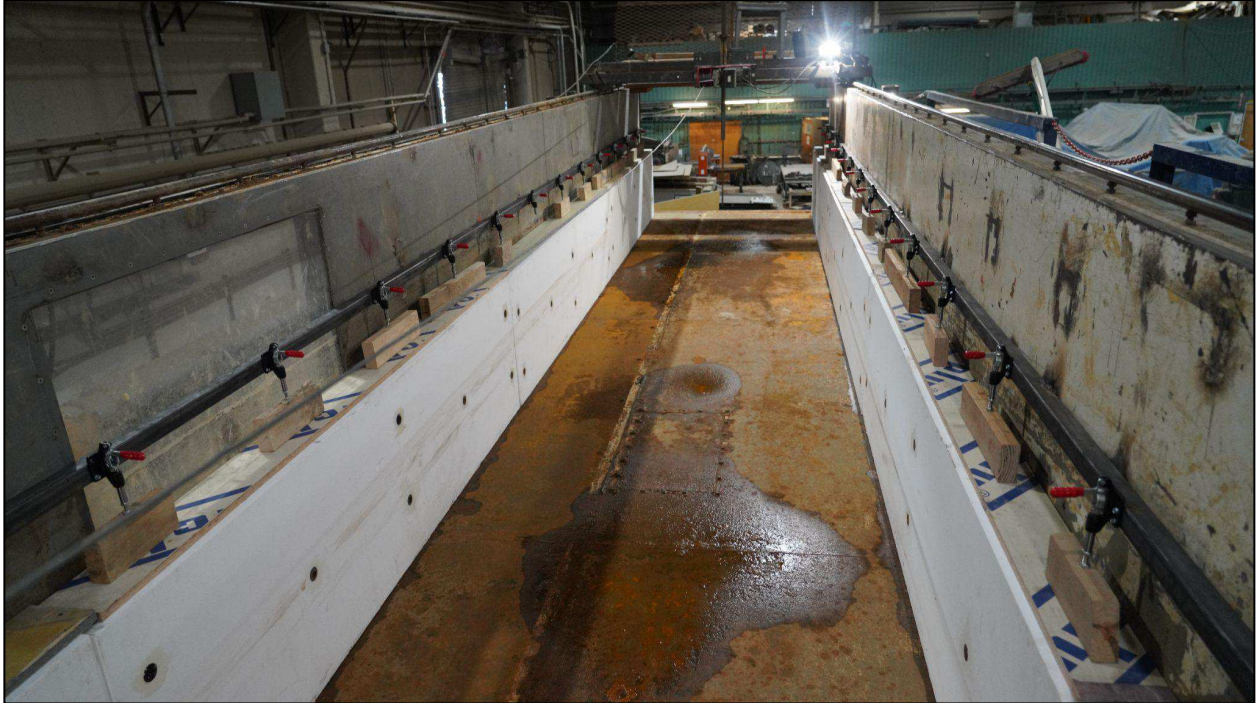
Fig. C1. System A smooth wall configuration
