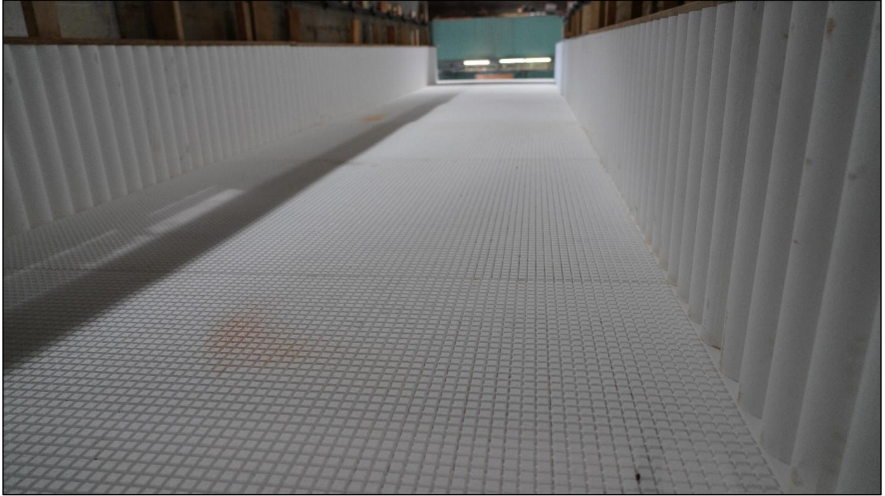
Fig. C11. System D tangent wall configuration
