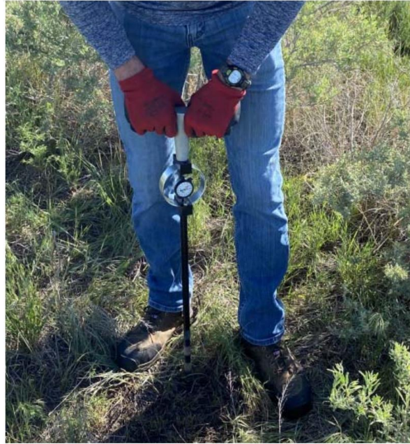
Figure A.3. Photo of cone penetrometer during insertion into the surficial soil as a proxy measurement for surficial soil strength. From Bindner (2020).
