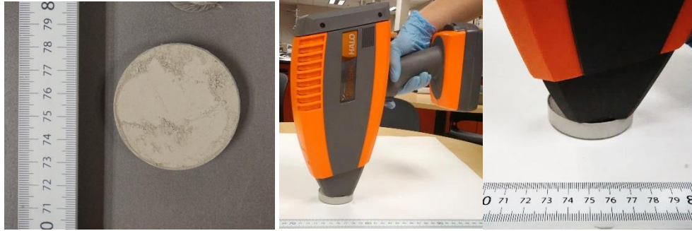
Figure 3.4. Images of (a) prepared test specimen, (b) spectrometer, and (c) close up of the spectrometer in contact with a test specimen.
