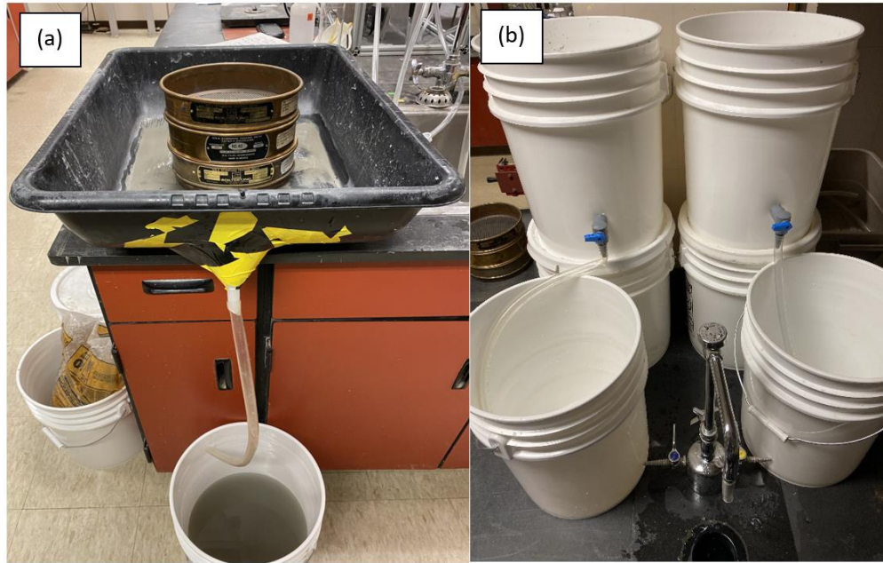
Figure A.13. Photographs of (a) wet sieving setup used to achieve whole tailings sub-samples with varying sand contents and (b) buckets used to mix the fine fraction of tailings (viz. passing No. 200 sieve) with water and allowed to settle for general separation of silt and clay sized particles. After the settling period, the bucket valves were opened, and clay dominated portions were drained. Both clay and silt dominated portions were then dried in forced-air ovens at 110°C.
