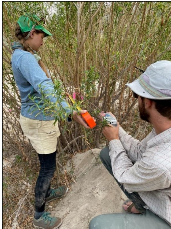
Figure 2.4. Measuring the force-displacement relationship for a baccharis plant to calculate flexural rigidity.
