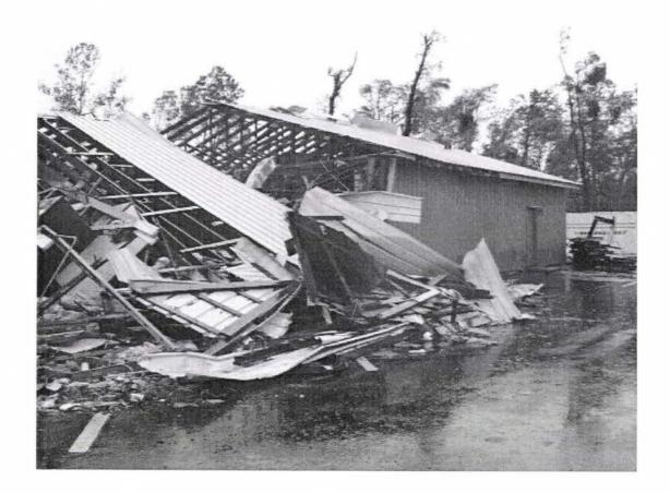
Figure 2.3 – Collapse of a wood frame (metal clad) building
