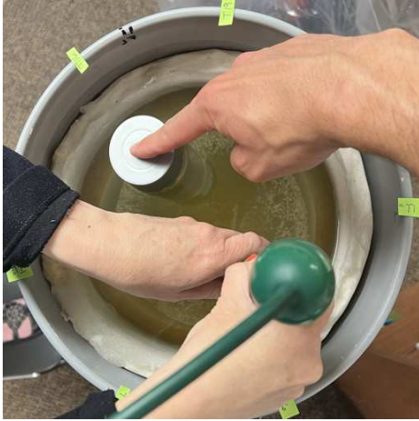
(a) The glass bottle in the water-filled tank near transducer 16 and the balloon near transducer 6.
