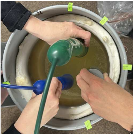
(c) The glass bottle in the water-filled tank near transducer three and the balloons near transducers 9 and 19.
