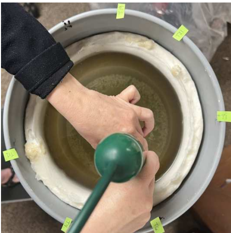
(e) One balloon in the water-filled tank near transducer 6.
