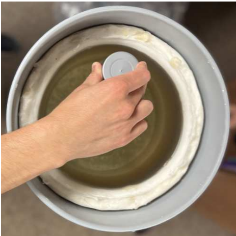
(c) The glass bottle in the water-filled tank near transducer 19.
