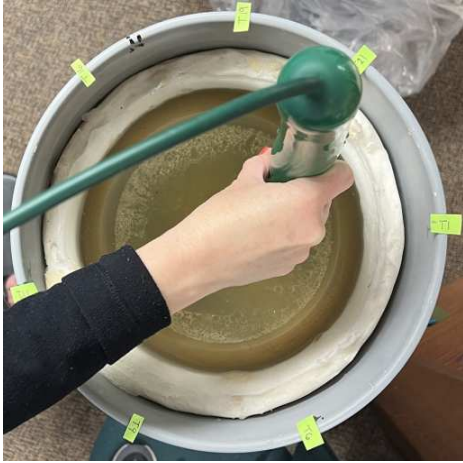
(a) One balloon in the water-filled tank near transducer 21.
