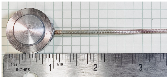
Fig. 2. Final assembled transducer.
