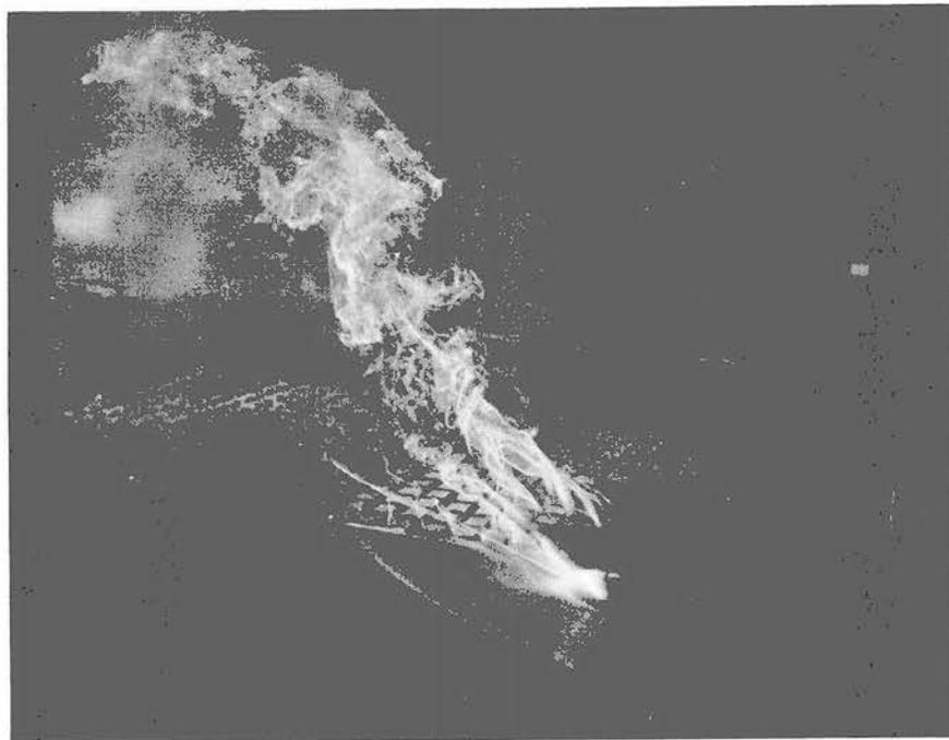
Fig. 5.6 Photograph - Stable approach flow over unstable rough heat island - ground smoke source at left side.
