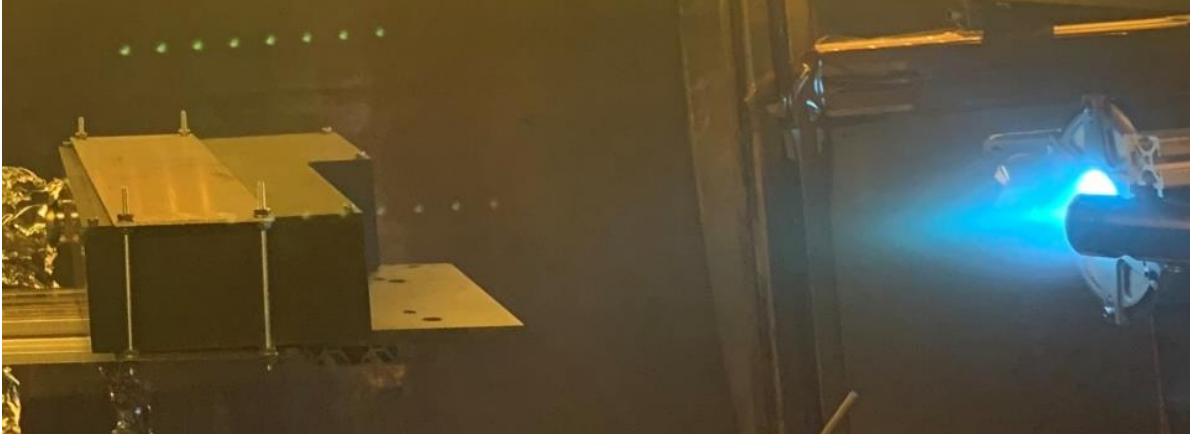
Figure 7: Photograph of the BHT-200 HET operated on xenon with a channel-aligned EVADER probe mounted on an in-vacuum motion stage.
