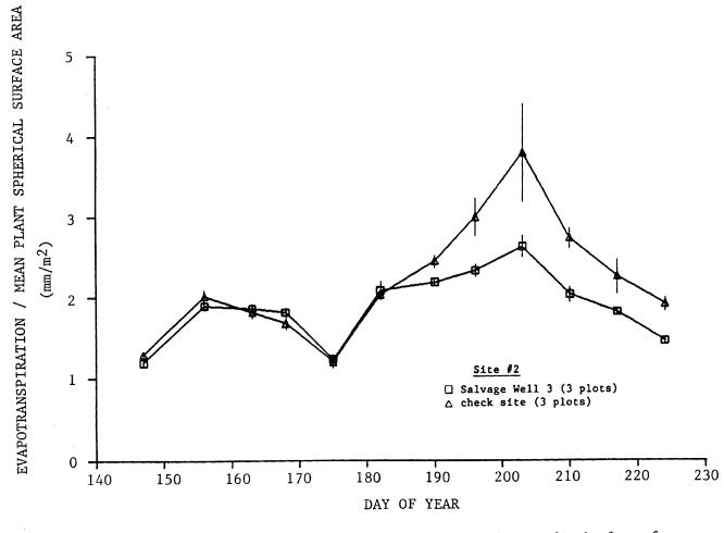
Figure 4.16 Mean evapotranspiration per mean plant spherical surface area + standard error. (Greasewood plots, Salvage Well 3 and check sites, 1986)
