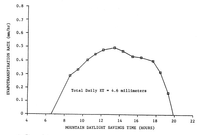
Figure 3.2 Diurnal evapotranspiration measured with a portable chamber. (Rabbitbrush #1, USBR Lysimeter site, 28 July 1986)
