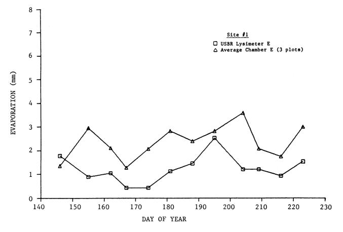
Figure 4.7 Evaporation comparison of USBR lysimeter versus chamber measurements. (Bare Soil plots, USBR Lysimeter site, 1986)
