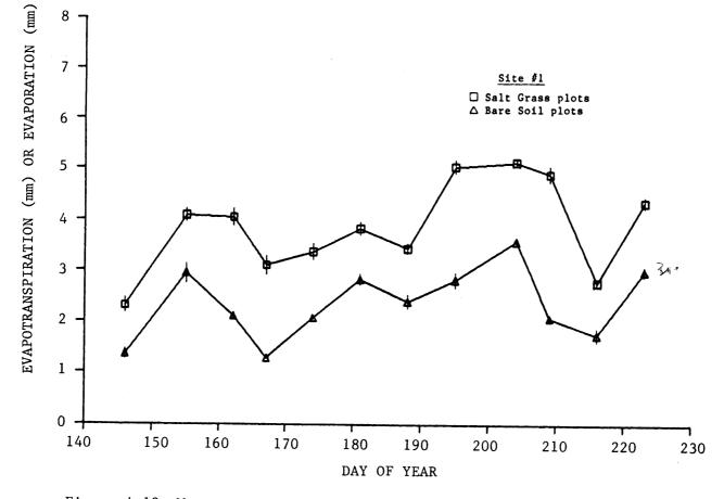
Figure 4.12 Mean evapotranspiration <u>+</u> standard error (Salt Grass plots) and mean evaporation <u>+</u> standard error (Bare Soil plots). (USBR Lysimeter site, 1986)
