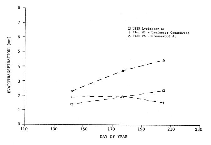
Figure 4.1 Evapotranspiration comparison of USBR lysimeter versus chamber measurements. (Greasewood plots, USBR Lysimeter site, 1985)
