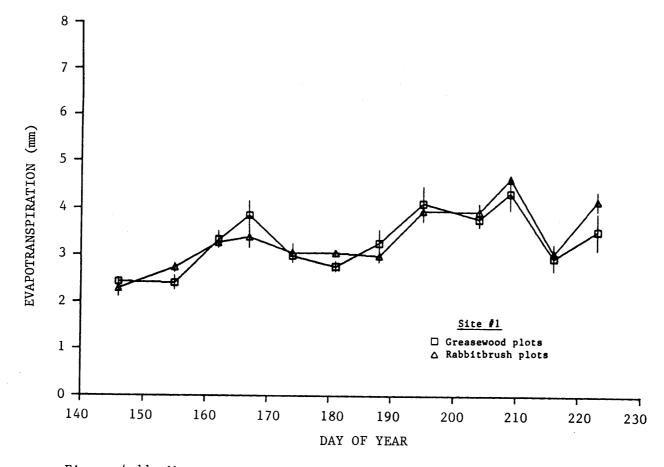
Figure 4.11 Mean evapotranspiration + standard error. (Greasewood and Rabbitbrush plots, USBR Lysimeter site, 1986)
