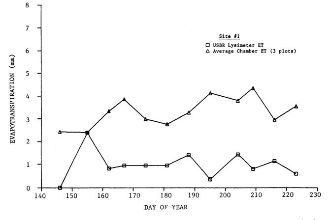
Figure 4.5 Evapotranspiration comparison of USBR lysimeter versus chamber measurements. (Greasewood plots, USBR Lysimeter site, 1986)
