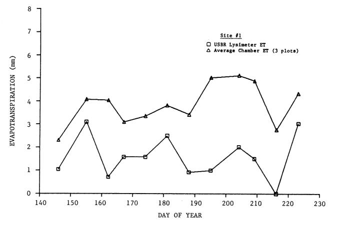
Figure 4.8 Evapotranspiration comparison of USBR lysimeter versus chamber measurements. (Salt Grass plots, USBR Lysimeter site, 1986)
