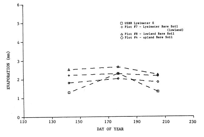
Figure 4.4 Evaporation comparison of USBR lysimeter versus chamber measurements. (Bare Soil plots, USBR Lysimeter site, 1985)
