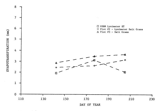
Figure 4.3 Evapotranspiration comparison of USBR lysimeter versus chamber measurements. (Salt Grass plots, USBR Lysimeter site, 1985)
