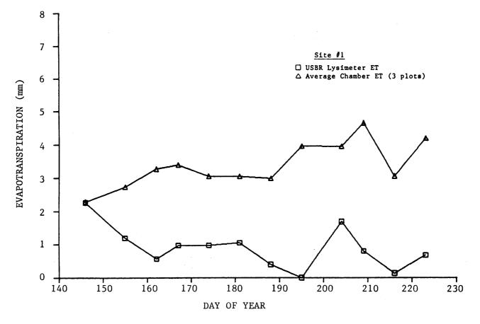
Figure 4.6 Evapotranspiration comparison of USBR lysimeter versus chamber measurements. (Rabbitbrush plots, USBR Lysimeter site, 1986)
