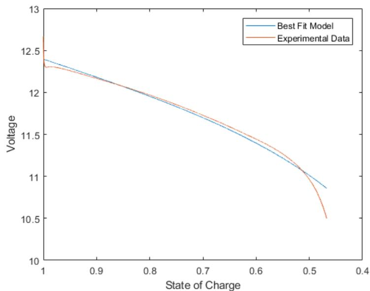
**Figure 2.10:** Identification of Lead battery at 5.0 A discharge - Data Set 1
