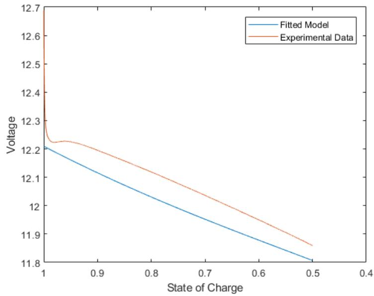
**Figure 2.34:** Prediction of 10.0 A discharge with parameters of 7.5 A
