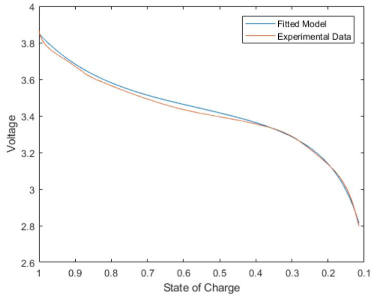
**Figure 2.16:** Prediction of 0.4 A discharge with parameters of 0.3 A
