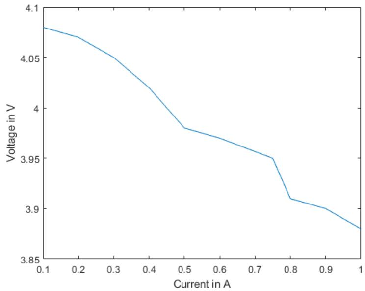
**Figure 3.15:** 1000 mAh Lithium-ion Battery Starting Voltages
