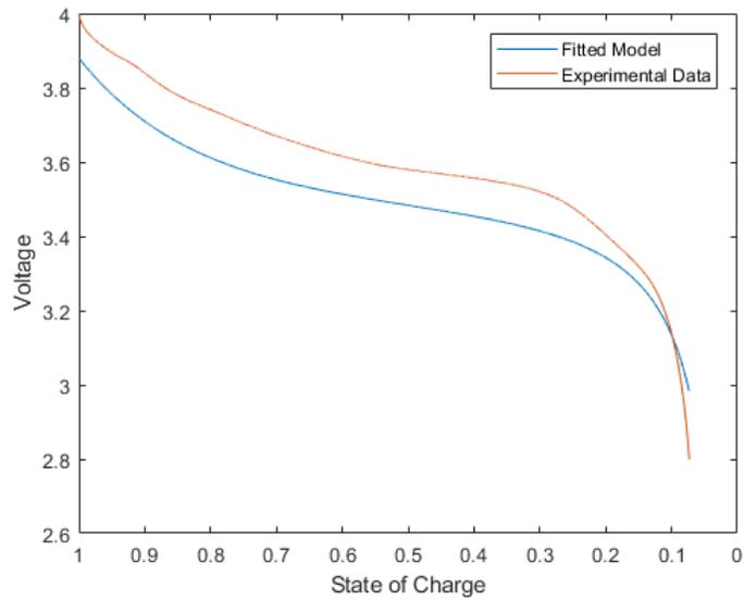
**Figure 2.17:** Prediction of 0.2 A discharge with parameters of 0.4 A
