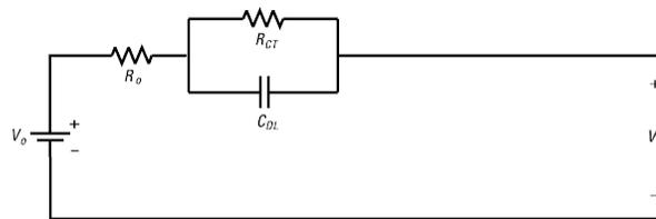
**Figure 1.1:** Basic Equivalent Circuit Model
