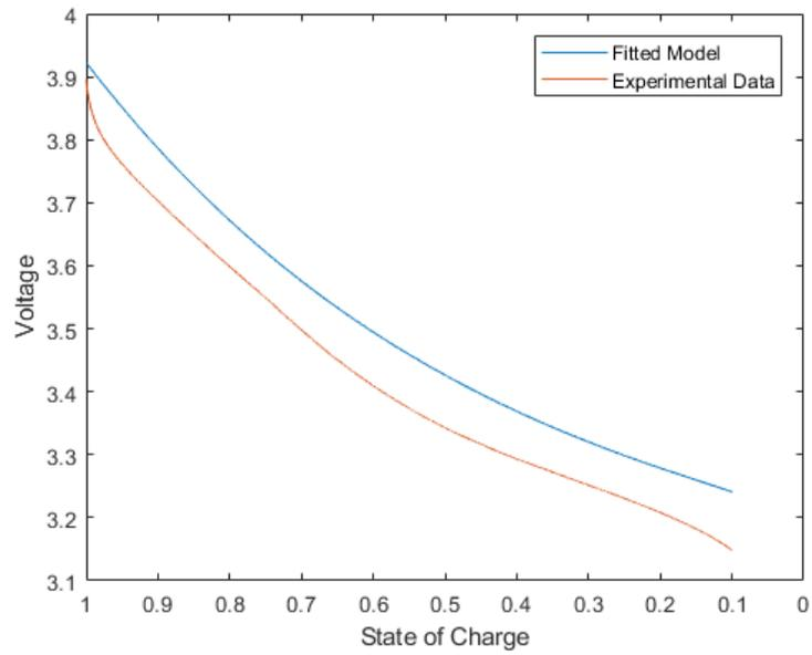
**Figure 2.21:** Prediction of 0.5 A discharge with parameters of 0.75 A
