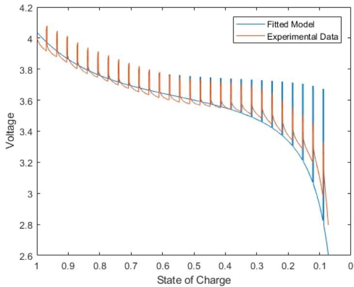
**Figure 2.42:** Predicting 6000 mAh Battery with varying current of 1.5 A
