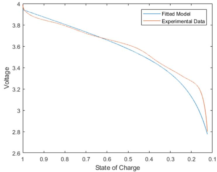
**Figure 2.25:** Prediction of 1.2 A discharge with parameters of 0.9 A
