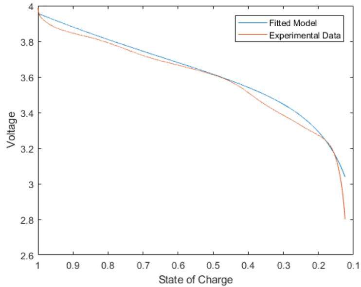
**Figure 2.30:** Prediction of 1.20 A discharge with parameters of 1.50 A
