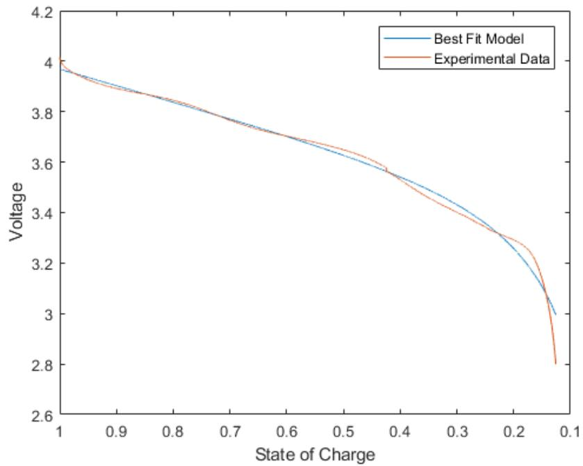
**Figure 2.7:** Identification of 6000mAh Lithium-ion battery at 0.9 A discharge - Data Set 1
