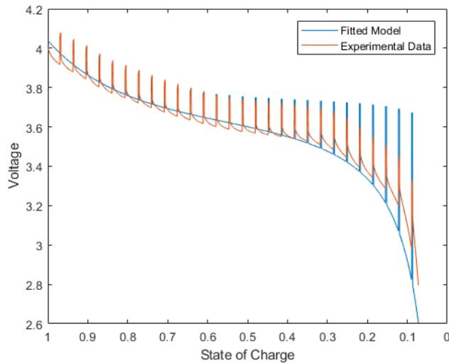
**Figure 2.38:** Predicting 400 mAh Battery with varying current of 0.4 A
