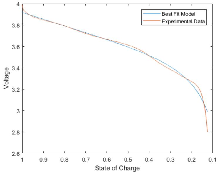
**Figure 2.8:** Identification of 6000mAh Lithium-ion battery at 1.20 A discharge - Data Set 1
