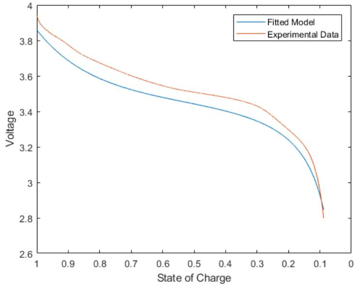
**Figure 2.18:** Prediction of 0.3 A discharge with parameters of 0.4 A
