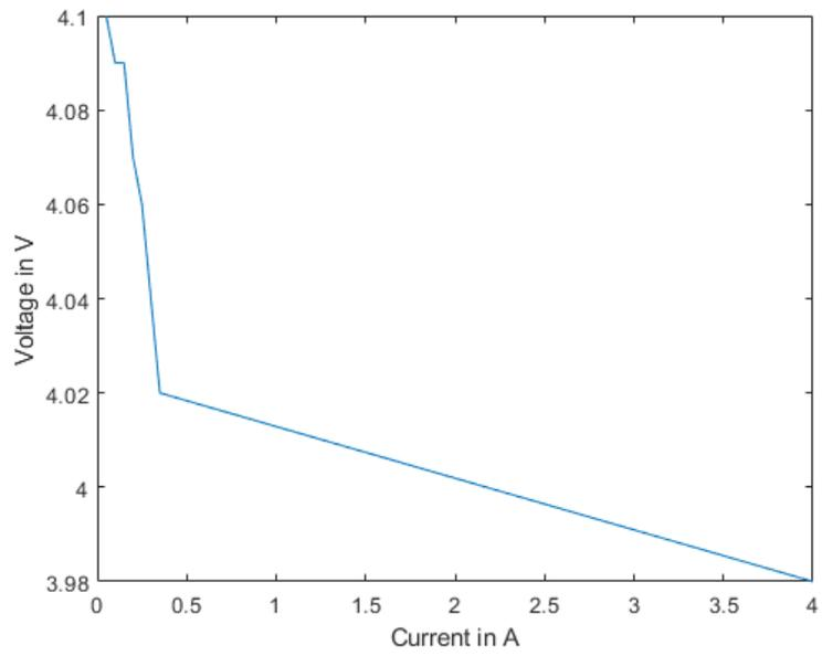
**Figure 3.14:** 400 mAh Lithium-ion Battery Starting Voltages
