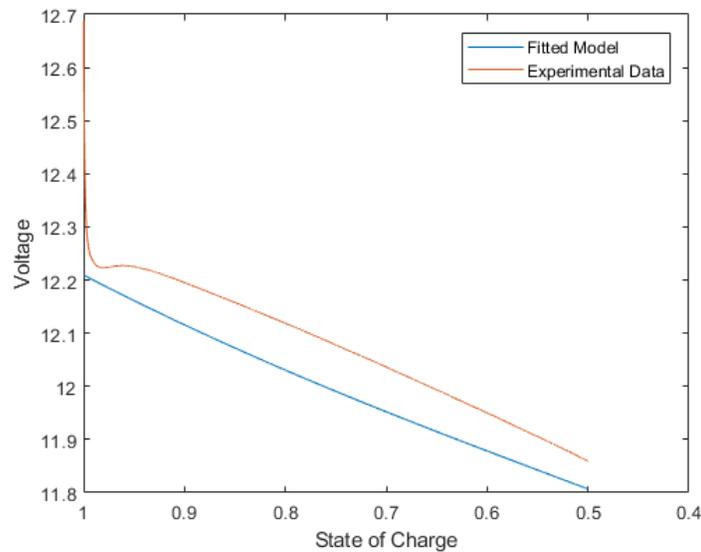
**Figure 2.32:** Prediction of 7.50 A discharge with parameters of 10.0 A
