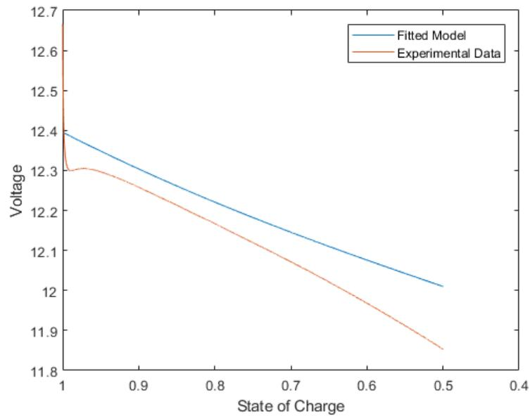
**Figure 2.33:** Prediction of 5.0 A discharge with parameters of 7.5 A
