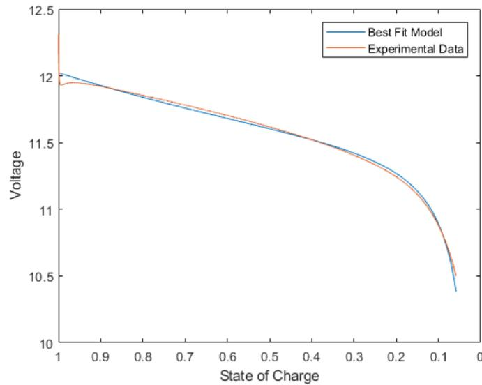
**Figure 2.12:** Identification of Lead battery at 10.0 A discharge - Data Set 1
