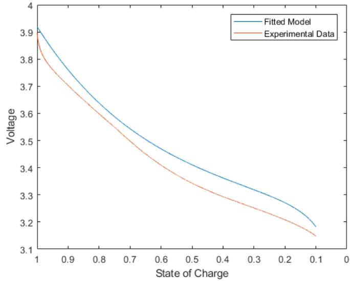
**Figure 2.23:** Prediction of 0.5 A discharge with parameters of 1 A
