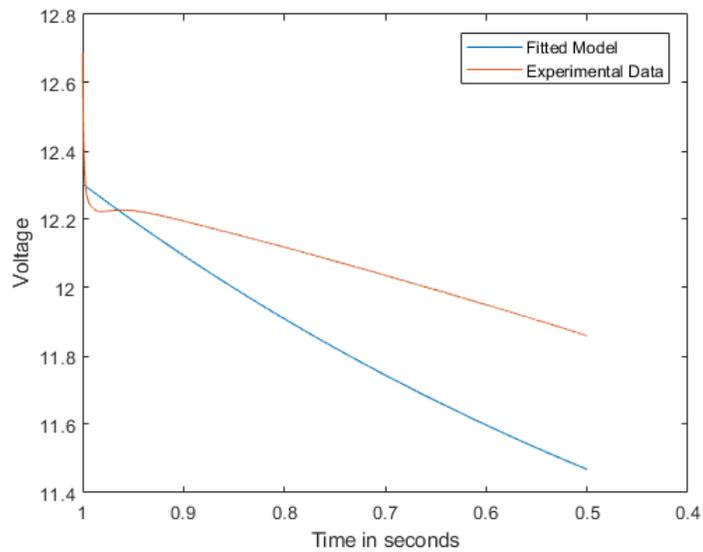
**Figure 2.35:** Prediction of 7.5 A discharge with parameters of 5.0 A
