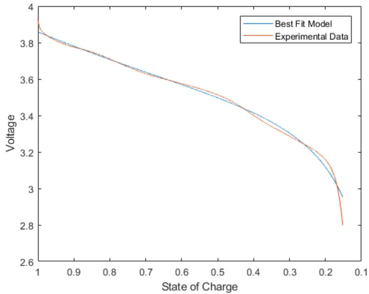
**Figure 2.9:** Identification of 6000mAh Lithium-ion battery at 1.50 A discharge - Data Set 1
