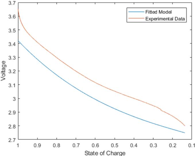
**Figure 3.5:** Prediction of 1.0 A using parameters of 0.75 A discharge
