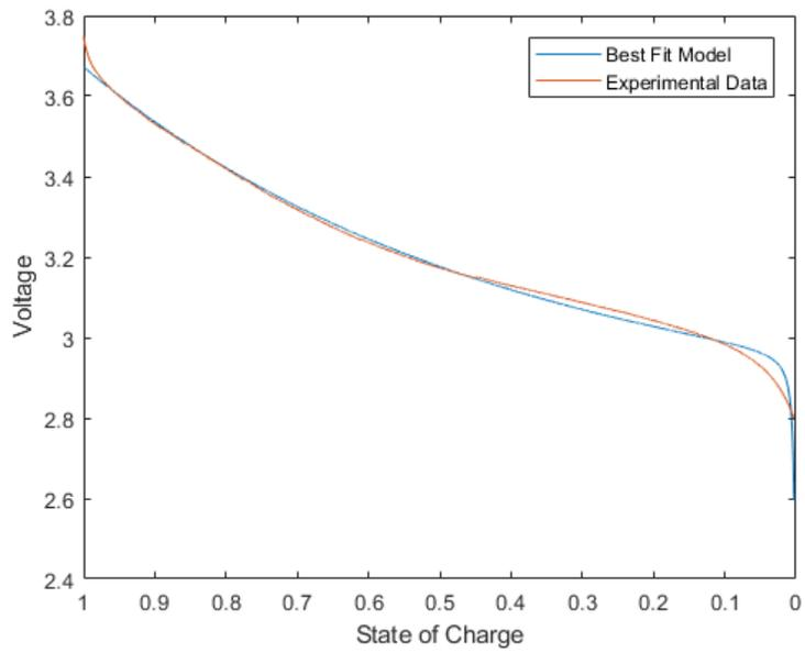
**Figure 2.5:** Identification of 1000mAh Lithium-ion battery at 0.75 A discharge - Data Set 1
