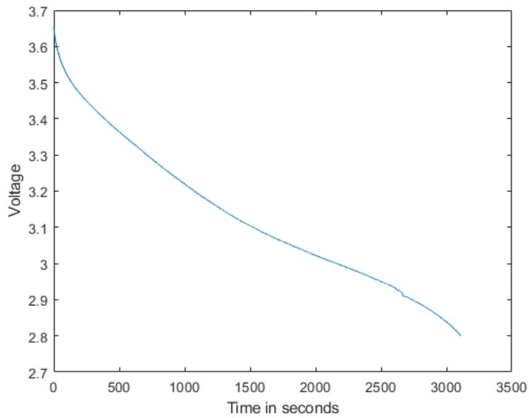
**Figure 3.3:** 1.0 A discharge of the 1000 mAh battery
