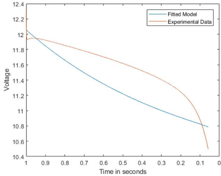
**Figure 2.36:** Prediction of 10.0 A discharge with parameters of 5.0 A
