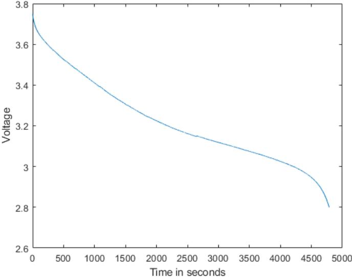
**Figure 3.6:** Discharge of 1000 mAh battery with 0.75 A
