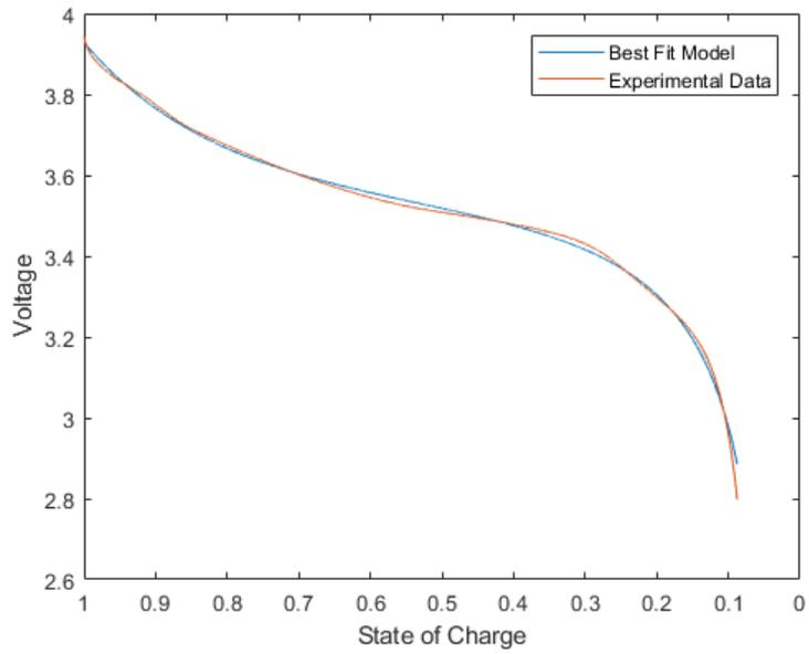
**Figure 2.2:** Identification of 400mAh Lithium-ion battery at 0.3 A discharge - Data Set 1
