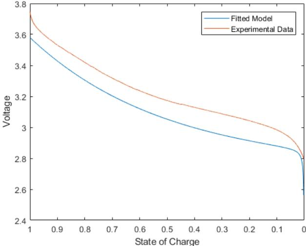
Figure 3.10: 0.5 A discharge parameters used to predict the discharge behaviour of 0.75 A discharge
