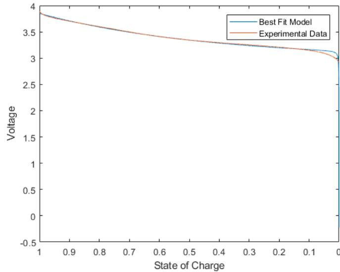
**Figure 2.4:** Identification of 1000mAh Lithium-ion battery at 0.5 A discharge - Data Set 1
