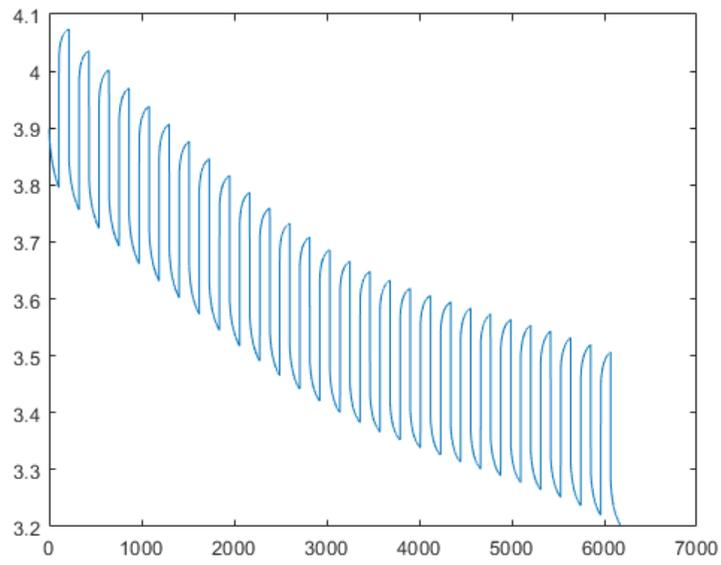
**Figure 2.39:** 1000 mAh Battery with varying current of 1.0 A
