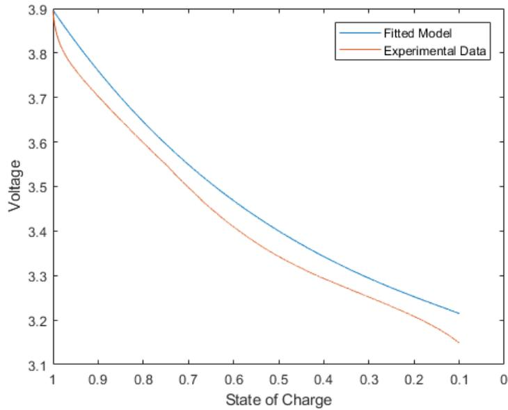
**Figure 3.13:** 0.75 A discharge parameters used to predict the discharge behaviour of 0.5 A discharge with  $E_a$  factor
