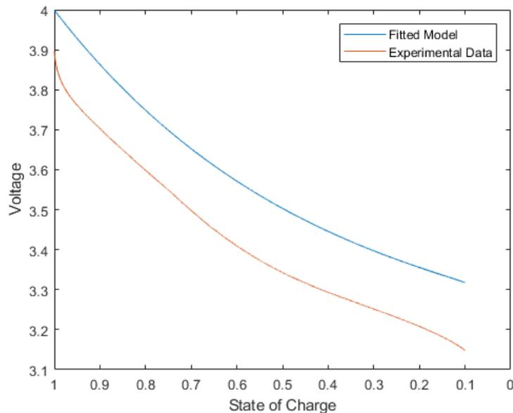
**Figure 3.12:** 0.75 A discharge parameters used to predict the discharge behaviour of 0.5 A discharge
