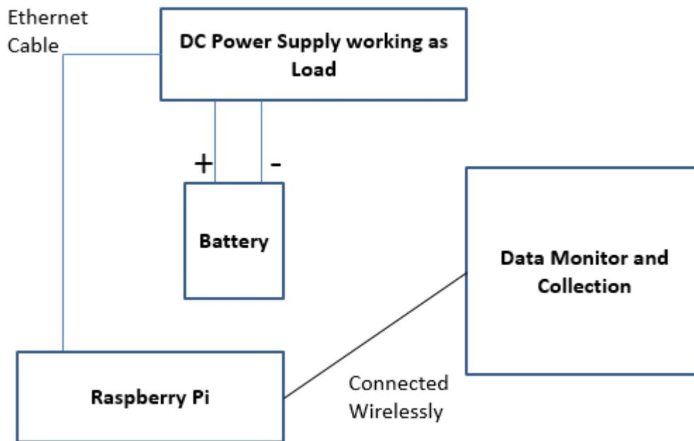
**Figure 1.2:** The Discharging Block Diagram
