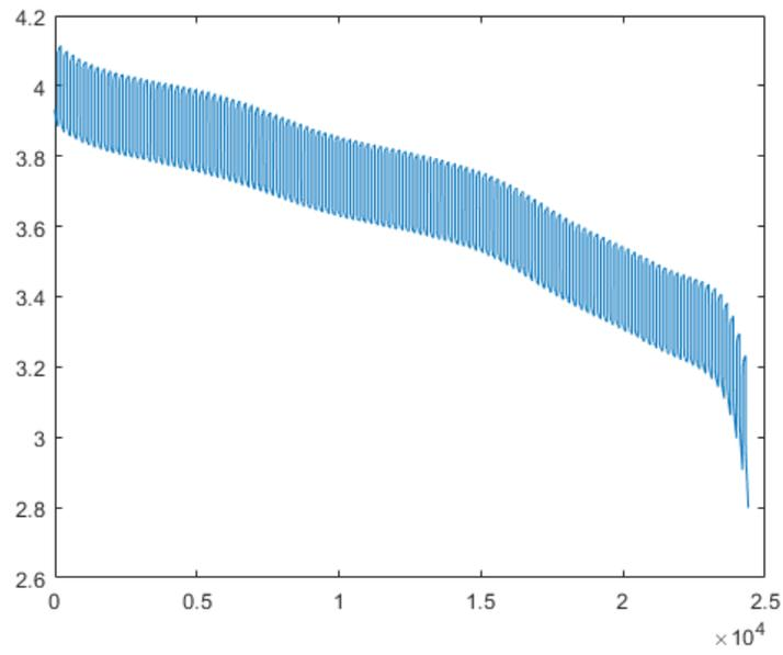
**Figure 2.41:** 6000 mAh Battery with varying current of 1.5 A
