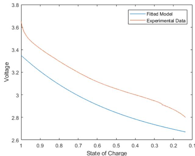
**Figure 3.1:** Prediction of 1.0 A discharge with parameters of 0.50 A
