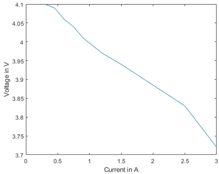
**Figure 3.16:** 6000 mAh Lithium-ion Battery Starting Voltages
