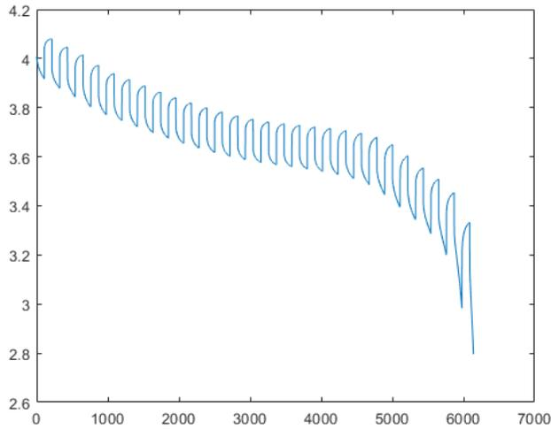
**Figure 2.37:** 400 mAh Battery with varying current of 0.4 A
