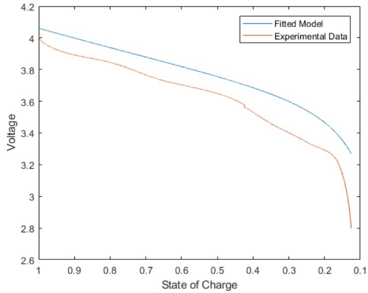
**Figure 2.27:** Prediction of 0.9 A discharge with parameters of 1.20 A
