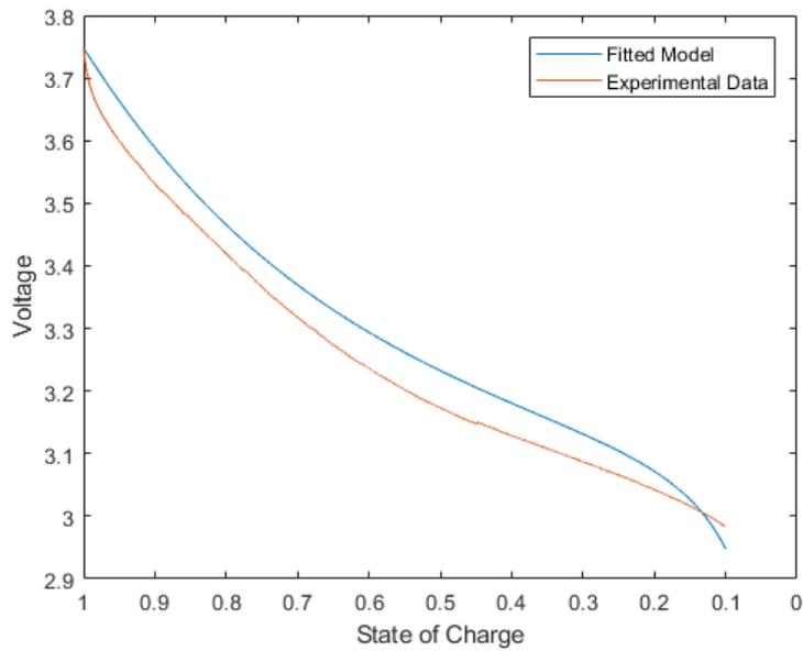
**Figure 2.24:** Prediction of 0.75 A discharge with parameters of 1.0 A
