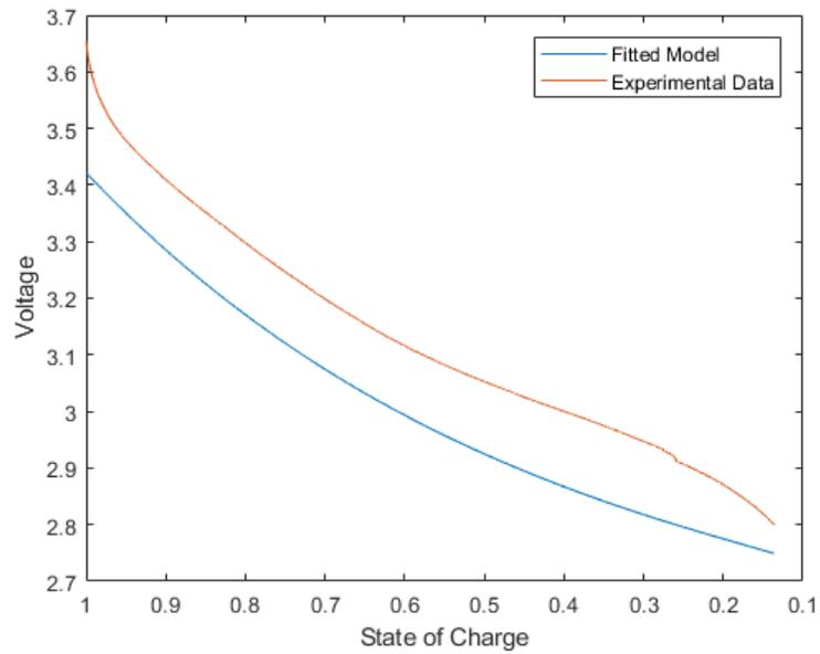
**Figure 2.22:** Prediction of 1.0 A discharge with parameters of 0.75 A
