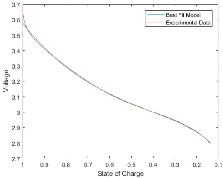
**Figure 2.6:** Identification of 1000mAh Lithium-ion battery at 1.0 A discharge - Data Set 1
