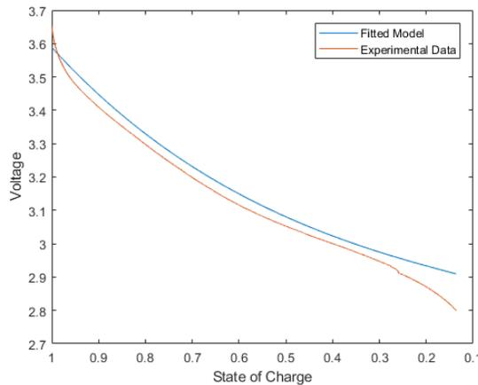
**Figure 3.4:** Reduced error after adjustment of the starting voltage
