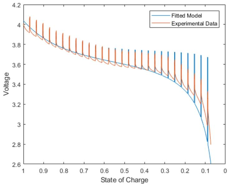
**Figure 2.40:** Predicting 1000 mAh Battery with varying current of 1.0 A
