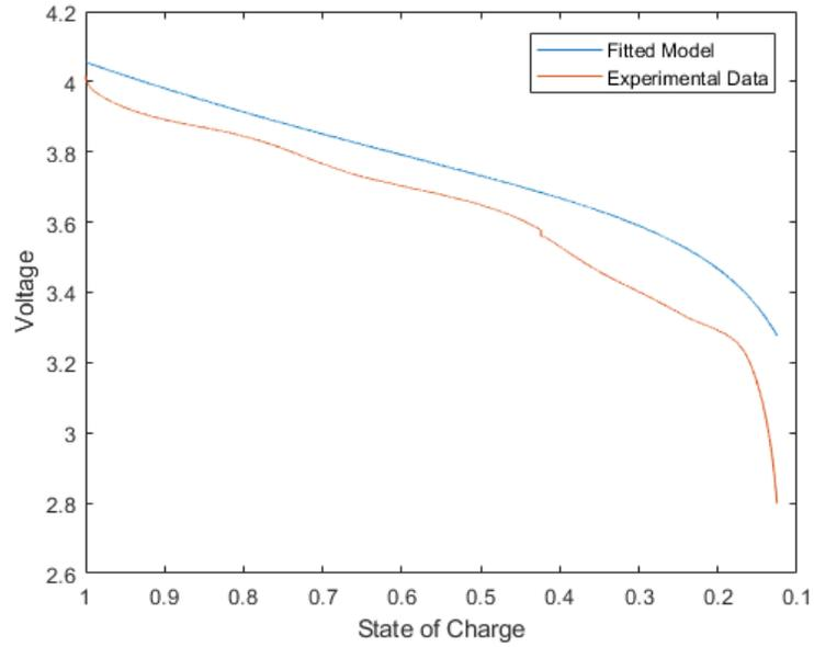
**Figure 2.29:** Prediction of 0.9 A discharge with parameters of 1.50 A
