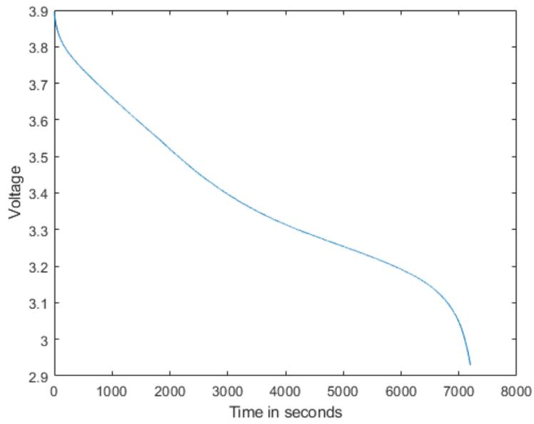
**Figure 3.2:** 0.50 A discharge of the 1000 mAh battery
