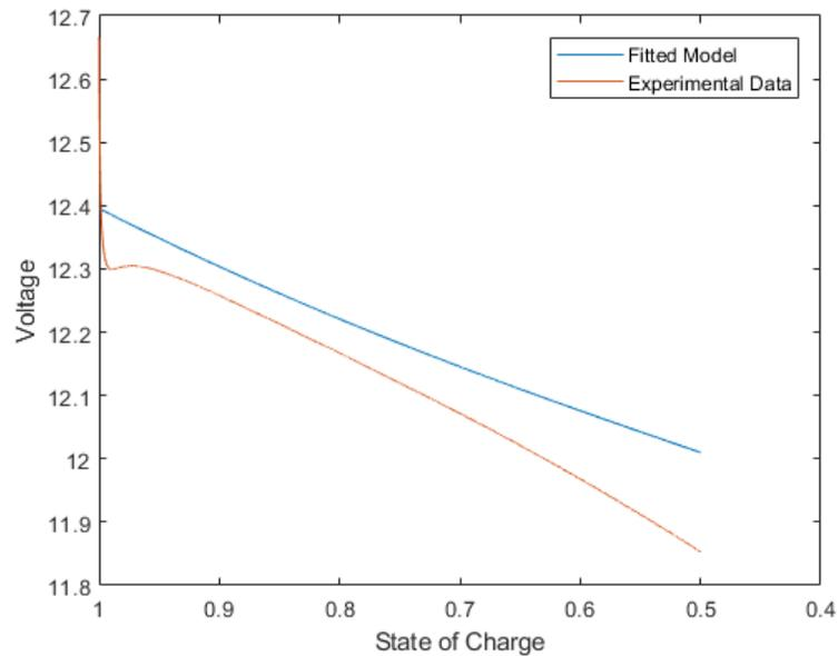
**Figure 2.31:** Prediction of 5.0 A discharge with parameters of 10.0 A
