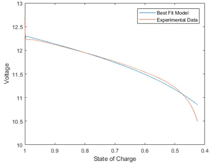
**Figure 2.11:** Identification of Lead battery at 7.5 A discharge - Data Set 1
