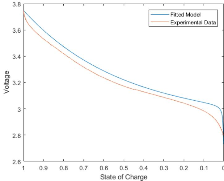
**Figure 3.11:** 0.5 A discharge parameters used to predict the discharge behaviour of 0.75 A discharge with  $E_a$  factor
