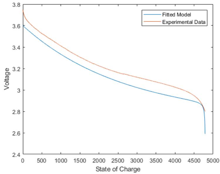
**Figure 2.19:** Prediction of 0.75 A discharge with parameters of 0.5 A
