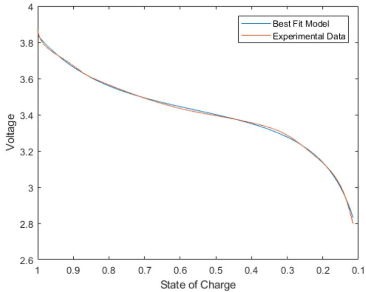
**Figure 2.3:** Identification of 400mAh Lithium-ion battery at 0.4 A discharge - Data Set 1
