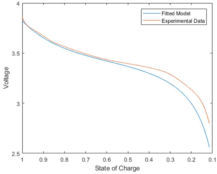
**Figure 2.14:** Prediction of 0.4 A discharge with parameters of 0.2 A
