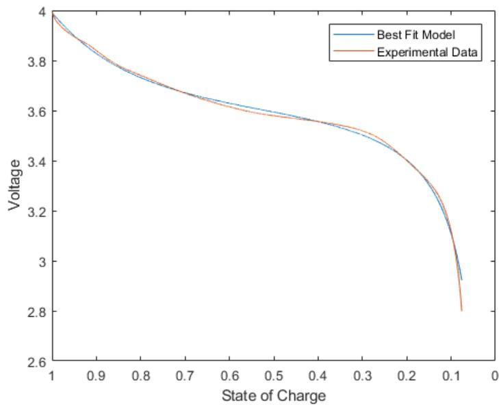
**Figure 2.1:** Identification of 400mAh Lithium-ion battery at 0.2 A discharge - Data Set 1
