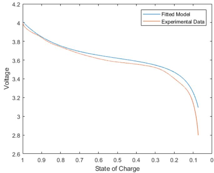
**Figure 2.15:** Prediction of 0.2 A discharge with parameters of 0.3 A
