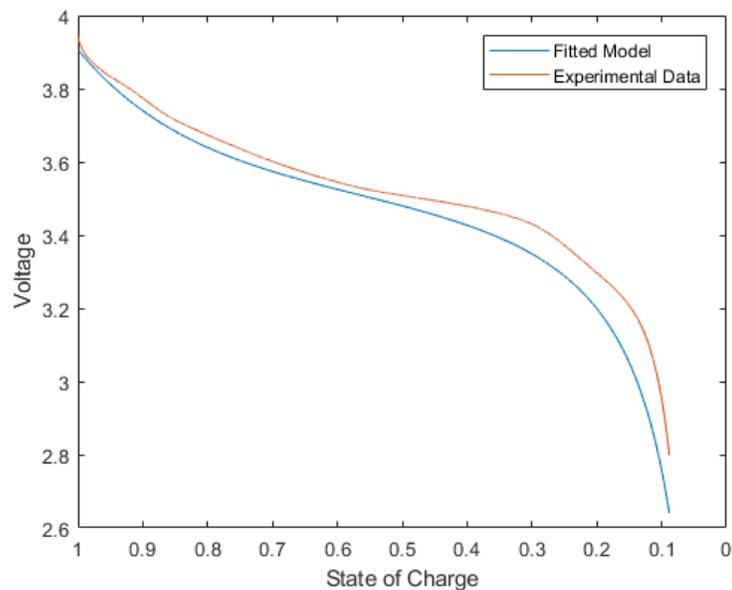
**Figure 2.13:** Prediction of 0.3 A discharge with parameters of 0.2 A
