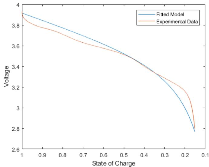
**Figure 2.26:** Prediction of 1.50 A discharge with parameters of 0.9 A
