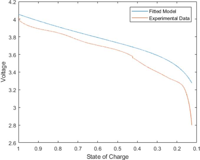
**Figure 3.8:** Prediction of 0.9 A discharge using 1.5 A discharge parameters
