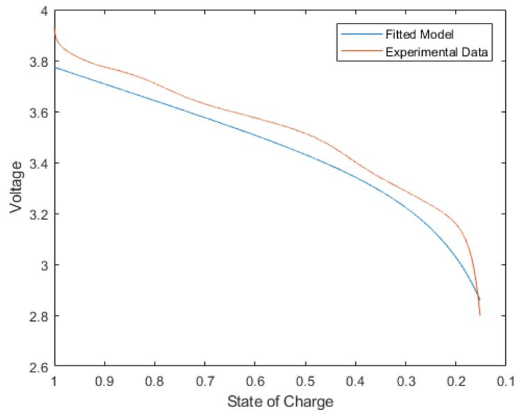
**Figure 2.28:** Prediction of 1.50 A discharge with parameters of 1.20 A
