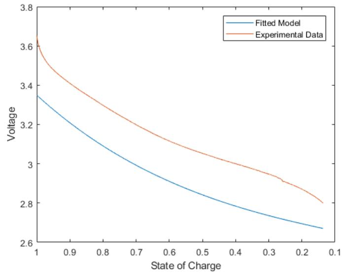
**Figure 2.20:** Prediction of 1.0 A discharge with parameters of 0.5 A
