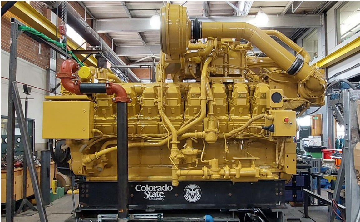
Figure 24: Photo of Colorado State University Engines Energy Conversion Laboratory Caterpillar G3516J natural gas engine.
