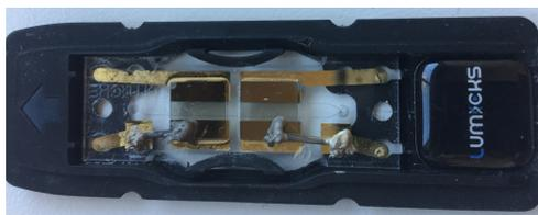
Figure 1.4: AFS Acoustic Force Spectroscopy flow cell chip: There are two pairs of piezoelectric component with separate controls, one flow channel with inlet and outlet to do the experiment. Samples are bound on the surface of this channel.
