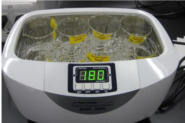
Fig. G.3. Ultrasonic bath containing tooth samples inside beakers of KOH.
