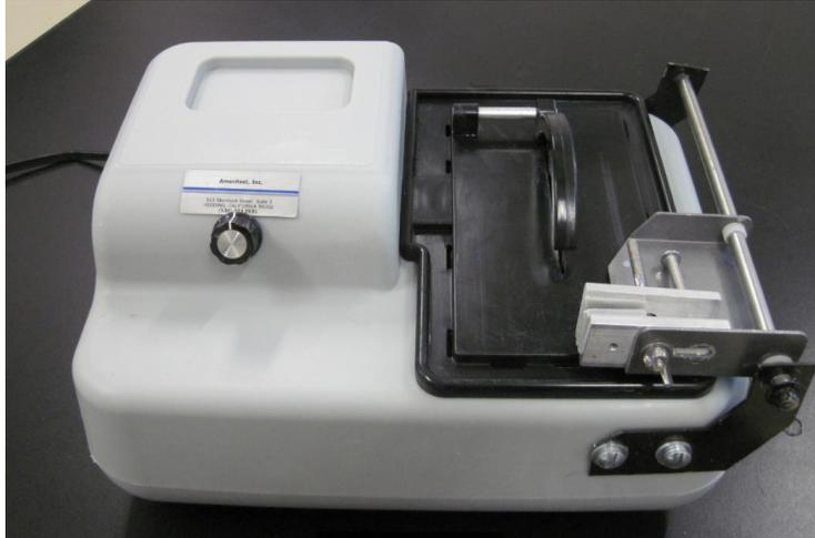
Fig. B.1. Saw used to perform crown amputations.
