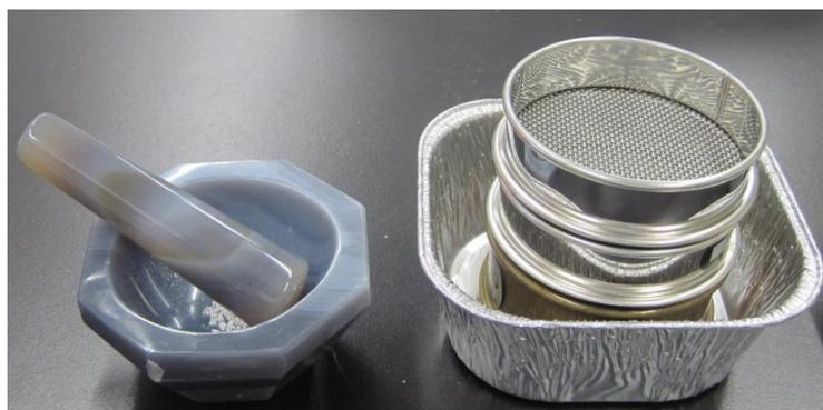
Fig. G.7. Mortar and pestle used to grind enamel into a powder for measurement in an EPR spectrometer alongside sieves used to ensure desired particle sizes are obtained.
