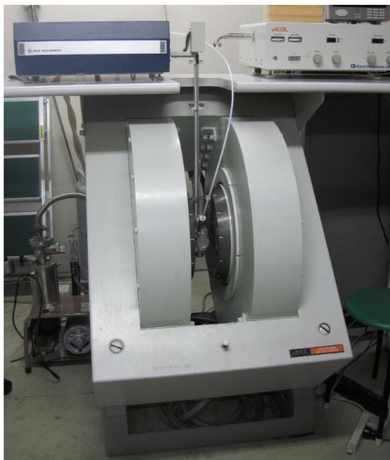
Fig. 2.3. JEOL JES-PX2300 ESR Spectrometer.
