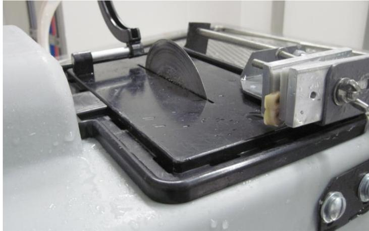
Fig. G.2. Boar tooth in position to be cut into smaller pieces.
