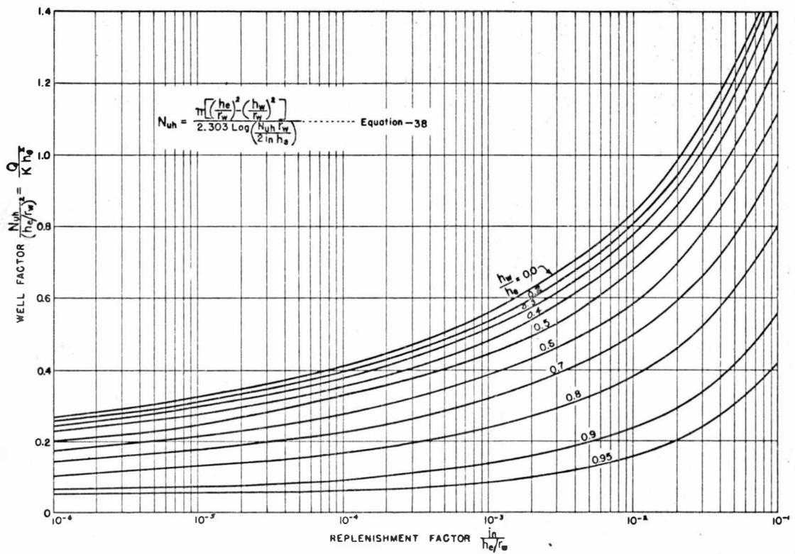
Fig. 5. Horizontally-recharged well in unconfined system
