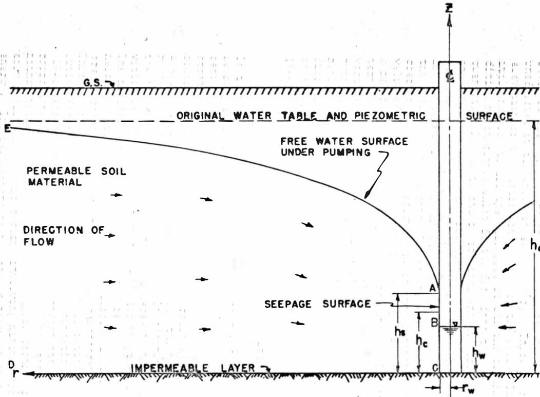
Fig. 2. Flow of unconfined ground water to a well in permeable soils overlying impermeable material
