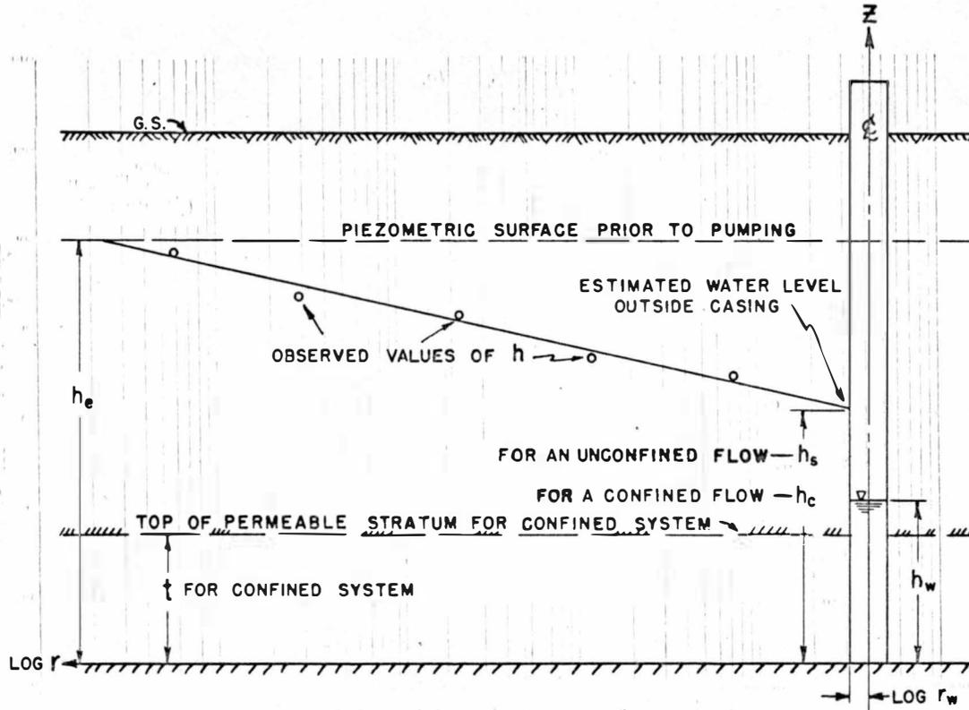
Fig. 9. Illustrating the method of estimating the water level outside a well for both confined and unconfined systems
