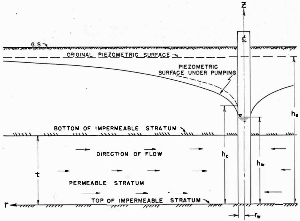
Fig. 1. Flow of confined ground water to a well
