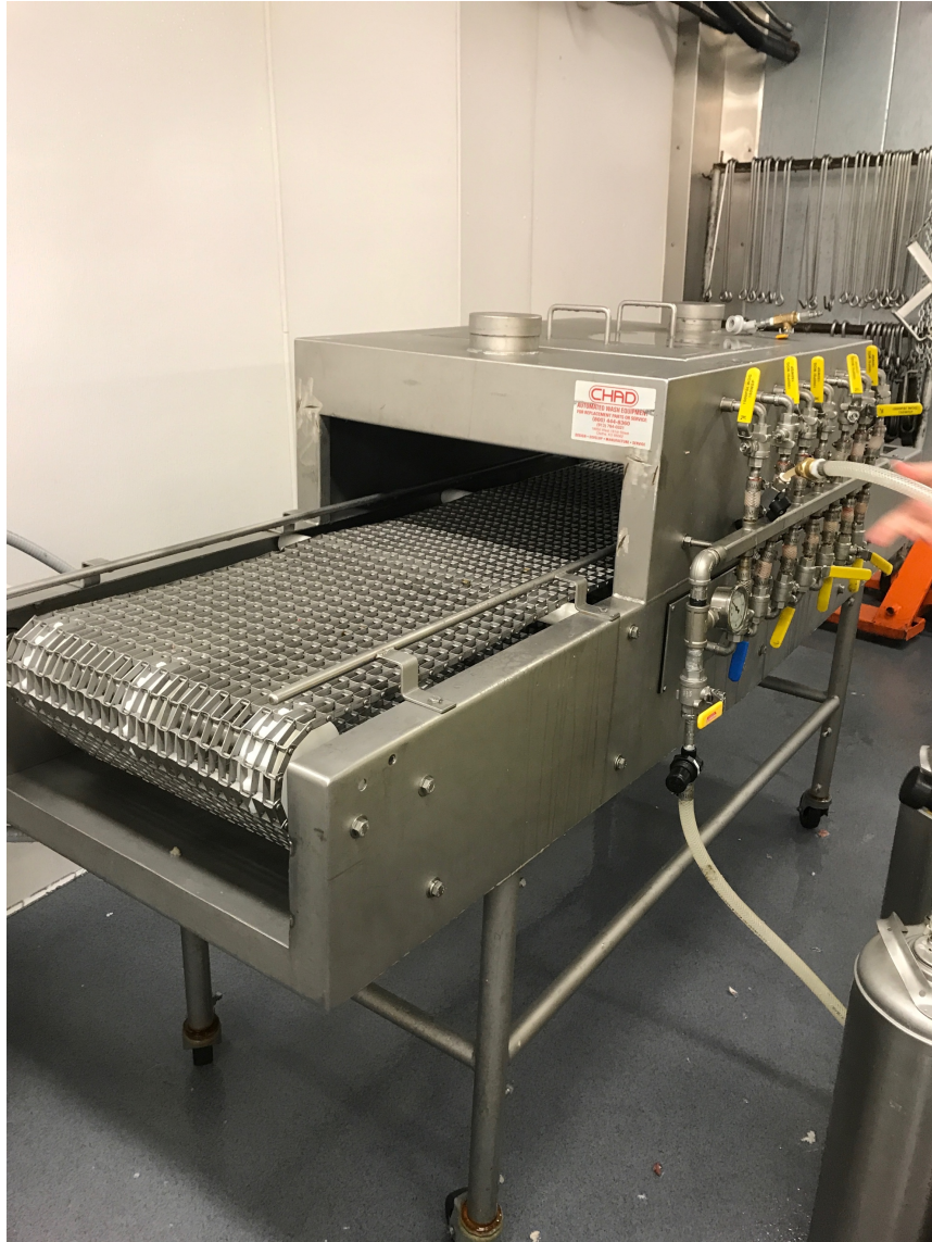
FIGURE 4. 1. Custom-built, pilot-sized spray cabinet designed to simulate a commercial beef spray cabinet.
