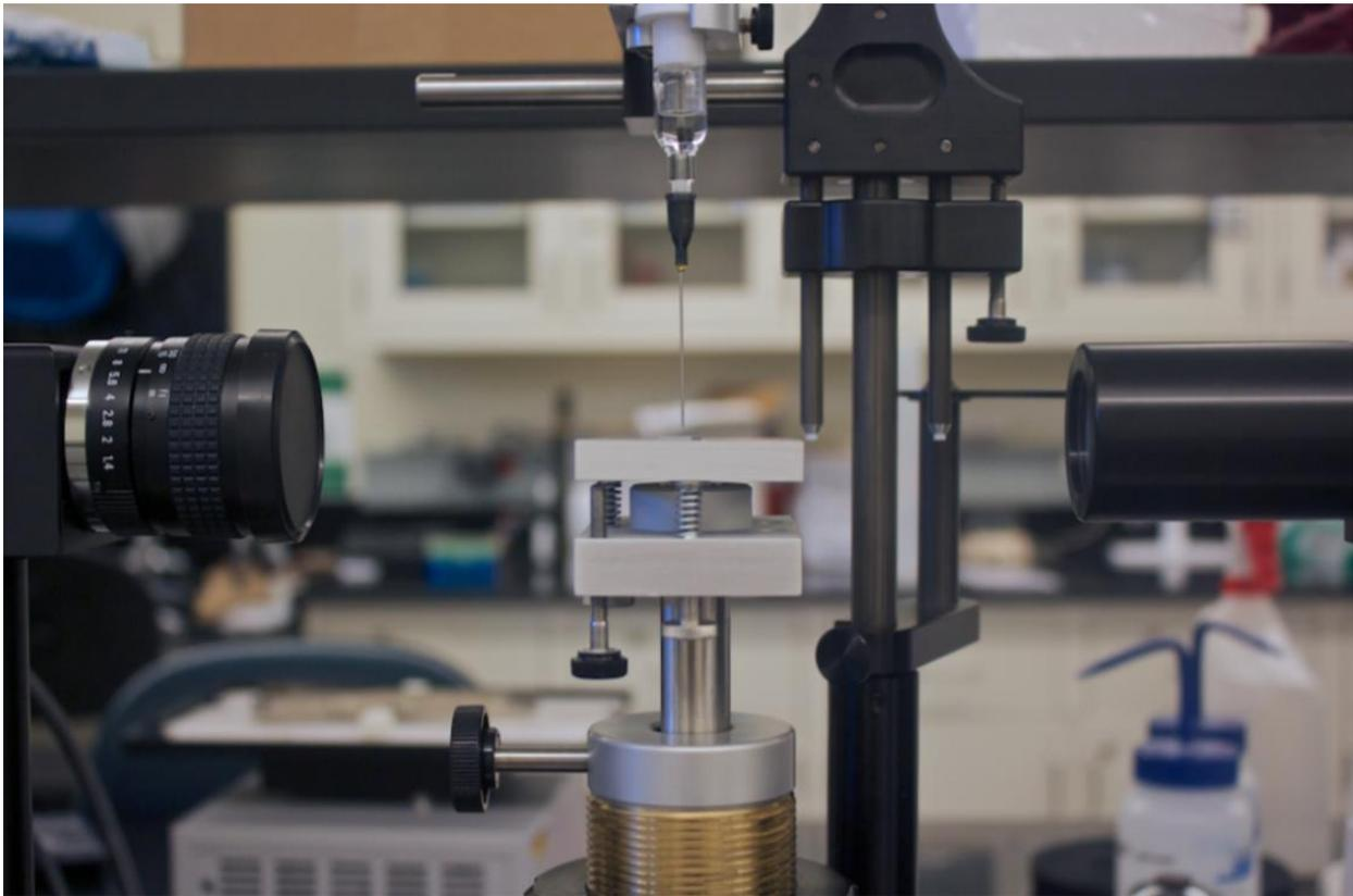
**Figure 2.3.1:** ramé-hart Model 250 Standard Goniometer used to obtain contact angle measurements.
