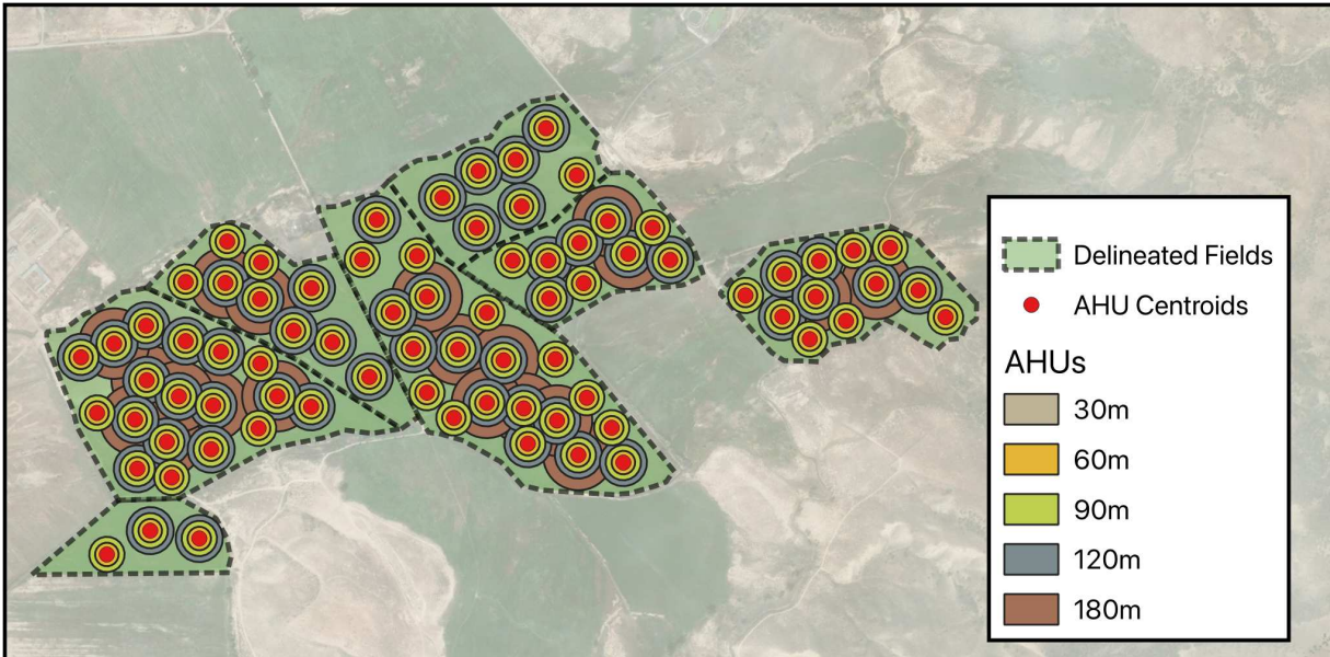
FIGURE 3.3. Nested orientation of AHUs with varying diameters randomly placed within fields that participated in water conservation activities in at least one year in the 2018-2024 period.
