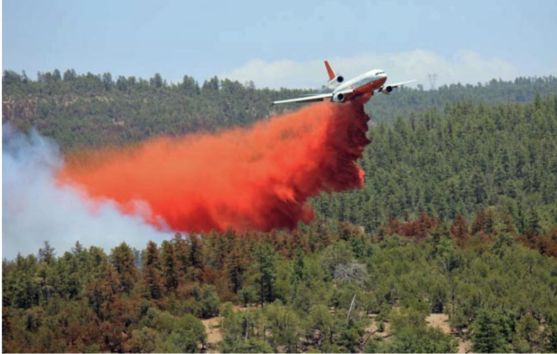
Figure 4.1: Large airtanker (LAT) delivering a load of fire retardant ahead of an advancing flame front. Photo by Ian James, courtesy of Wildfire Today .
