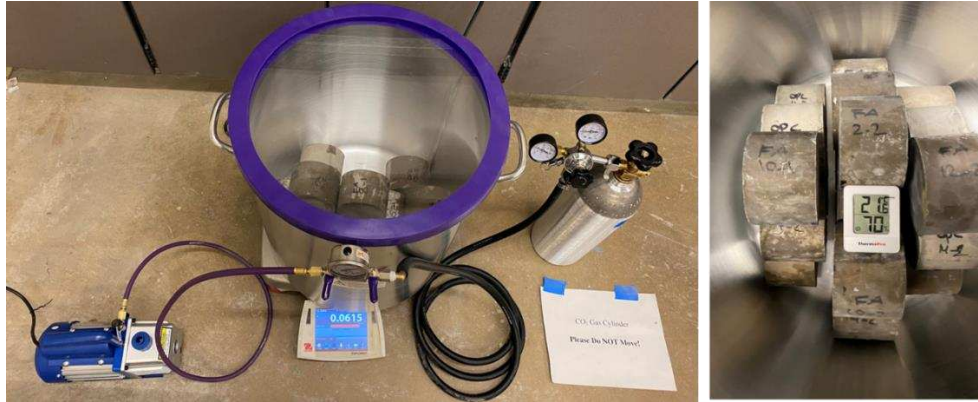
Figure 3.16. Exposure to carbon dioxide (carbonation test)
