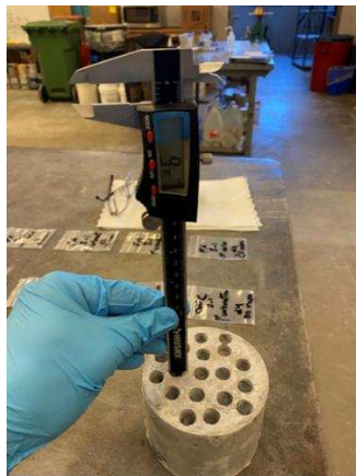
Figure 3.17. Taking powder from four depths of carbonated paste (colors represent depths)
