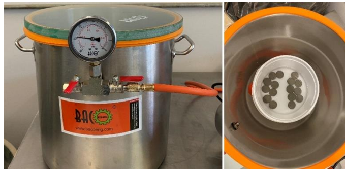
Figure 3.3. The experimental setup used for saturating disk samples
